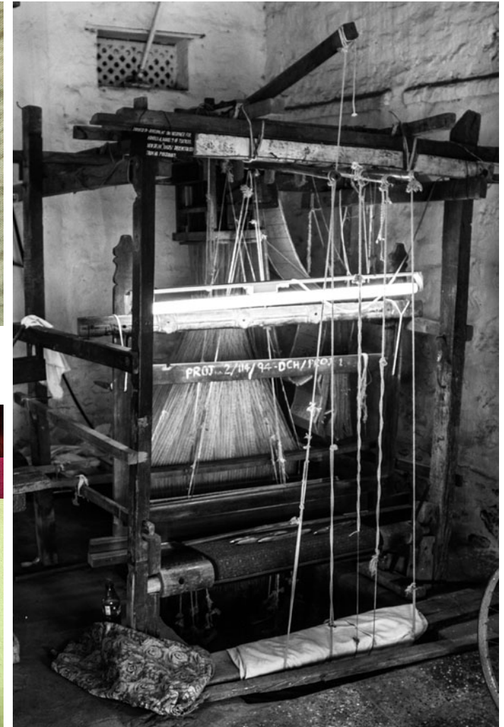
Traditional Loom is used for weaving Himroo.
