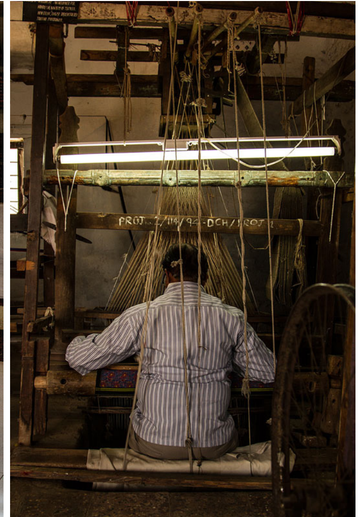
Traditional jacquard loom is used to weave Himroo.
