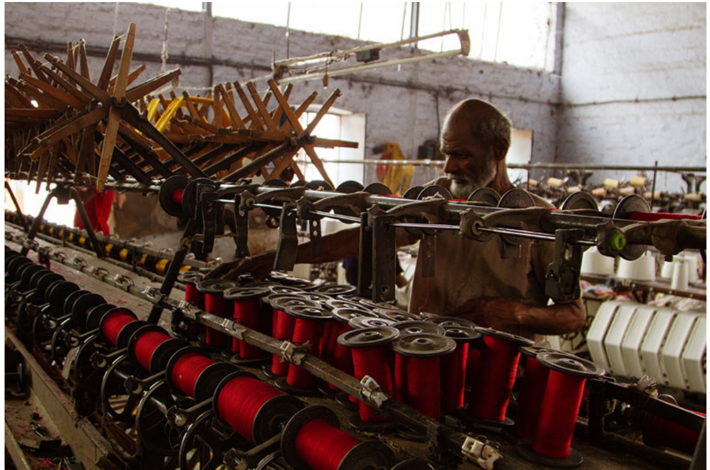
The yarns are converted into spools using reeling machine.
