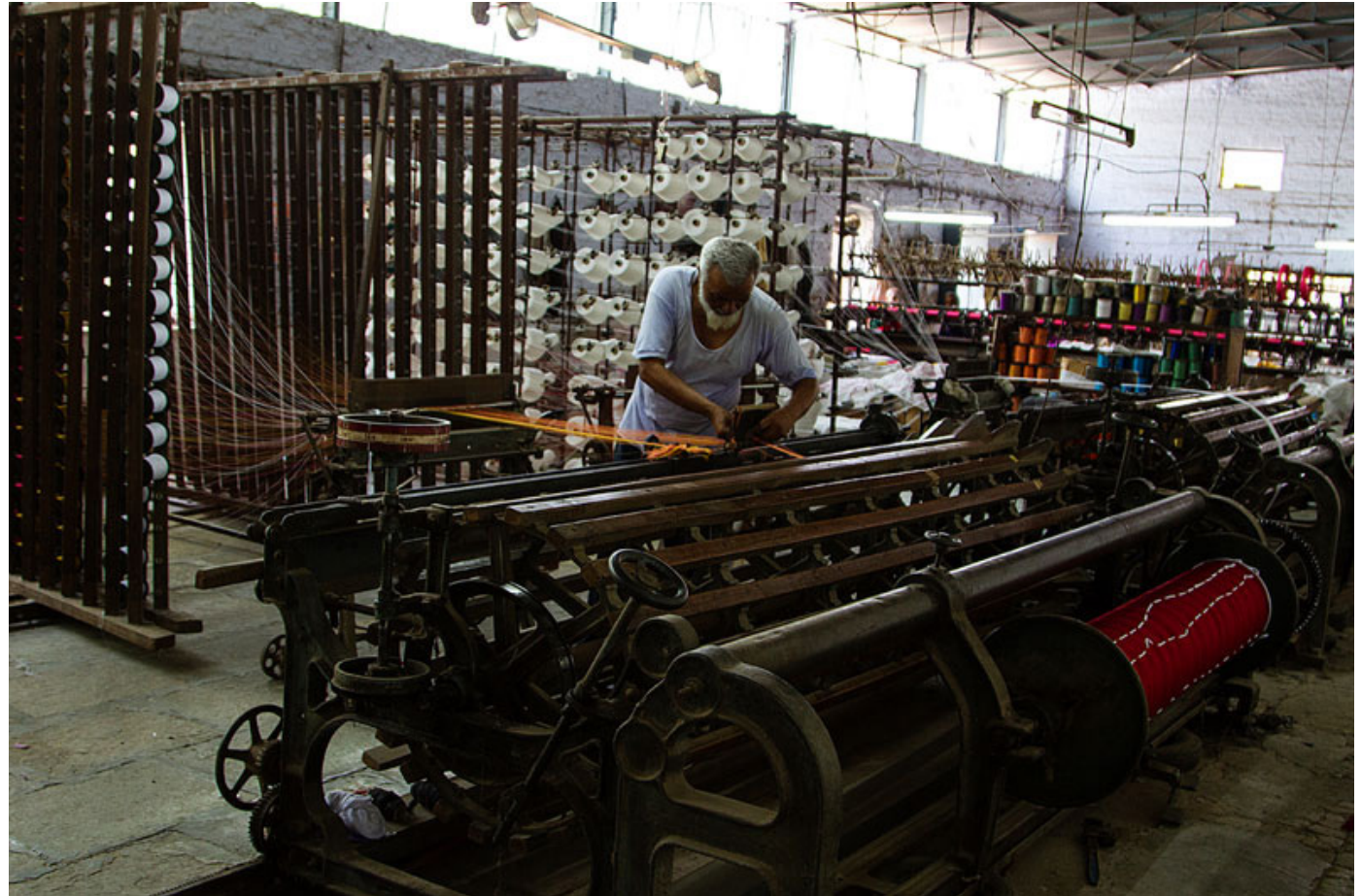
Threads are wound on the beam.
