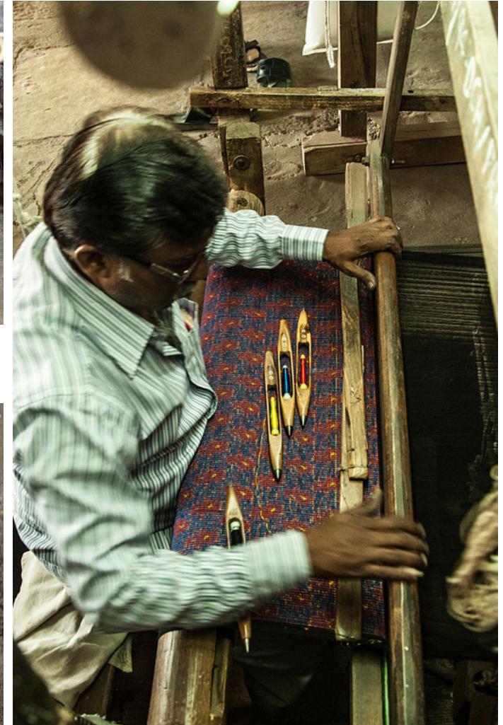
Spindles are inserted in the fly shuttle, which is passed through layers of yarns to weave pattern.
