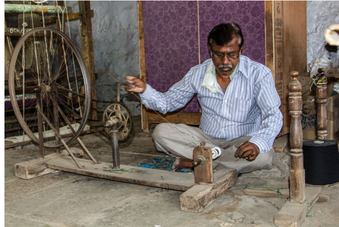
Charkha is used to make spindles for the fly shuttle.
