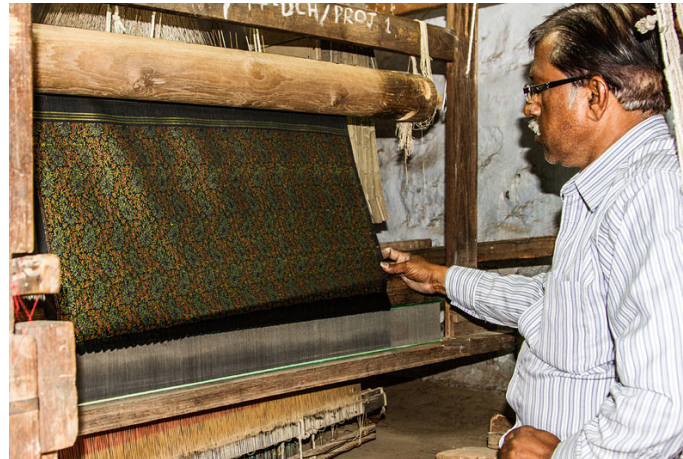
The front side of the himroo shawl is faced down while weaving.
