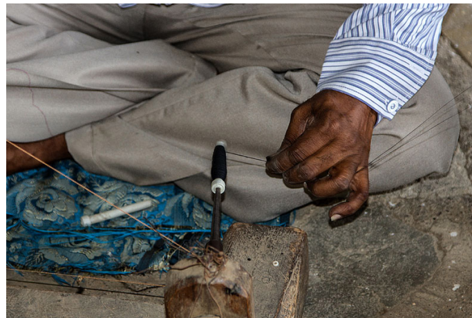
Plastic pin is attached to the charkha and the thread is wound on the pin to make spindles.
