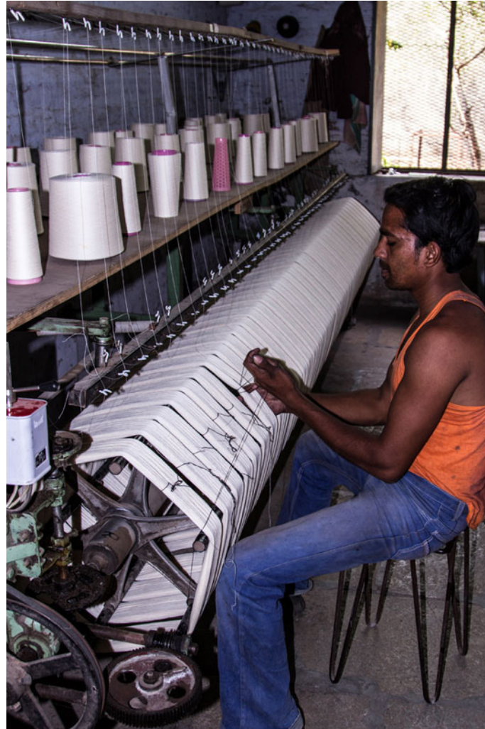
Cotton and silk threads are converted into spools and spun into yarns.
