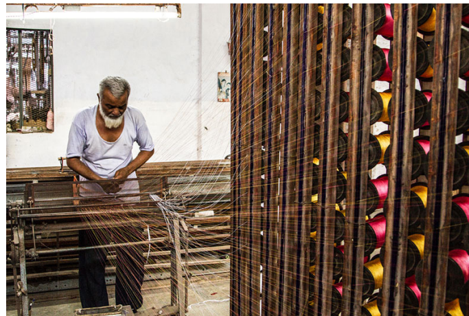
The spools are attached to the creel and connected to the warping machine.
