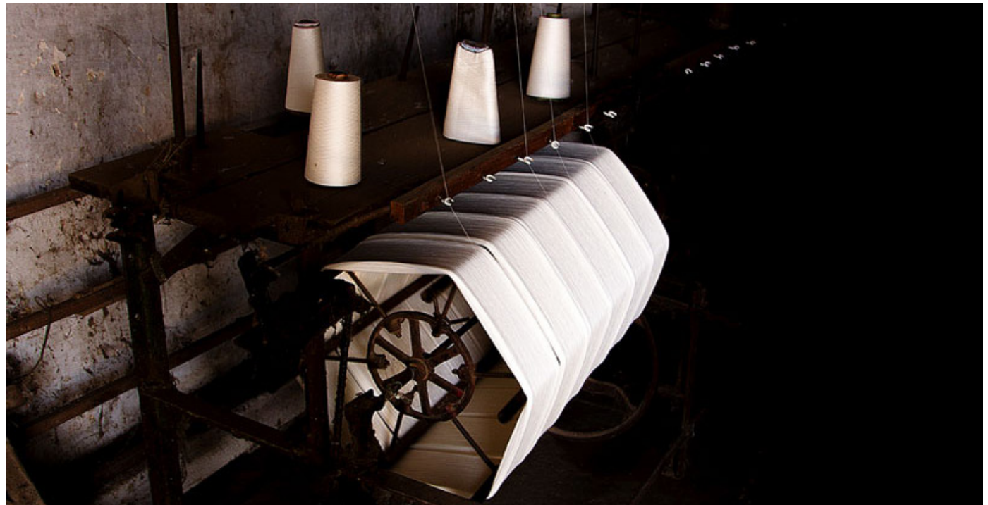
Yarns from cones are wound to hank with the help of winding equipment.
