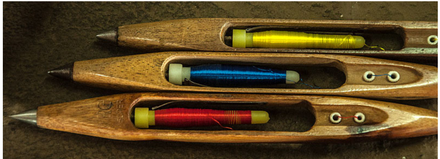
Different colors of spindles inserted in the fly shuttle.
