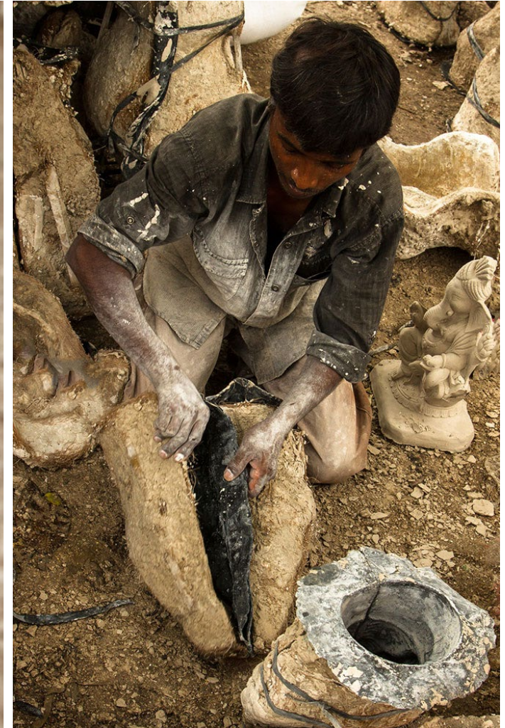
Rubber mold is placed between PoP molds.
