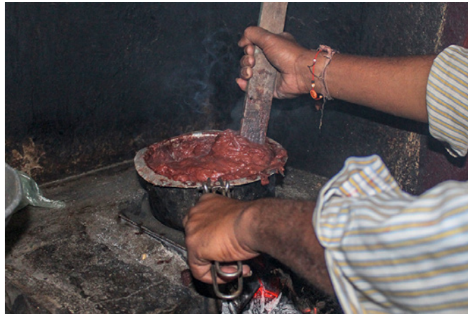
Tamarind seed powder, water and natural adhesive are mixed with hot boiling water.
