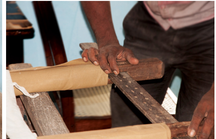
A wooden bar, passing through the hole to form a rectangular frame.
