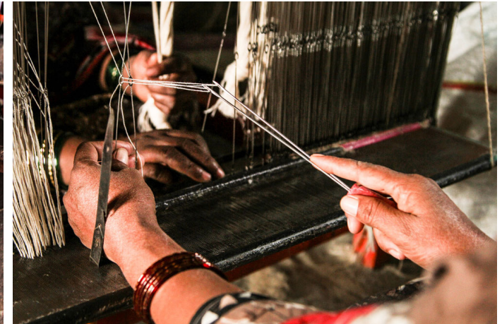
Threads are pulled through the loop of the heddle wire.
