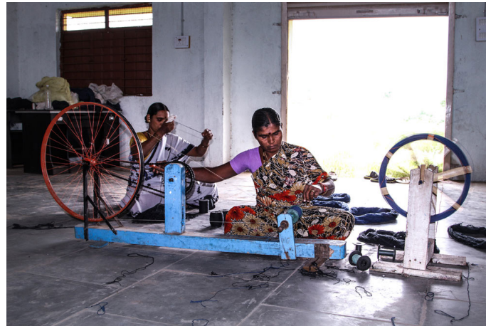
Wooden wheel is then attached to the charkha to make spools of the yarn.
