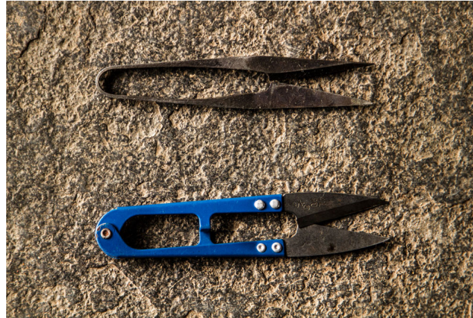
Cutters are used to cut out the excess threads.
