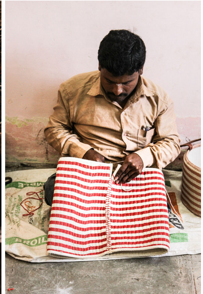
Fabric is cut into required size and joined together to form a cylindrical basket, and the ends are joined by sewing manually.
