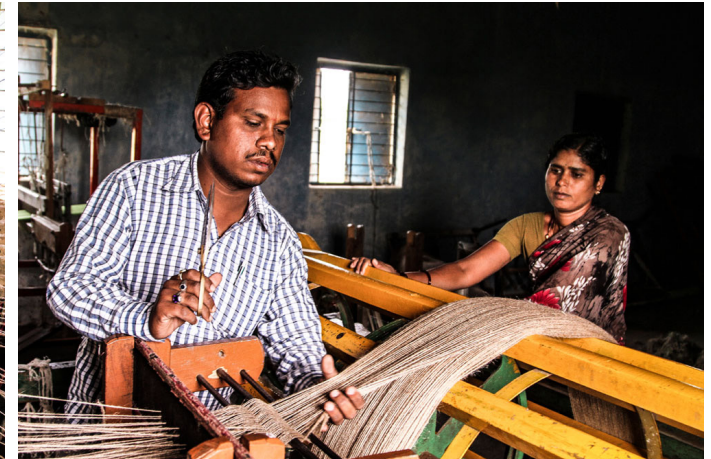
Warping process is done to remove the tangles and strengthen the quality of the thread.
