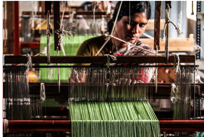
After the drawing process warp beam is fixed to the weaving loom and weaving of the fabric is started.
