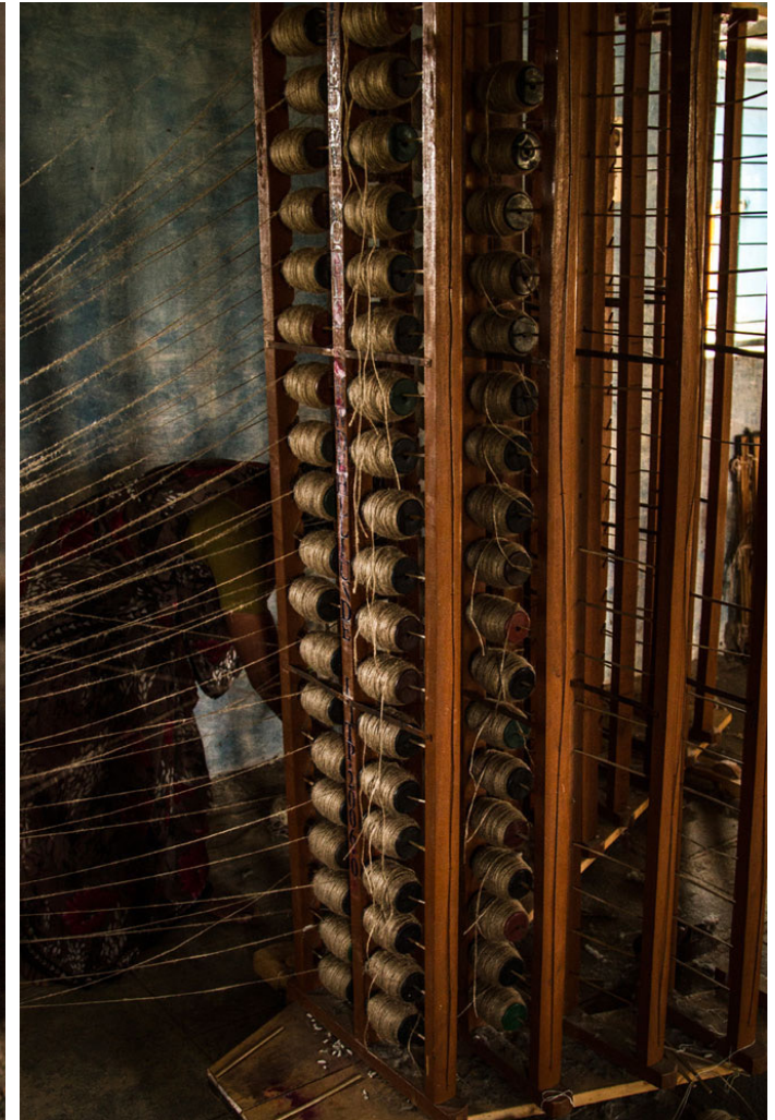
Wooden frame are used to hold the spool in the warping process.
