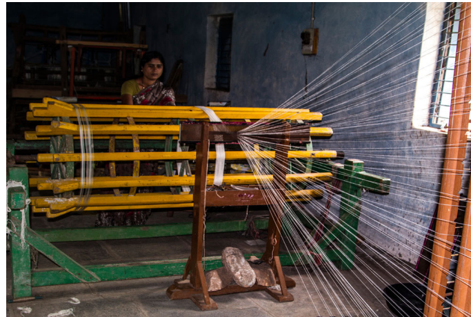
Warped threads are spun on the warping wheel.
