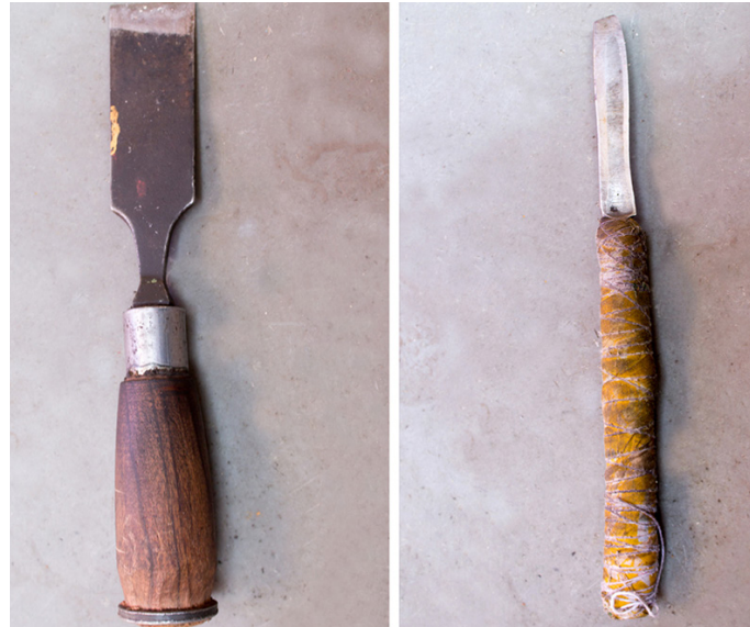
Varies chisels are used to craving wooden surface.
