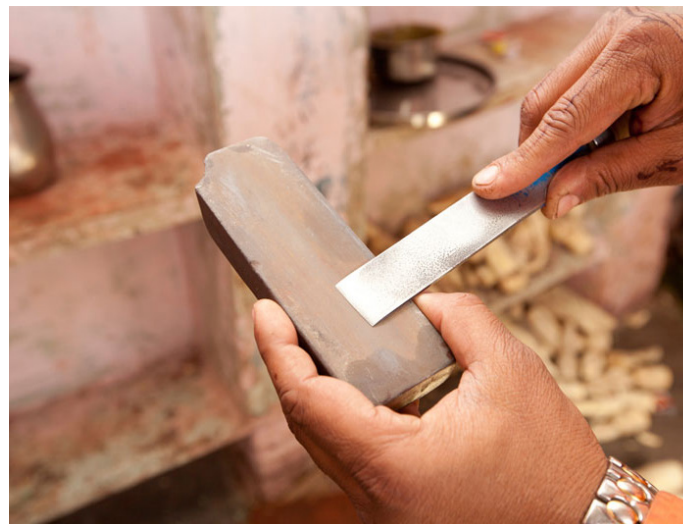
Whet stone or sharpening stone is used to sharpen the chisels.
