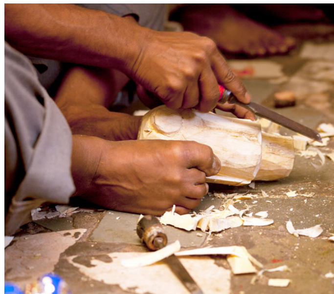
Scraping is done to make the log surface even.
