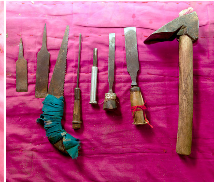
Various tools are used to shape a Kathputli. Small hand saw is used to cut the wood and small chisels for detailed carving.
