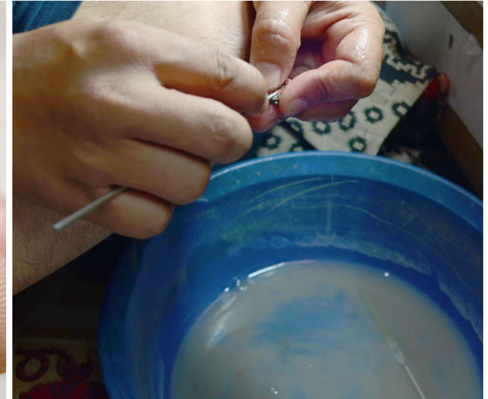
The jewelry piece being scrubbed with a filer to enhance the gold outline of the pattern.
