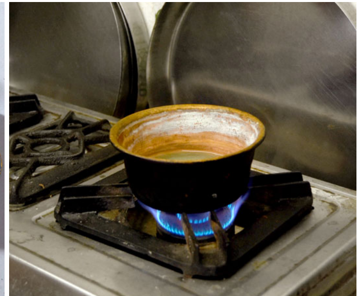
The piece being boiled with mild acid for sheen.
