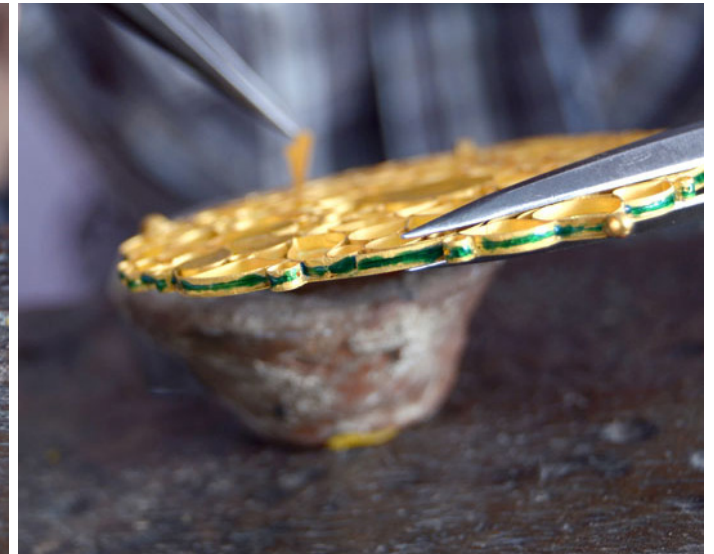
Lac being heated and poured into the creeks, which are supposed to hold the gems.
