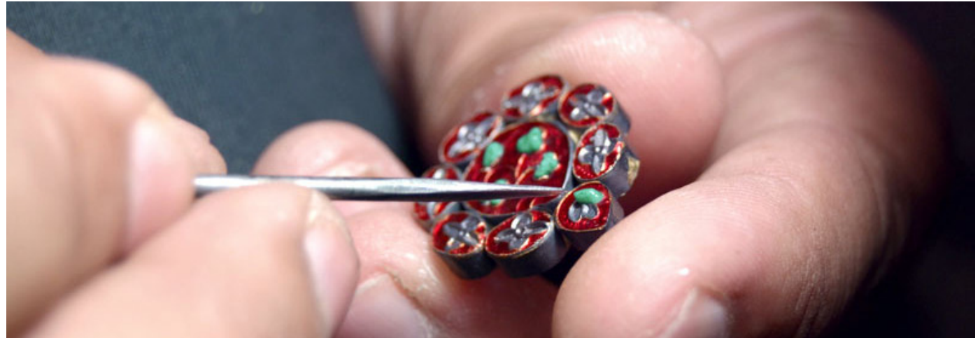
Color being applied with thin spoke in the engraved pattern.
