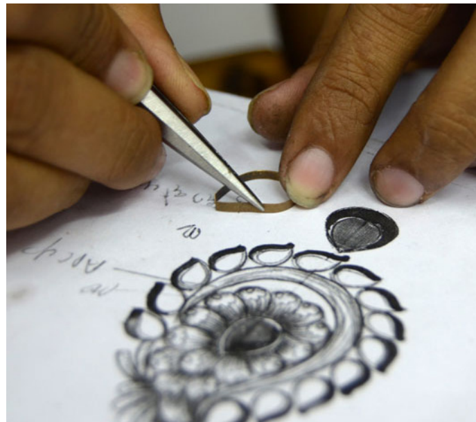
Gold strip being shaped according to the design.
