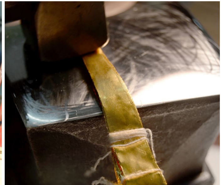
24 carat gold foil being made soft and malleable by hammering.
