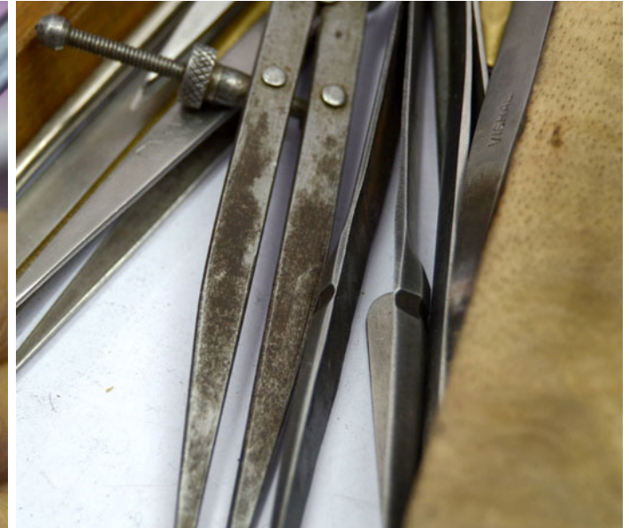
Fine tools and tweezers to shape the gold strips.
