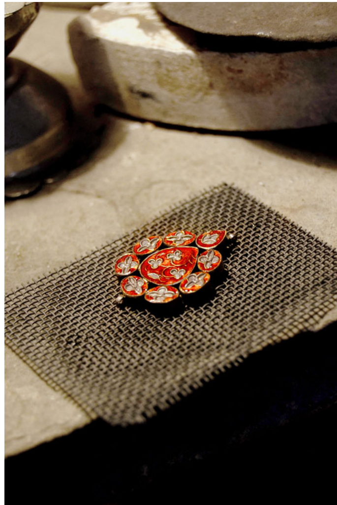
The piece kept on an iron mesh after the first firing.
