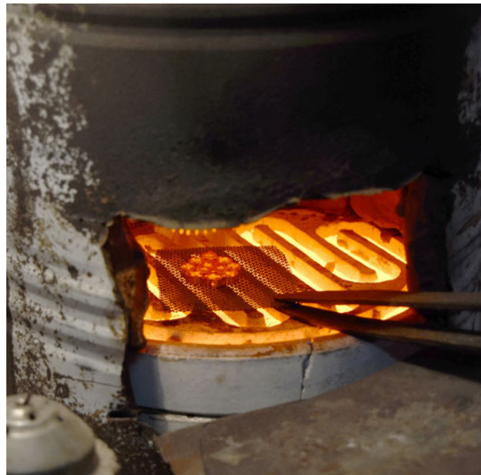
The piece being fired on the coils of the domestic heater.
