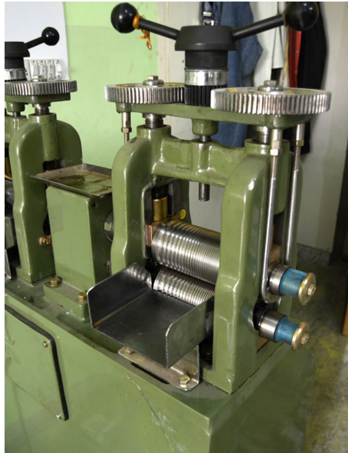
Thin gold strips being prepared from a rolling machine.
