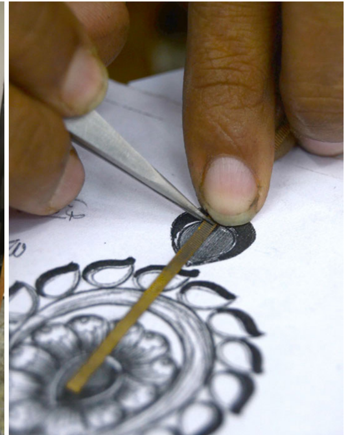
Gold strip being shaped according to the design.
