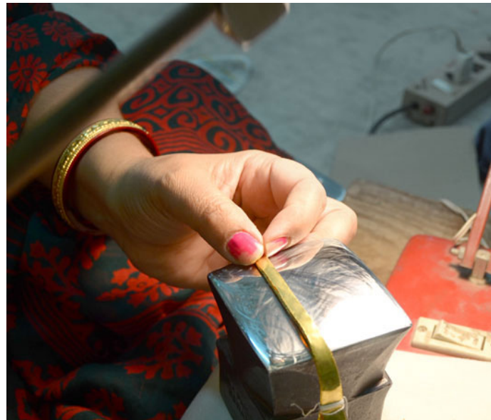
24 carat gold foil being made soft and malleable by hammering.
