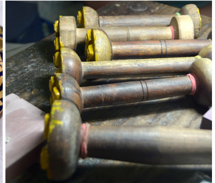
The dumbbells used for holding the jewelry piece in lac.
