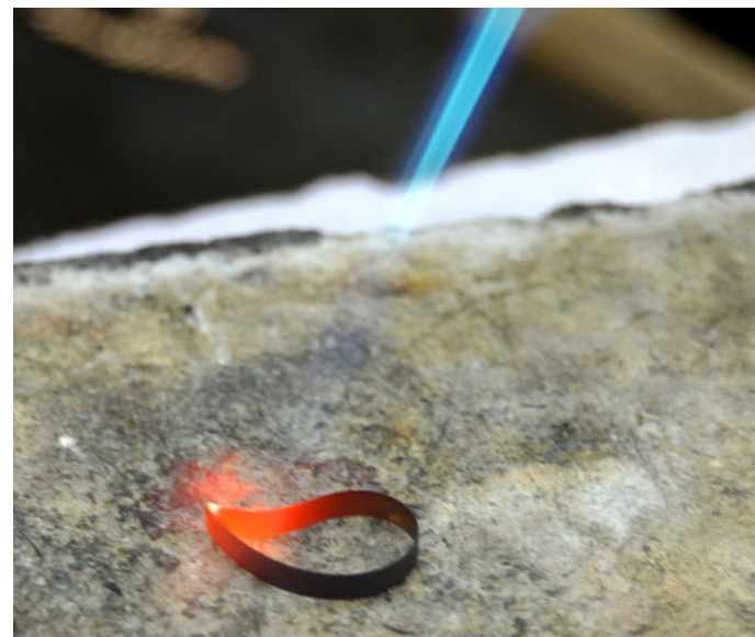
Gold strips being soldered together to form one solid piece.
