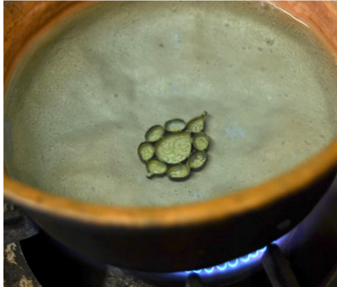
The piece being boiled with mild acid for sheen.
