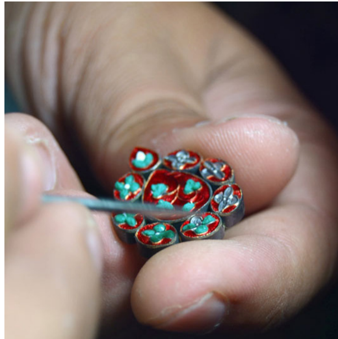
Color being applied with thin spoke in the engraved pattern.
