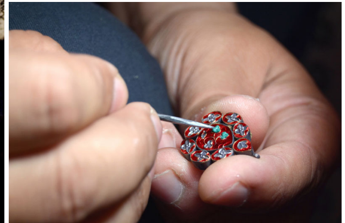
Color being applied with thin spoke in the engraved pattern.
