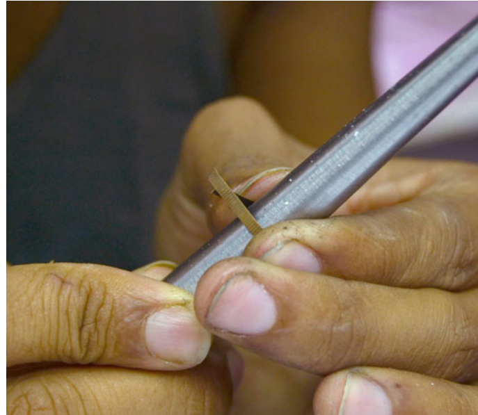
Gold strip being shaped according to the design.
