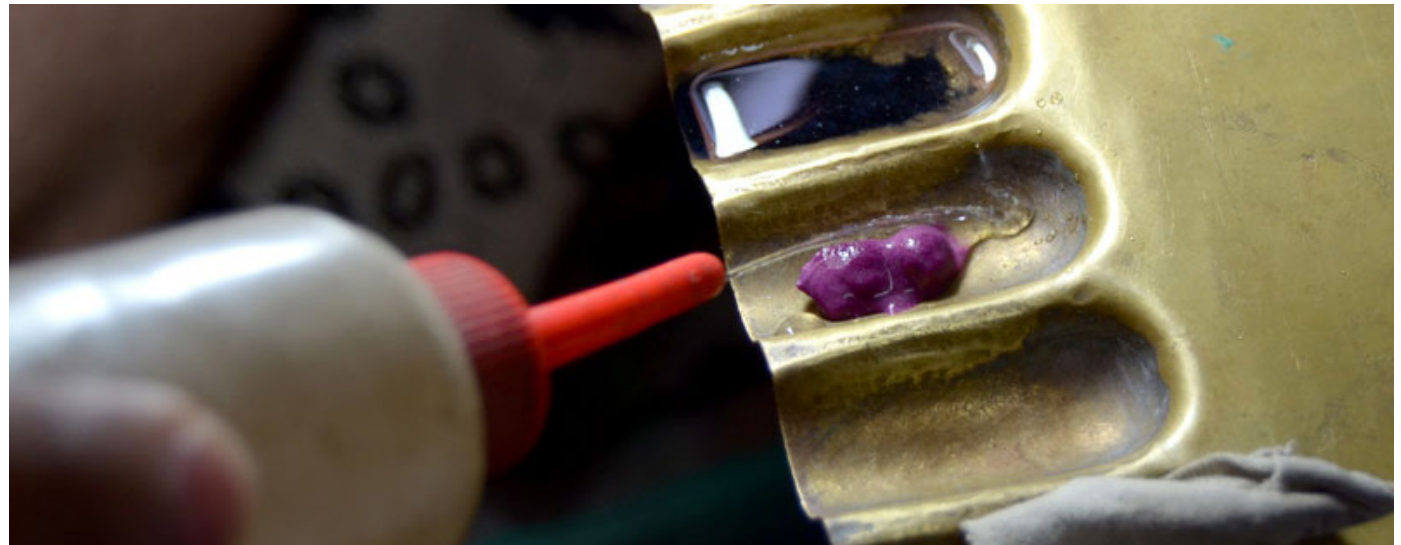
Enamel colors being mixed with water for use.
