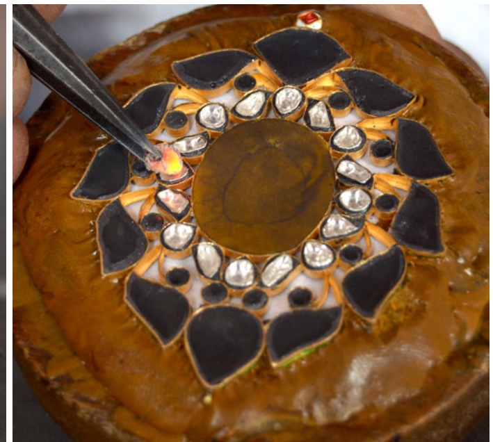
Stones being heated and placed on lac.
