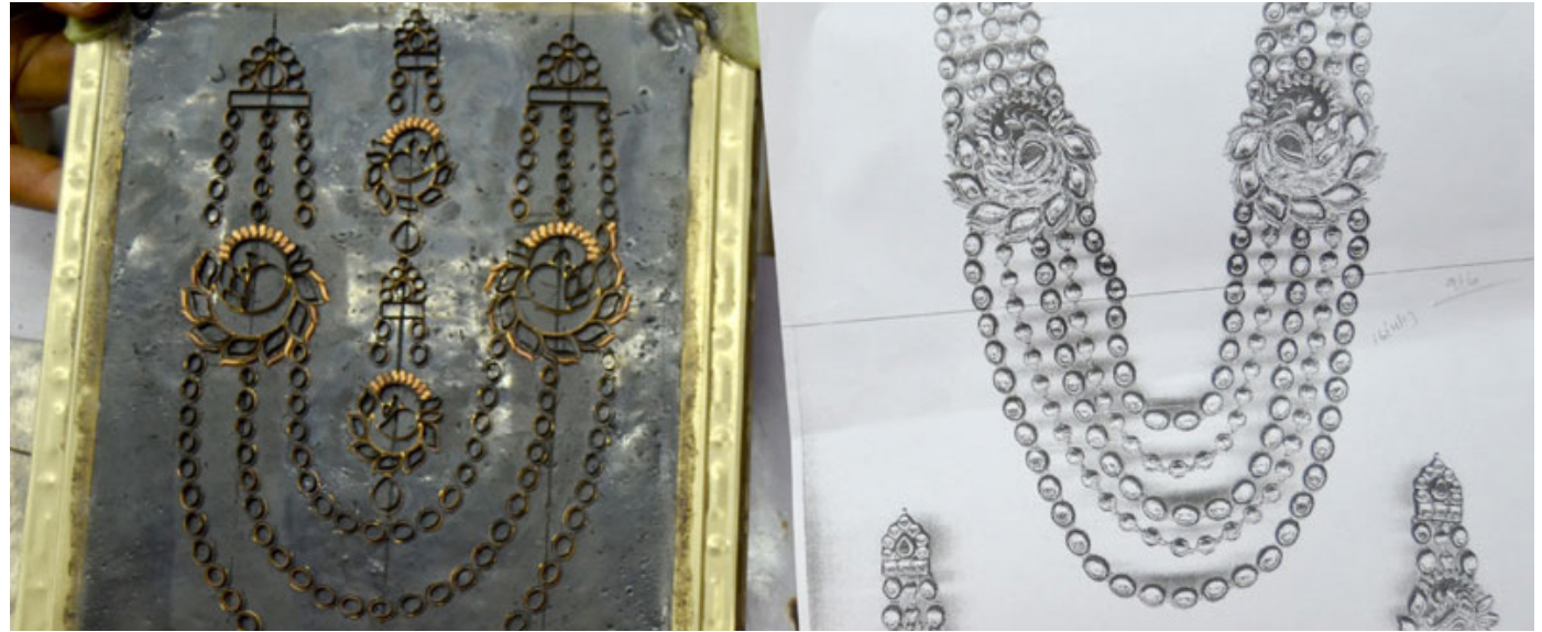
Soldered strips being set' on a wax board to exactly replicate the design.
