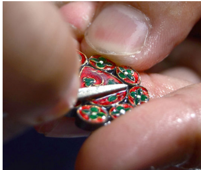
The jewelry piece being scrubbed with a filer to enhance the gold outline of the pattern.
