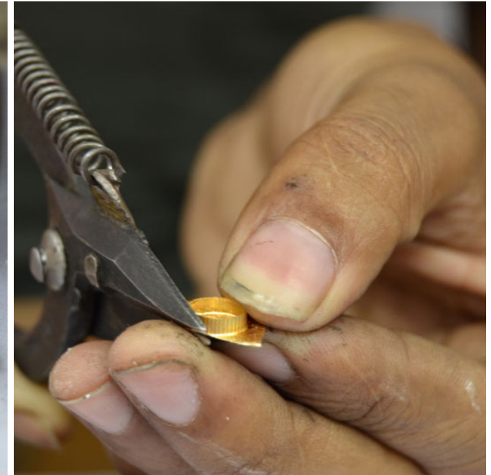
Soldered strips being finished.
