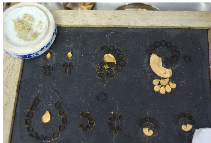
Soldered strips being set' on a wax board to exactly replicate the design.
