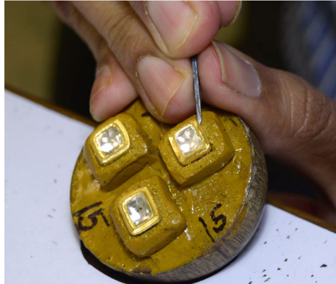
The foil being chiseled at an angle to bring out the fine details of the precious stones.
