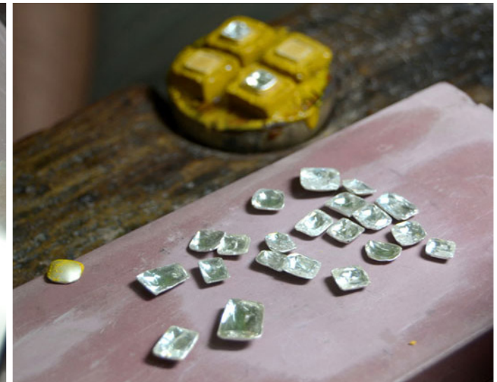
A piece of silver foil placed under the stones, making them gleam.
