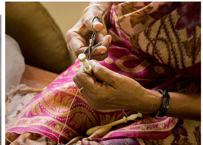
Rotating the thread to Bobbin with the help of Charaka machine, second photo cutting another string of wrapping around Bobbin.
