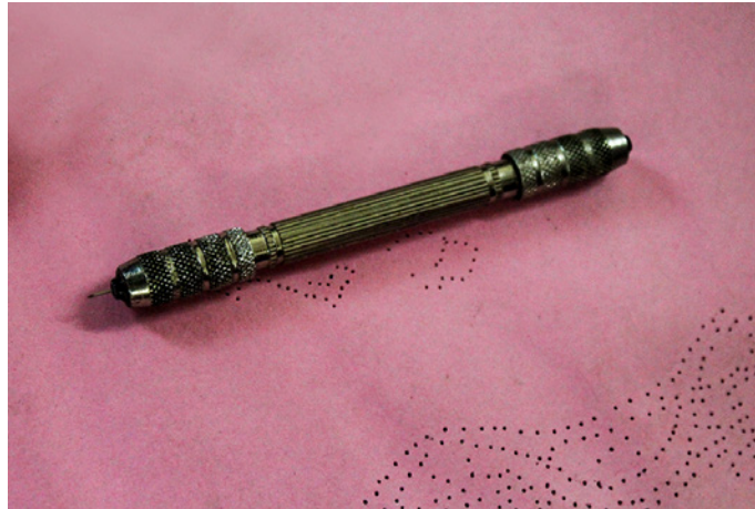
The piercing device used to remove artificial lace design mold.
