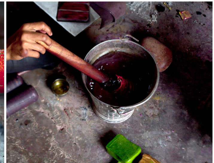
Water is used to cool the heated bangles before finishing.
