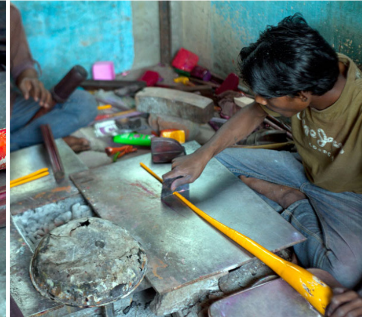
Thin coils are cut into pieces using a metal strip.
