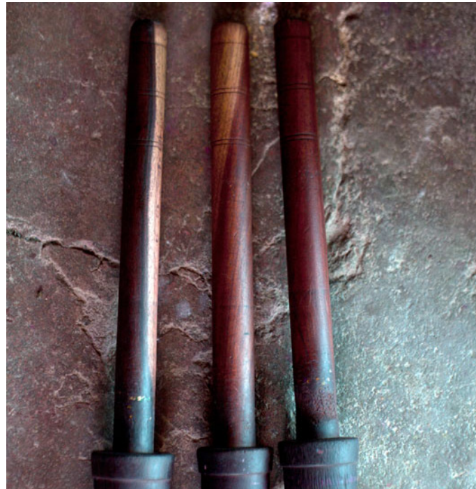
Round shaped wooden khali, used to size the bangles.
