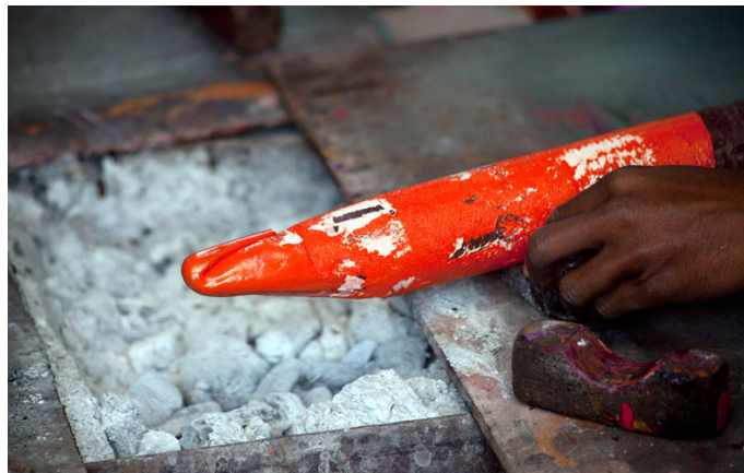
The colored lac is heated to make it soft.
