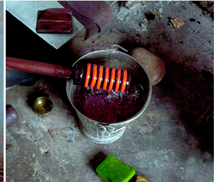
The shaped and sized bangles are dipped in water.
