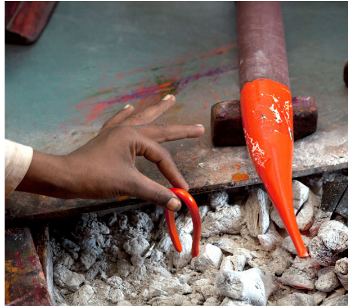
The coil is heated slightly to soften.
