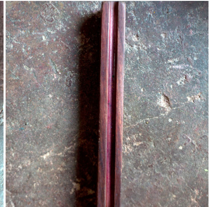
Farma, used to shape the bangle.
