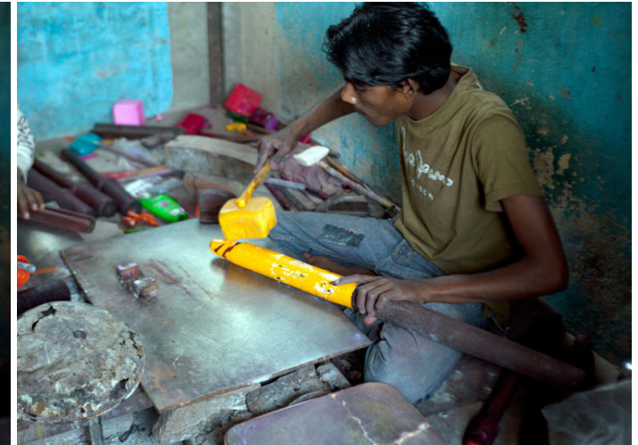
The required color is rubbed over the lac surface for detailed carving.
