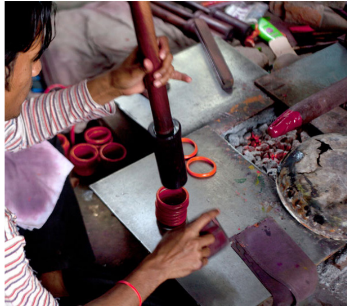
Removing the bangles for the wooden frame.
