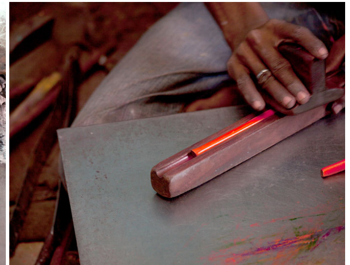
The coil is placed in the farma in order to give it a semi-circular shape.
