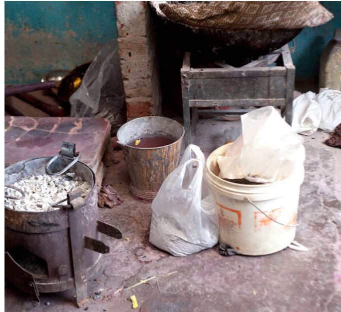
Iron stove is used to heat the bangles slightly during embellishing process.
