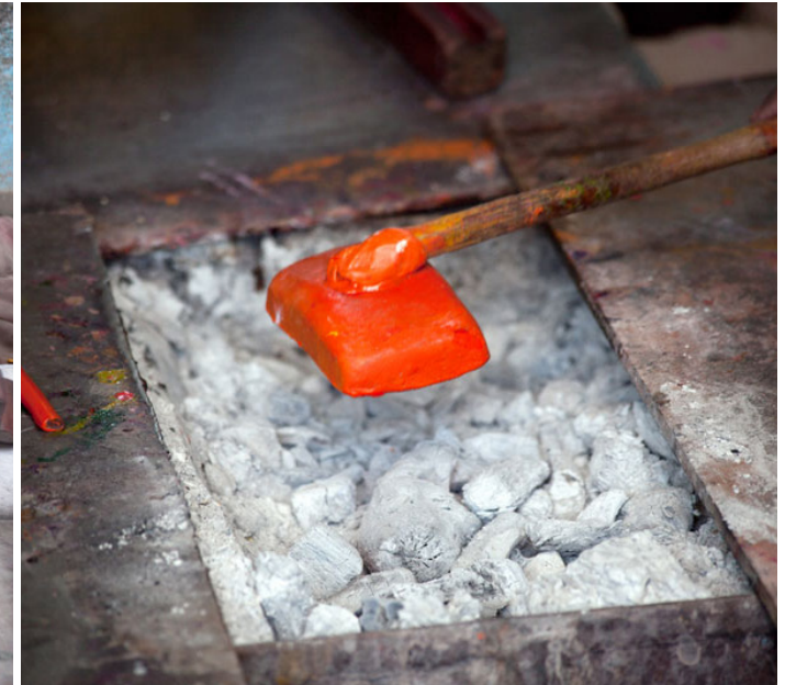
Lac is easily softened by heating.
