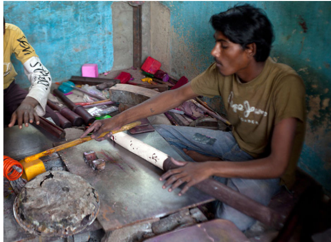
The base brown color lac is initially coated with white color.
