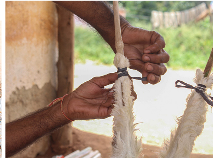
Again the fur is fixed tightly to the bamboo sticks and the sticks are covered.
