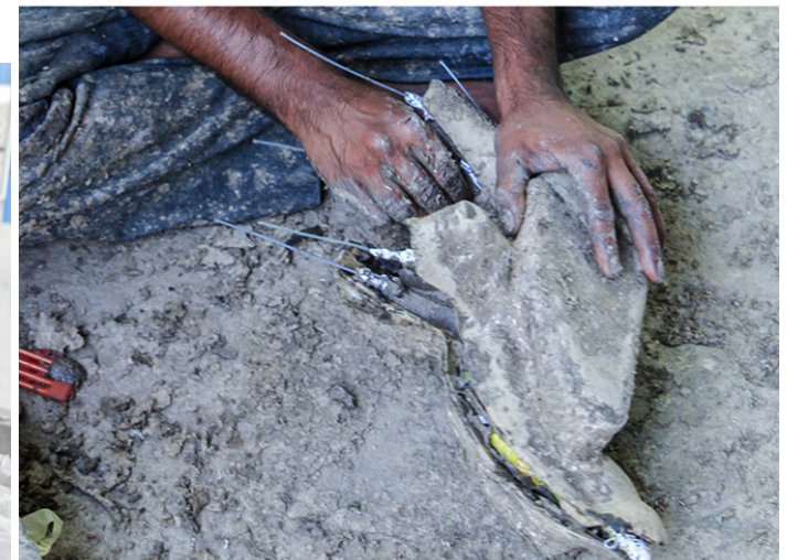
The paper clay is applied on toy by placing armature between molds.
