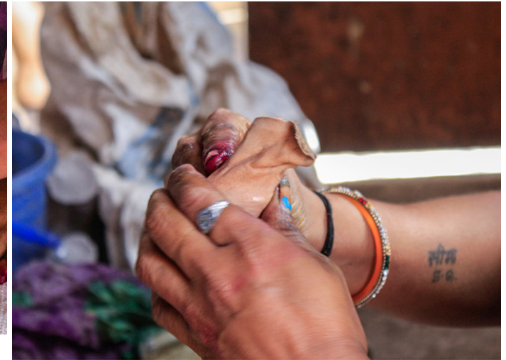
The leather is cut according to the shape of the toy.
