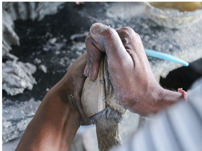
Face of the toy is made by placing molds near neck.
