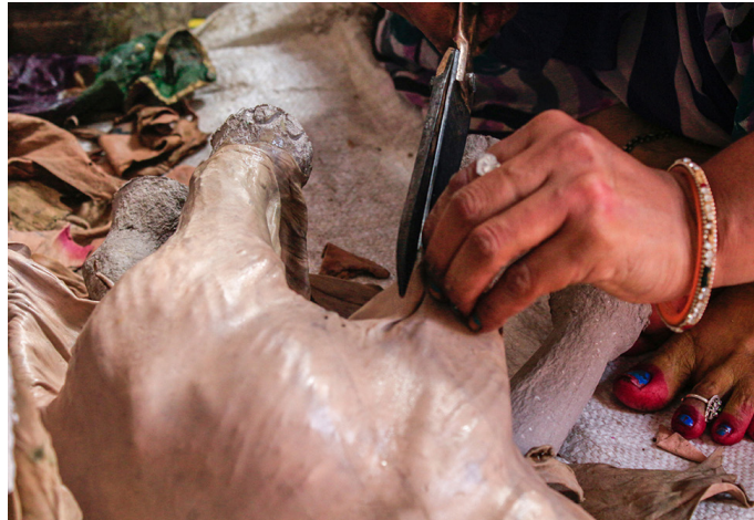
The leather is cut according to the shape of the toy.
