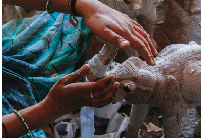
Toy is strengthen near the bends by pasting cotton cloth.
