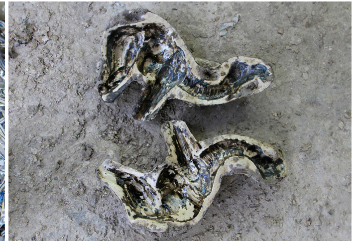
Stencil mold is used to apply paper clay on the toy.
