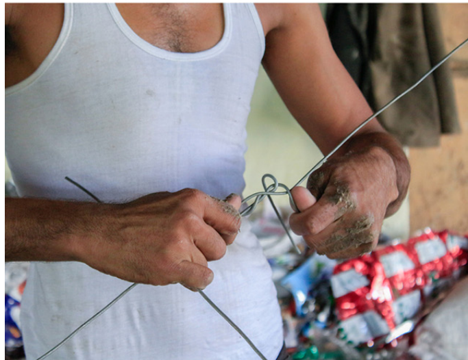
The skeleton of the toy is done using binding wire.
