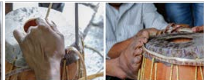
Two layers of buffalo Leather with a big hole is tied to the left side of resonator using rope.
