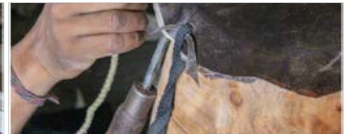
Holes are made on the leather to tie nylon strip.
