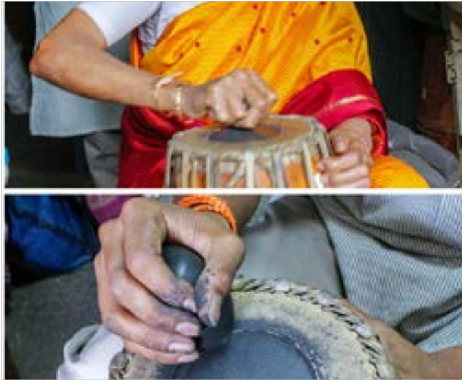
The karne (black patch) is leveled layer by layer using a stone.
