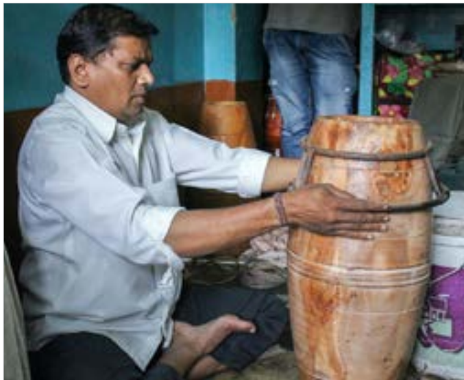
Iron frame of circular shape is placed on wood resonator to support the leather straps.
