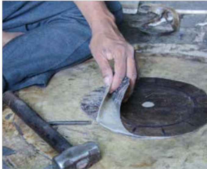
Three layers Buffalo, Goat and Buffalo calf leather is used to make the right side of the mridangam.
