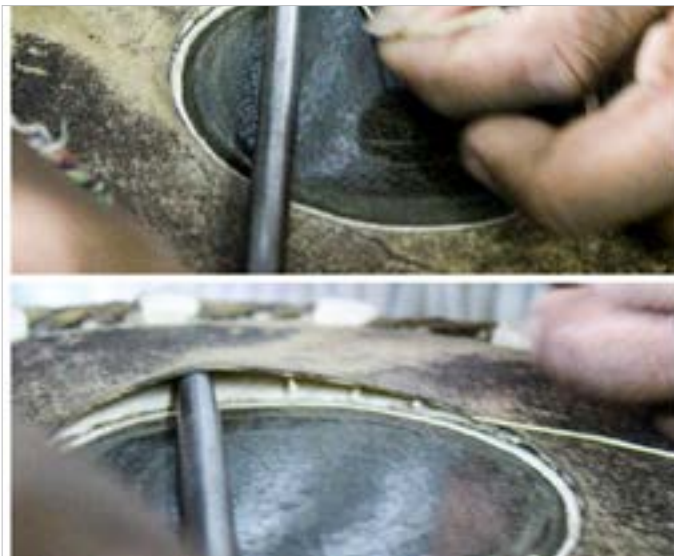
Small stick is placed inside a layer of leather to produce good sound.
