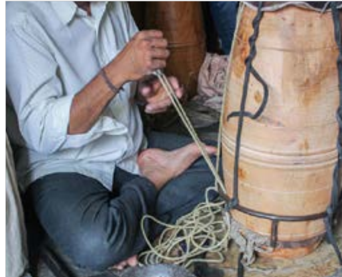
The rope is passed through the iron frame.
