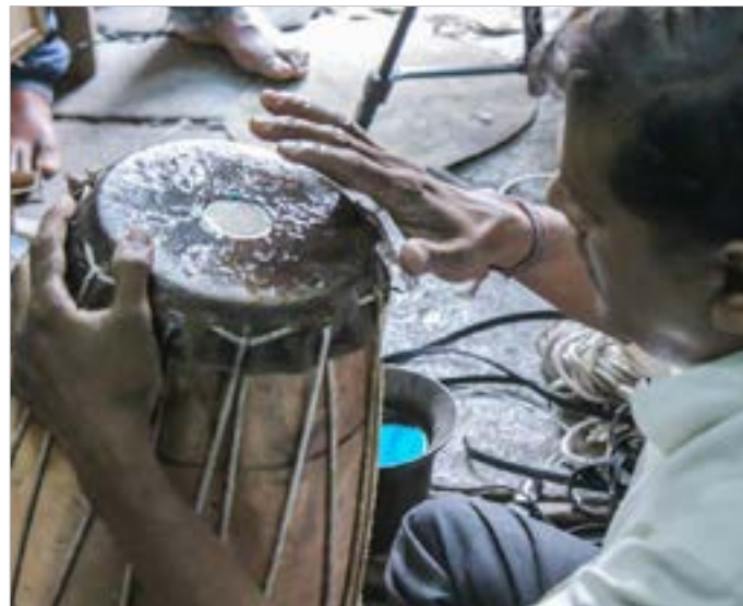
Water is applied frequently to soften the leather.
