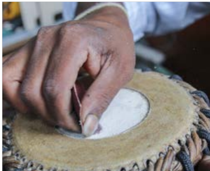
Using sand paper, the surface is cleaned.
