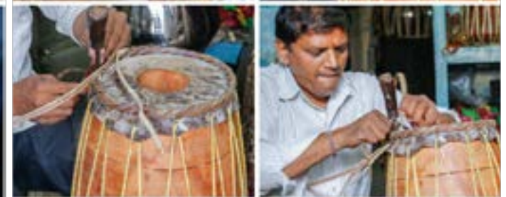
Leather straps is woven to make a circular grip.
