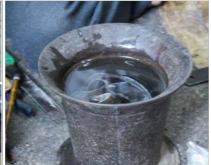
Leather is soaked into water to make it soft.
