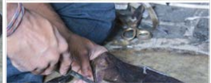
Holes are made on the leather to tie nylon strip.
