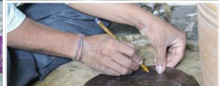
Resonator is placed on leather for marking the required size.
