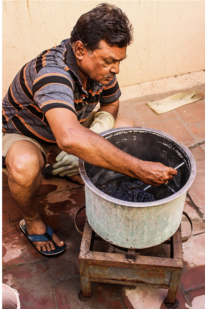
Artisan adds the required quantity of water and color to the vessel and the tied fabric is dipped into it.
