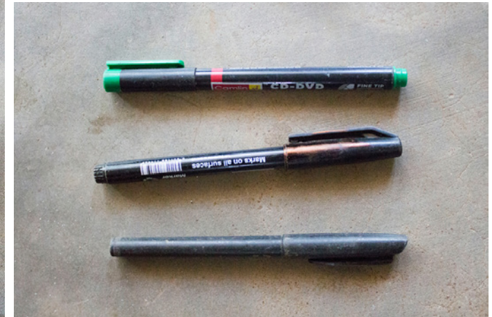
Marker is used for making the margins on the metal.
