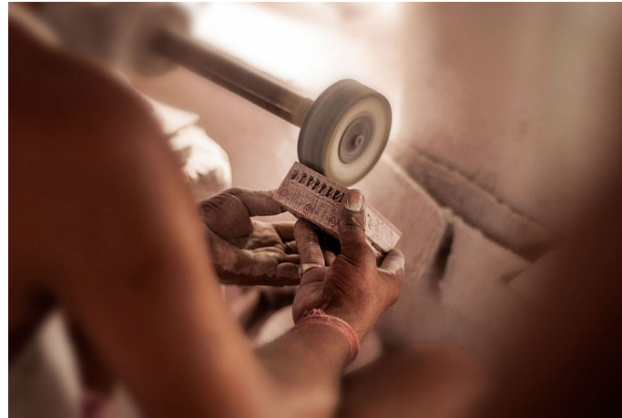
Buffer is used to smoothen the surface and give a shine to the article.
