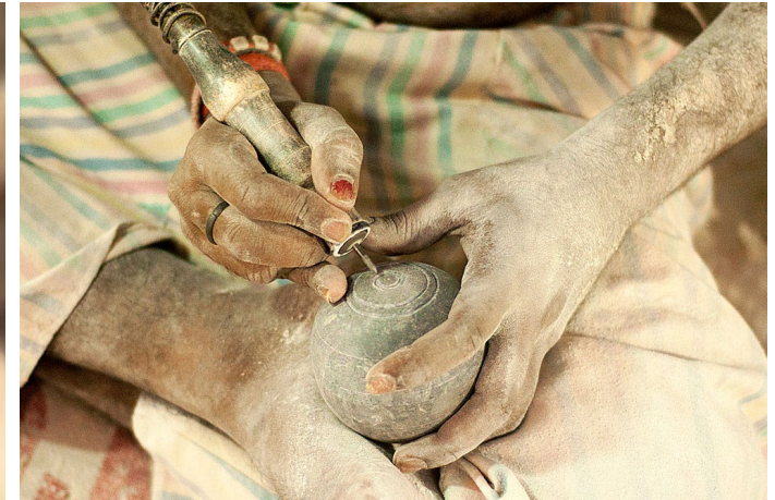
With the help of an electric chisel designs are carved in the marble.
