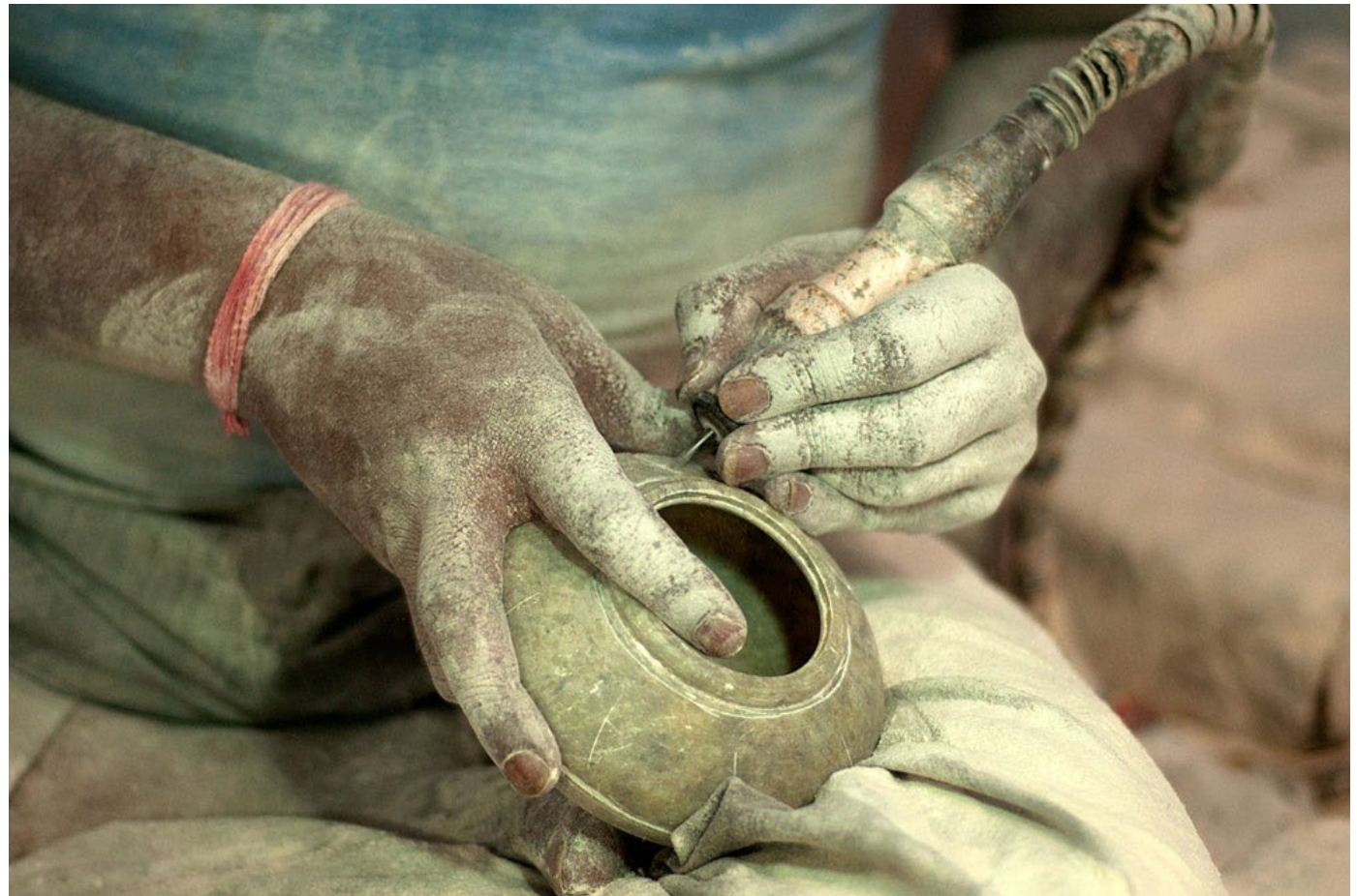
Electric Bits of different sizes are used to carve designs on the marble.
