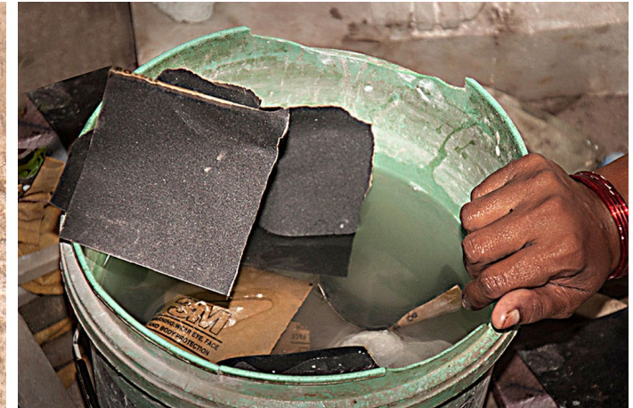
Sand paper is used to smoothen the rough edges.
