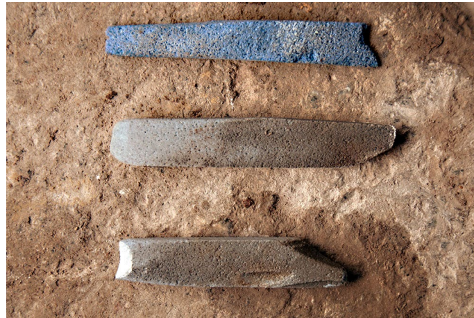
Carborundum stone is used to smoothen the marble surface and bring out shine.
