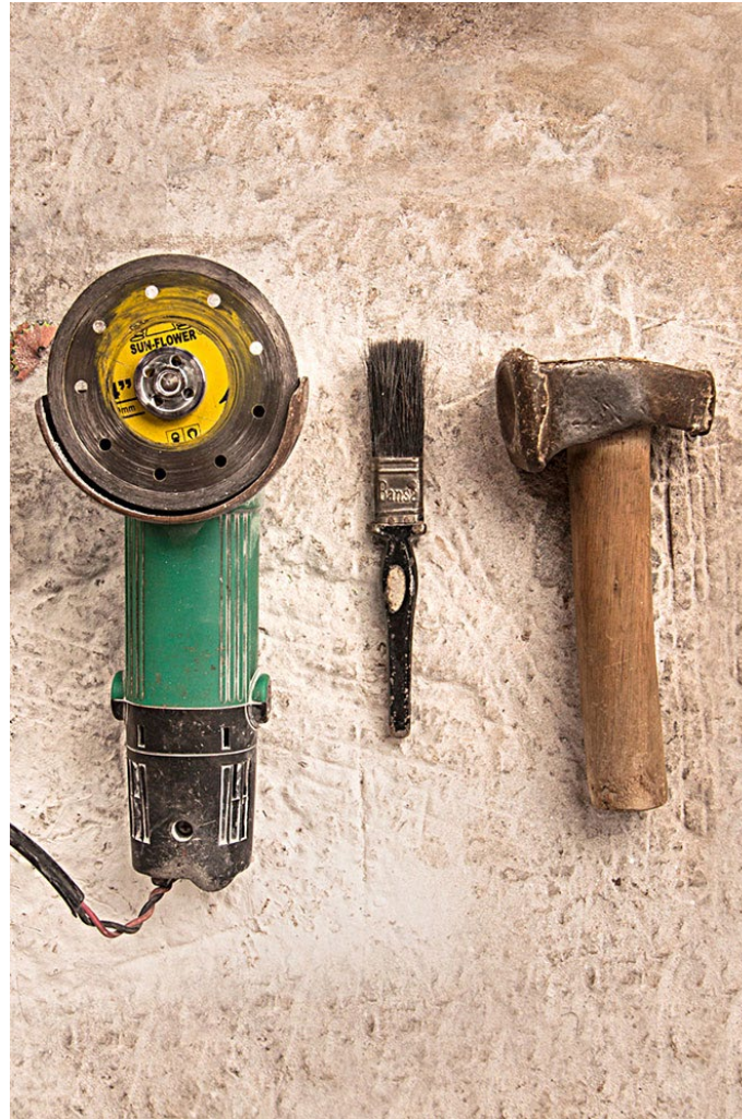
Tools used to carve marble idols into required shapes.
