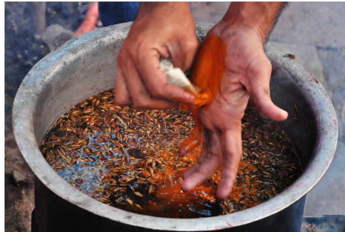
Aligarin powder is placed in a small cloth and dipped, rubbed with hand to the solution for boiling.
