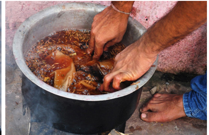
Fabric is immersed and removed several times in sequence in the solution to check changing of the color.
