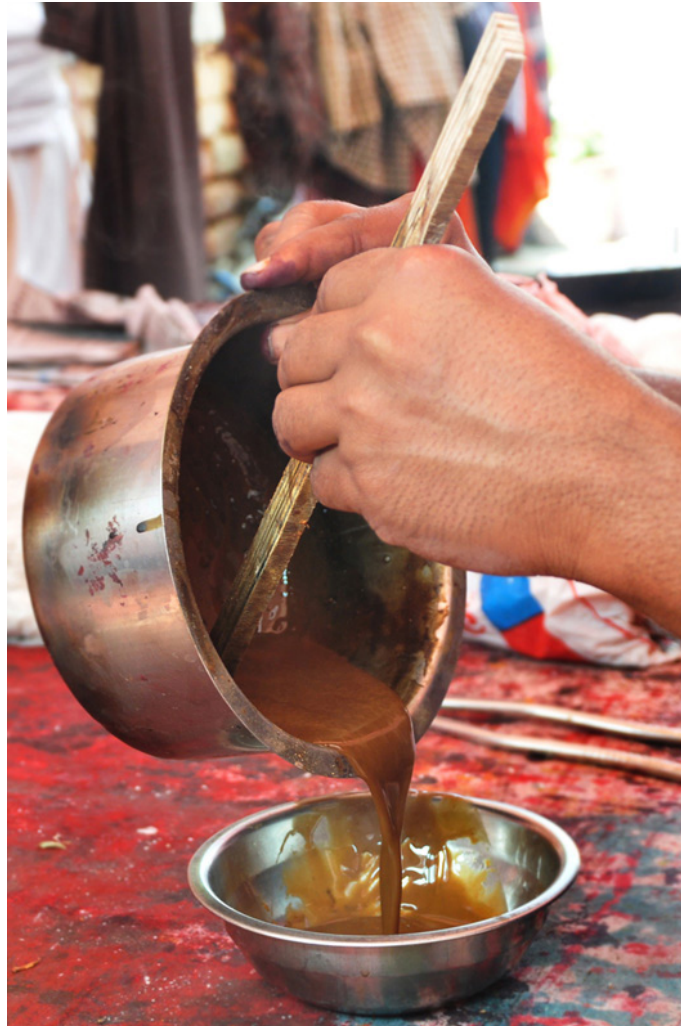
Mixture of jaggery, scrap iron metal and kachu ka atta (tamarind seed powder) is heated for black color.
