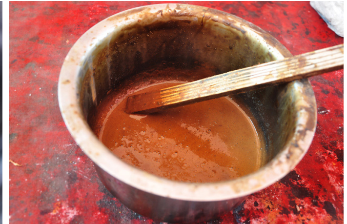
Heated mixture of jaggery, scrap iron metal and kachu ka atta for black color.
