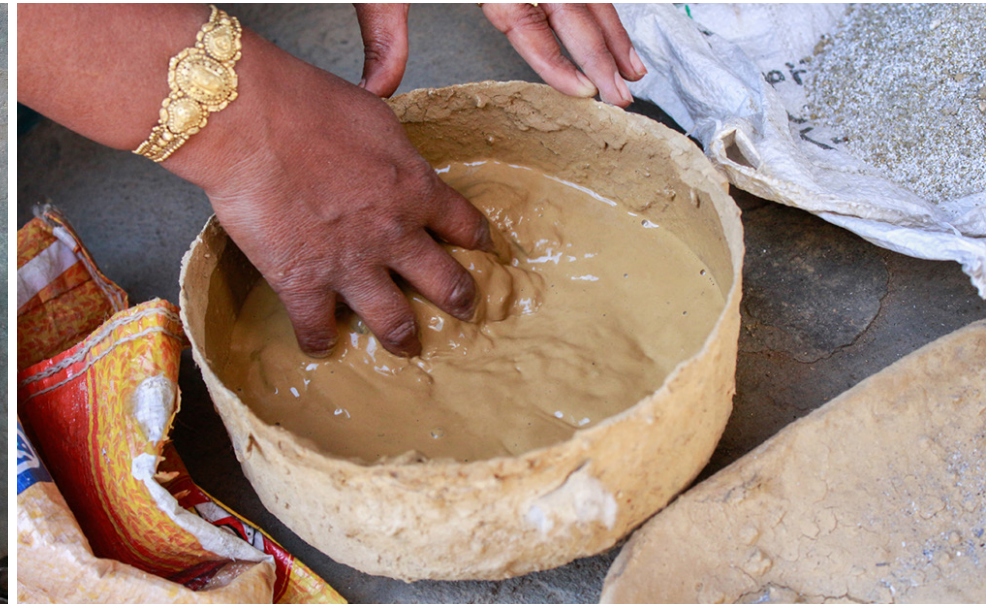
Mud water and mud mixed with raw cotton are used to wrap the bell before placing in kiln.
