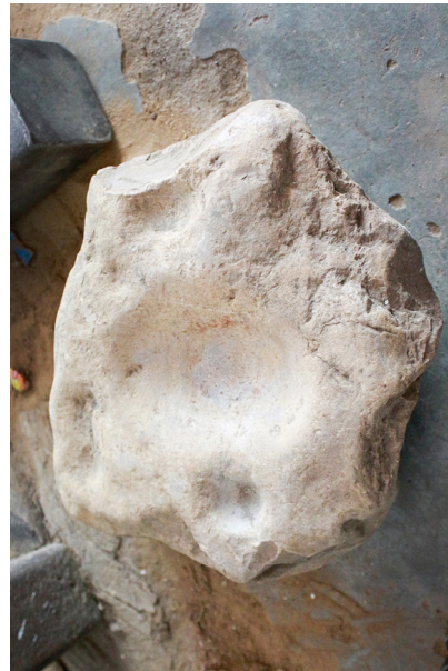
Customized tool to shape the metal sheet according to the requirement.
