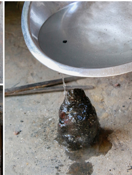
The object is taken out from the kiln and dipped in cold water.
