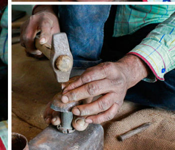
The hole is formed on the cap and handle for the bell is attached.
