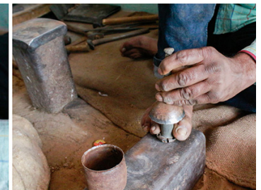
Marked sheet is cut and beaten to get a dome shape.
