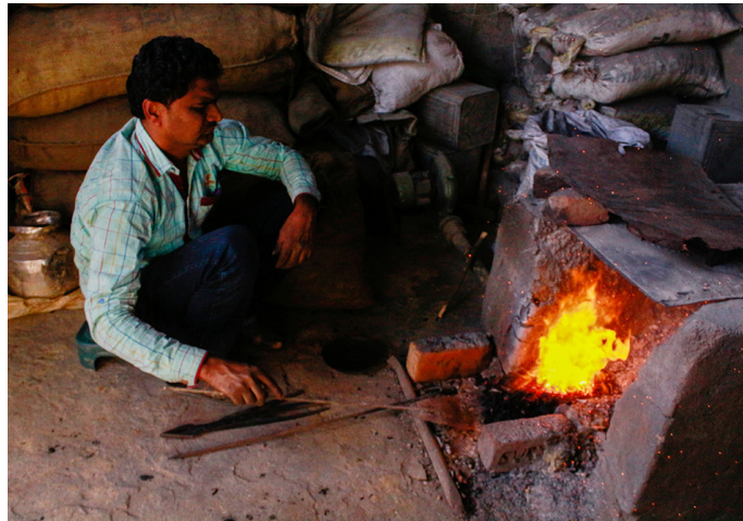
Kiln is used to heat the metal bells.
