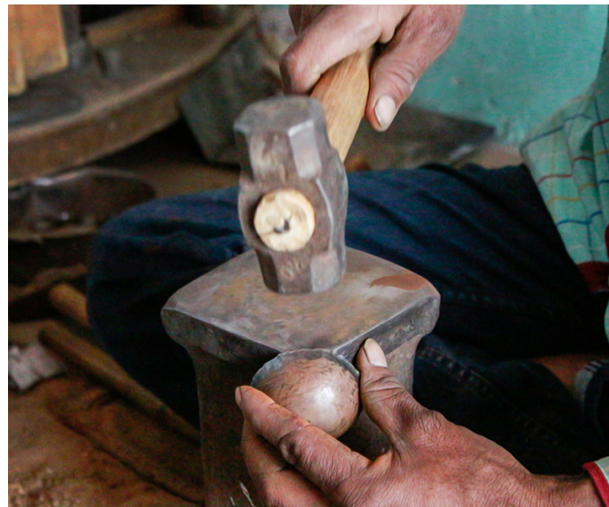
Smoothing the sharp edges by hammering.
