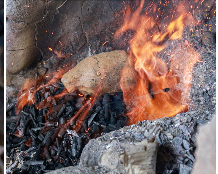
The wrapped bell is baked in the kiln with high temperature.
