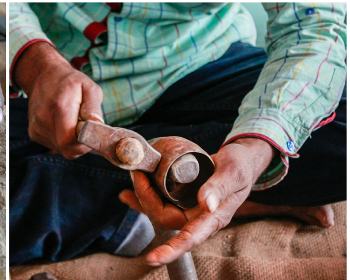
Shaping the metal sheet by beating to obtain a required shape.
