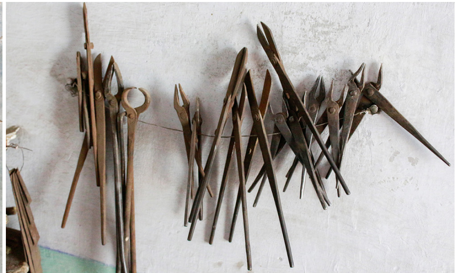
Different size cutters are used to cut the metal sheet.
