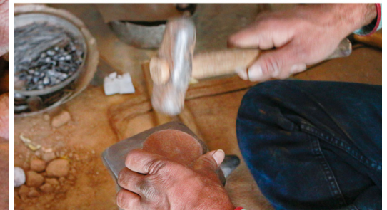
Marked sheet is cut and beaten to get a dome shape.
