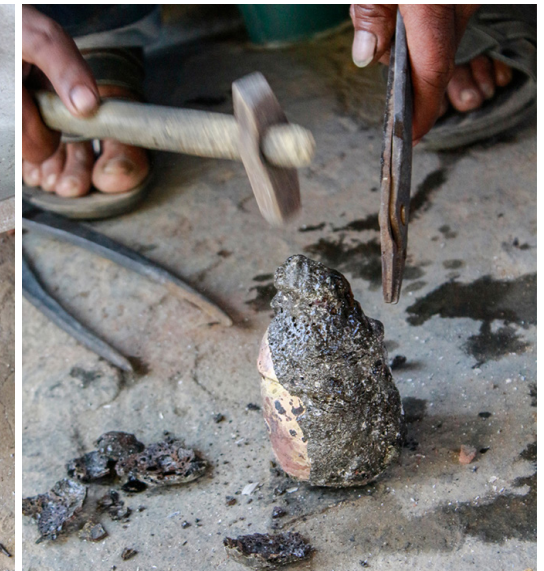
The cooled object is hammered to break the mud cover.
