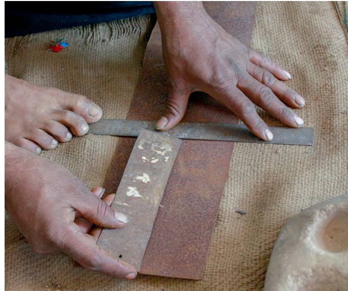
Initially metal sheet is measured using customized measurement tools.
