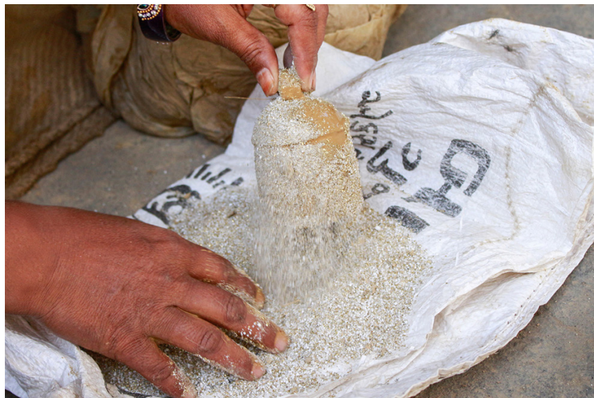
Metal powder (brass, zinc, copper and iron) is coated to the wet bell.
