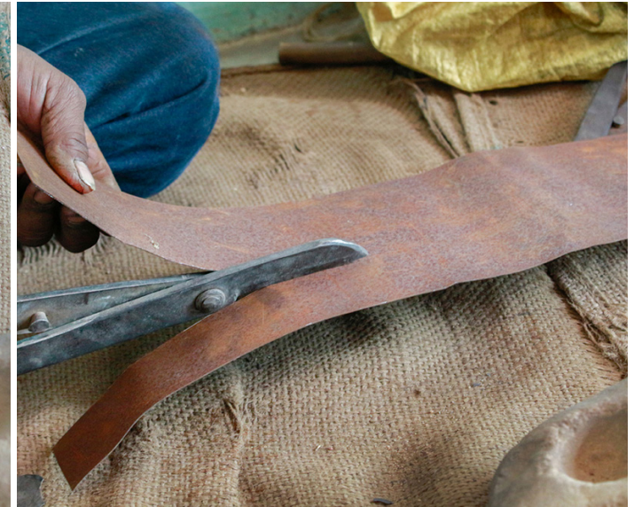
Metal sheet is cut with the help of metal sheet cutter.
