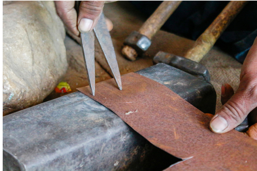
Metal sheet is measured and marked using compass.
