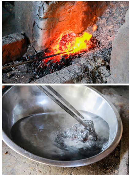
The object is taken out from the kiln and dipped in cold water.
