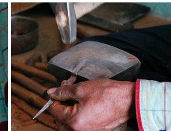
Marked sheet is cut and beaten to get a dome shape.
