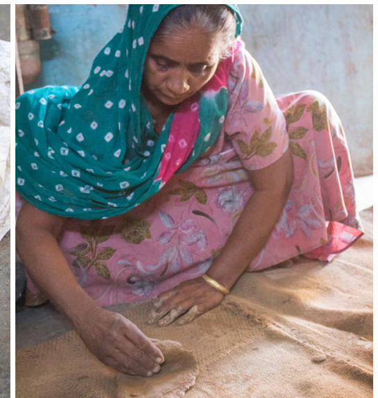
Mixture of raw-cotton and mud is kneaded thoroughly.
