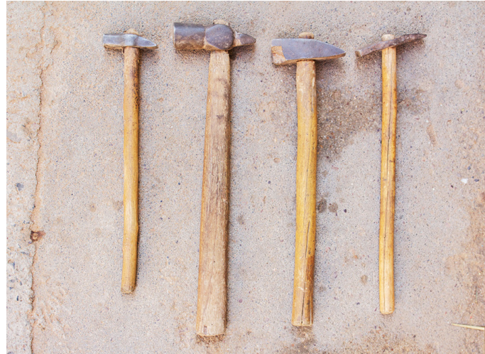
Hammers are used to shape the metal sheet and for tuning the bell.
