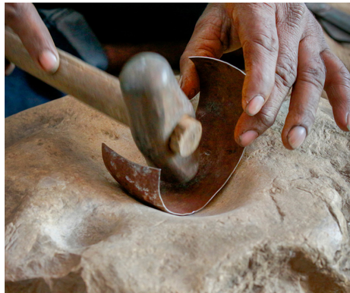
Metal sheet is bent by hammering.
