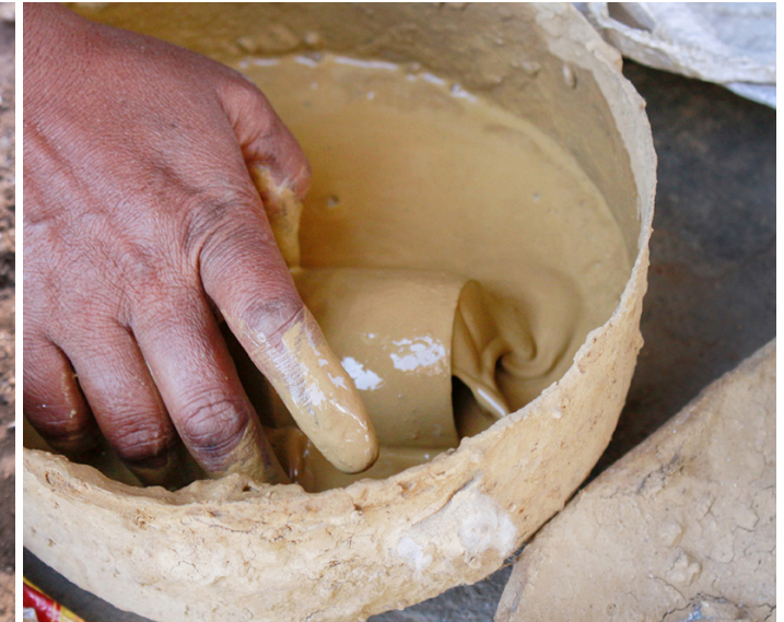
Bell is dipped in mud water before coating the metal powder.
