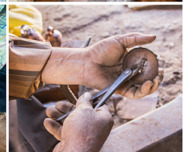
The hole is formed on the cap and handle for the bell is attached.
