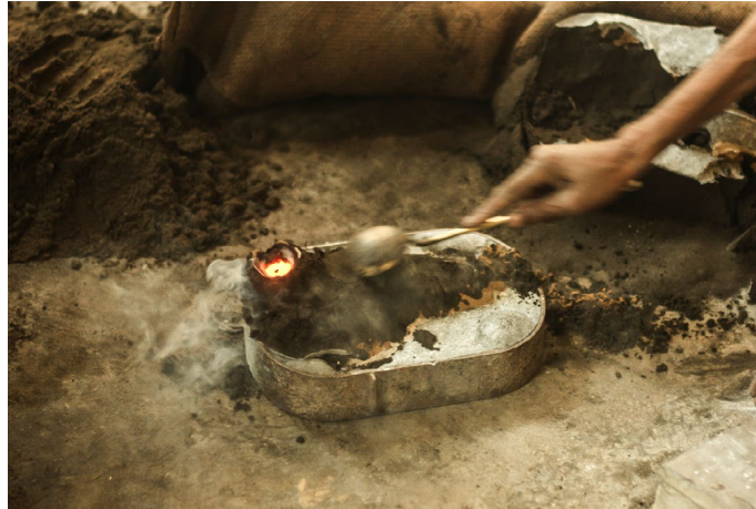
After cooling, craftsmen separates the filling material from mold box.
