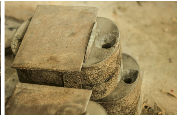
Prepared molds arranged (one above) to pour molten material easily.
