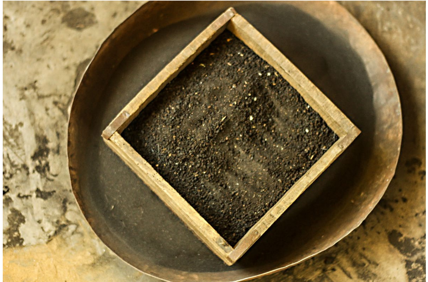
Sand is refined and filled in the mold for casting.
