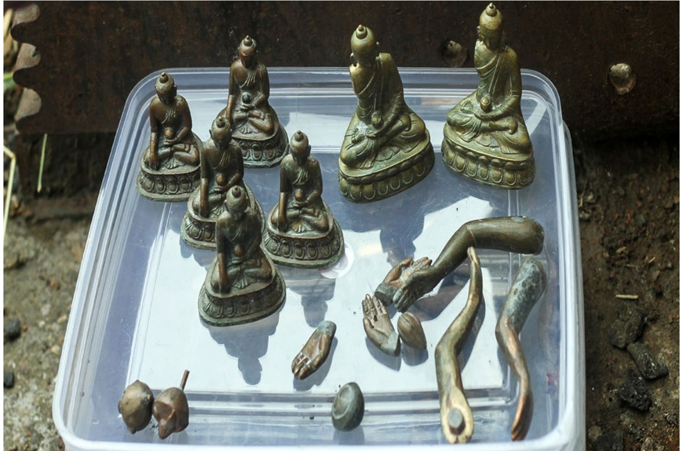
Completed full idols and body parts are casted separately.
