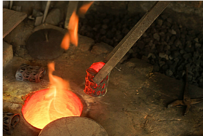
80% copper and 20% bronze is added in the furnace to melt.
