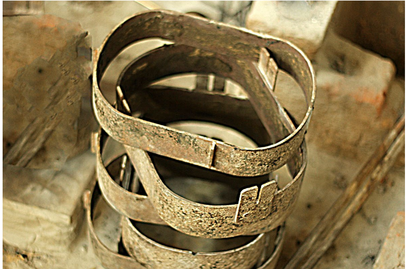
Frames in which the sand casting is done.
