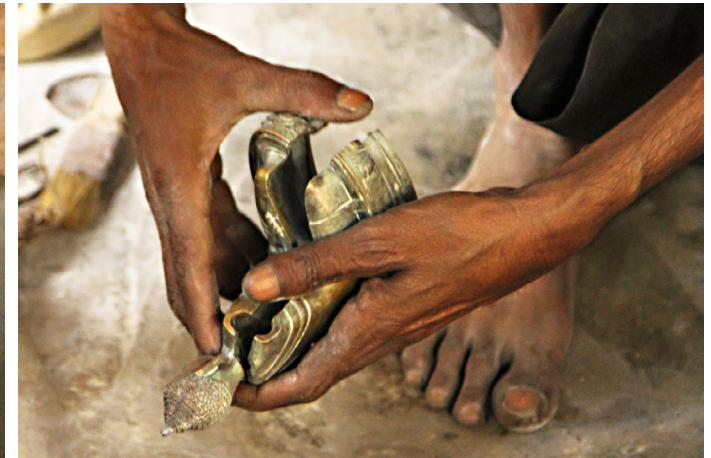
Master casted piece of the idol is used to prepare the mold.
