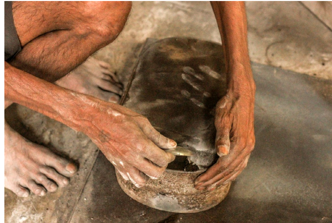
A small hole is scooped to pour the molten metal.
