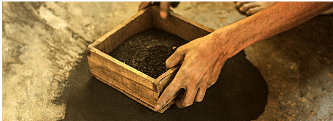
Sand/reusable sand used as filling material in casting is filtered.
