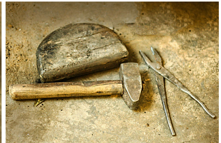
Tools used for breaking the mold on the molten surface.
