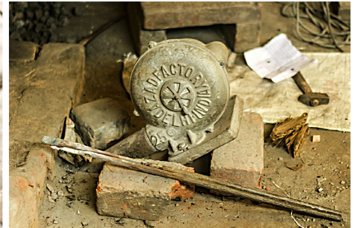
Hand blower is used to heat the furnace.
