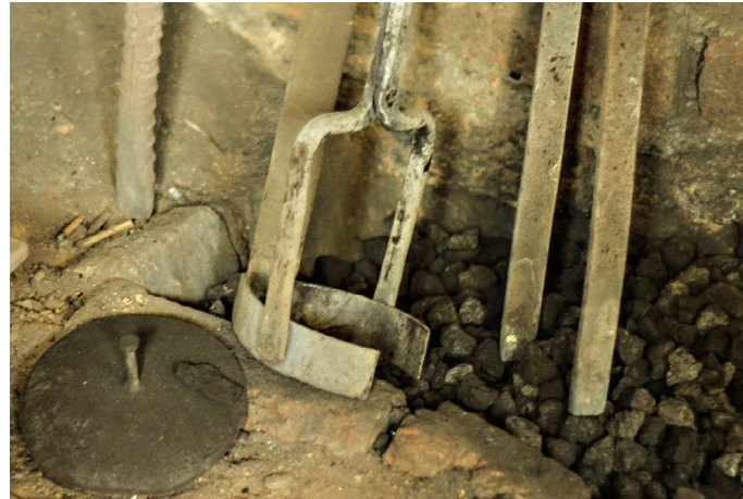
Tongs and flask tongs are used for holding and lifting the crucible.
