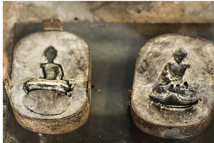
Masterpiece idol is removed leaving the impression in the mold.
