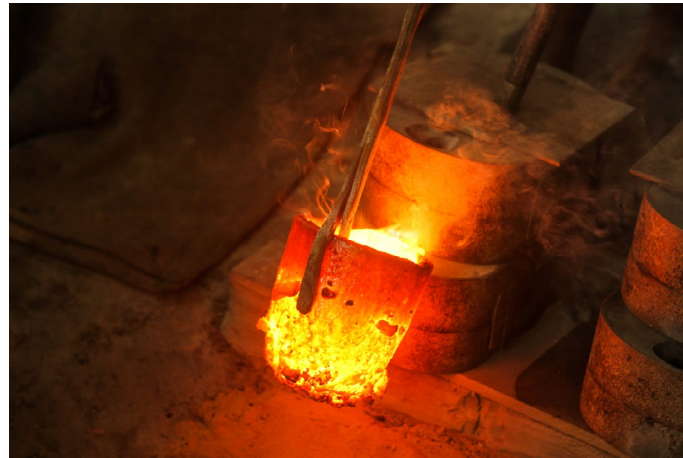
Molten material is poured in the mold box.
