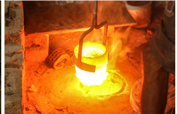
Metals are melted at high temperature of around 950 degree Celsius.
