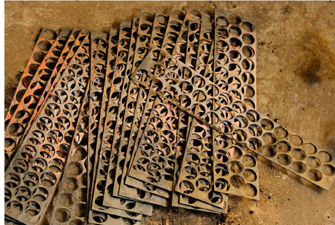
Left over parts from copper sheet strip is reused.
