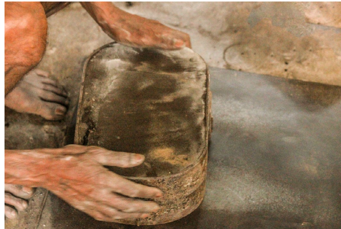
The mold frame is filled with the sand mixture.
