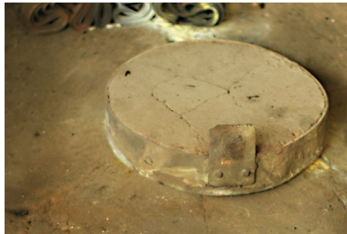
Bhatti (furnace), which is made in the ground is covered with a concrete lid that is used for melting the metal.
