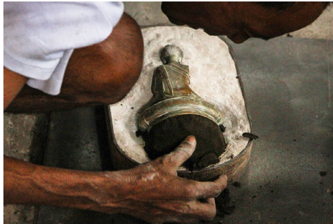
Joined piece is placed in mold to create the impression of the idol in the mold.
