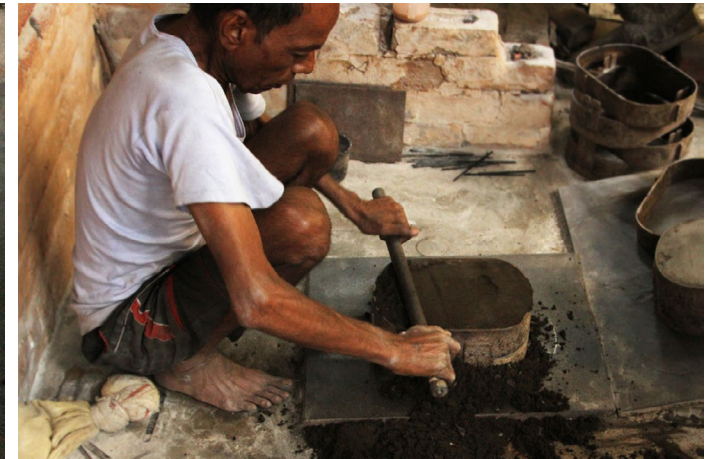
Other side of the mold frame is placed and filled with sand and pressure is applied on it to settle closely.
