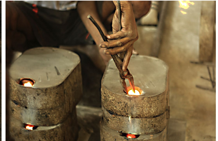
Excess casted metal is removed.
