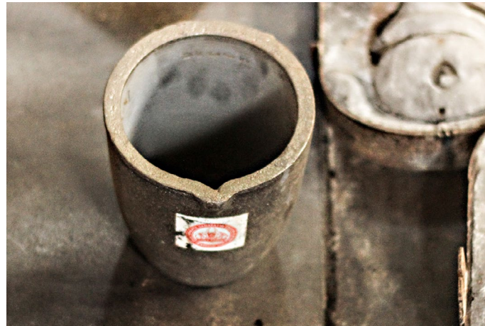
Crucible is used to melt the metals.
