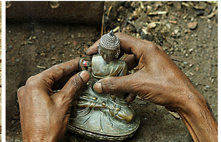
Body parts like hands are attached separately for five inches and above cast parts.
