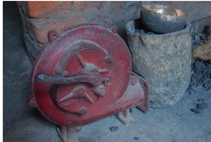
Hand crank blower is used to heat the coal.
