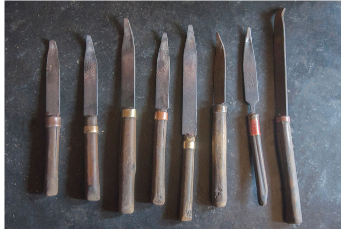
Different types of files and scrapers to make the metal in shape and smooth.
