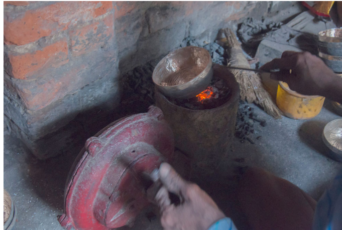
The brass metal is heated to apply tar on it.
