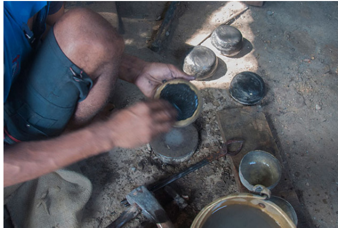
Coal is applied on the brass metal to observe heat.
