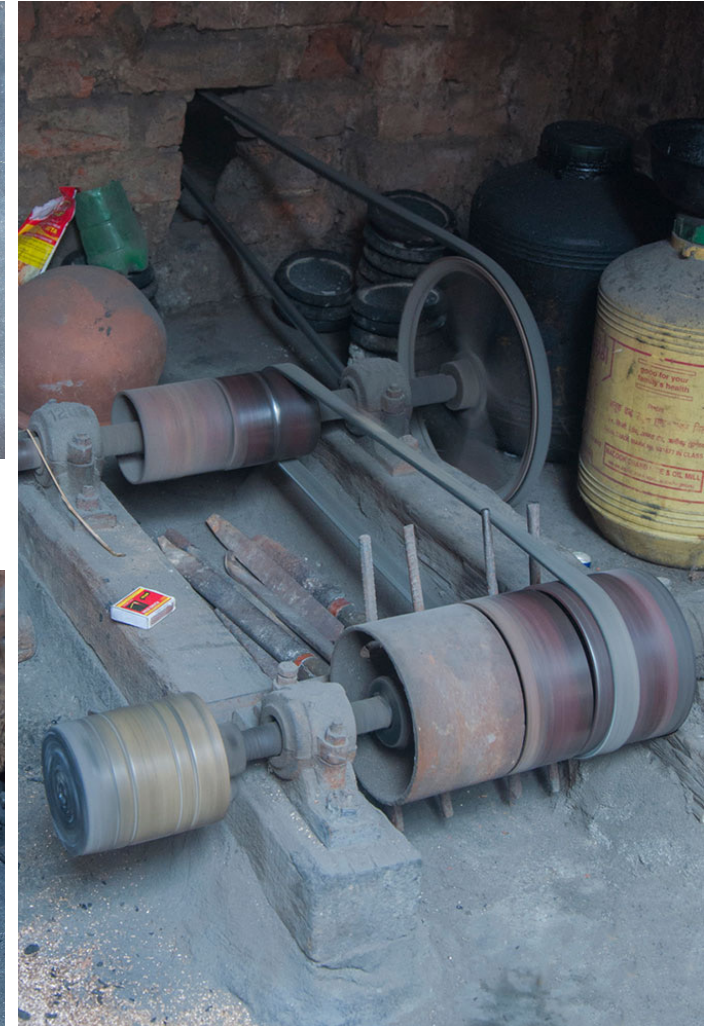
Lathe machine is to rotate the brass metal during the refine process.
