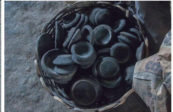
Mould made of earthen pot to cast ingots of brass metal.
