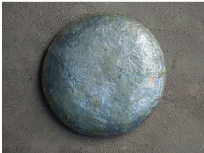
Copper and zinc is melted together to attain ingot of brass metal.
