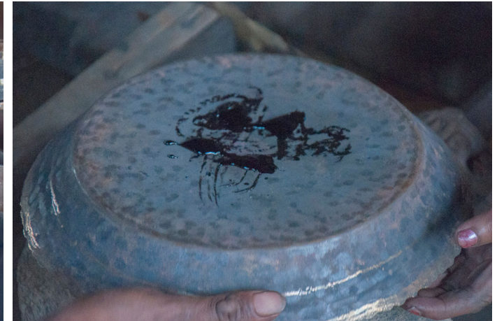
Tar is applied on the bottom of brass metal to stick on the machine.
