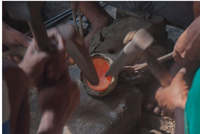
The ingot is hammered to attain the required shape.
