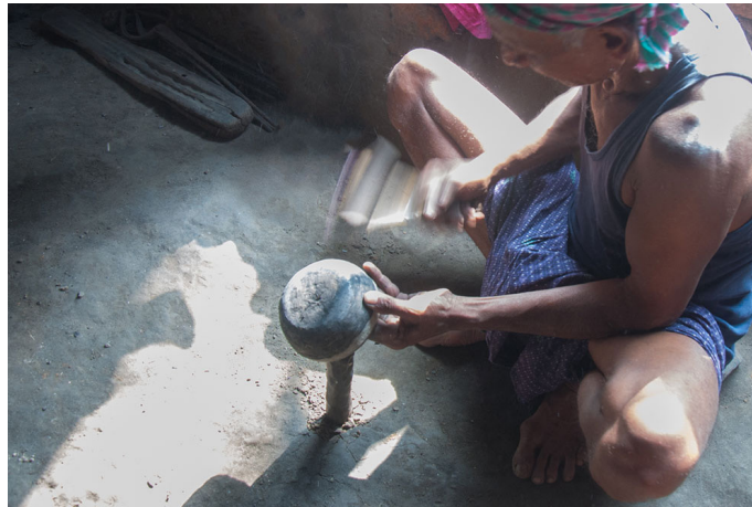
The brass metal is hammered to attain proper shape.
