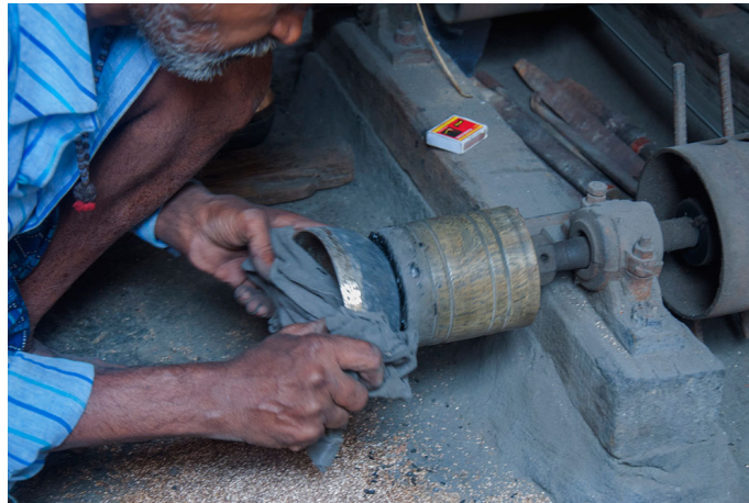
The brass metal is fixed to the lathe machine for refining.
