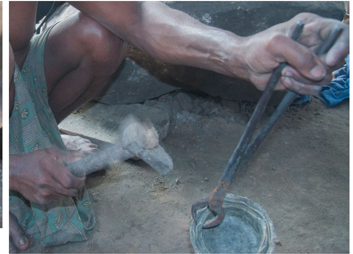
Heated ingot is placed on the required shape of the mould.
