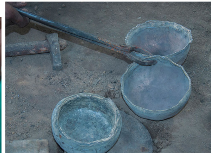
The brass metals are separated using hammer.
