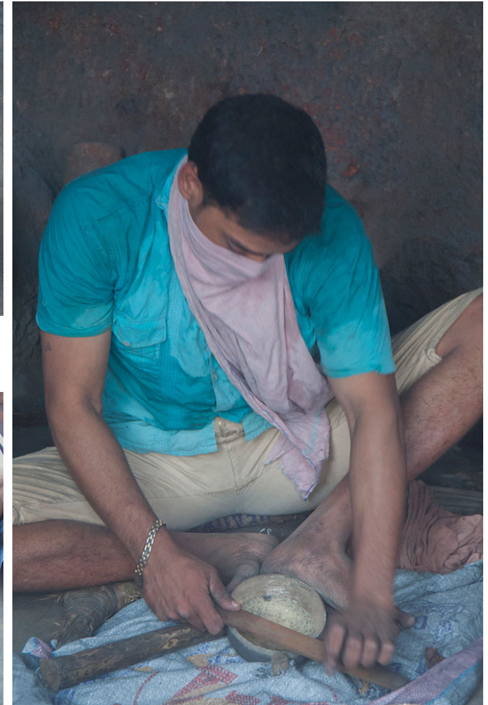
The brass metal is smoothen on the edges using the file.
