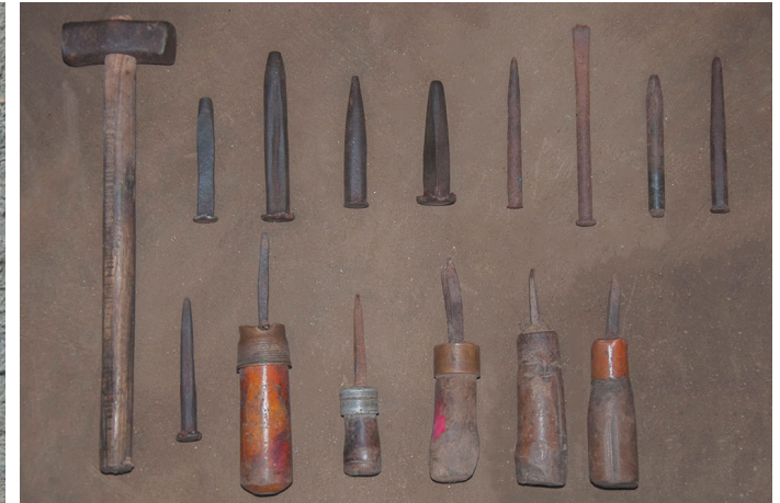
Hammer and Different types of chisels to engrave designs on the metal object.
