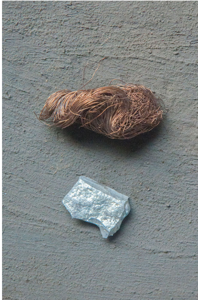
Copper and zinc is melted together to make brass metal ingot.
