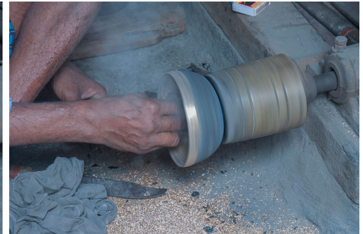
The brass metal is buffered using brass wire sponge.
