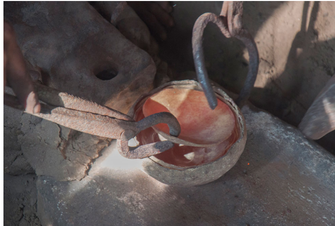
Heated ingot is placed on the required shape of the mould.
