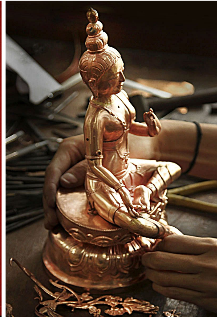
Parts of the sculpture is made separately and joined together.
