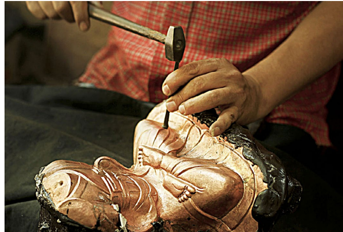
Shaped sheet is arrested on lacquer for support.
