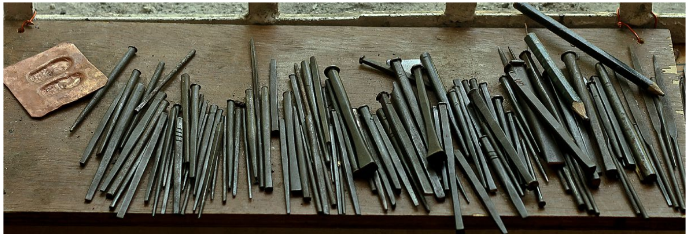
Various kinds and sizes of chisels used in sculpting.
