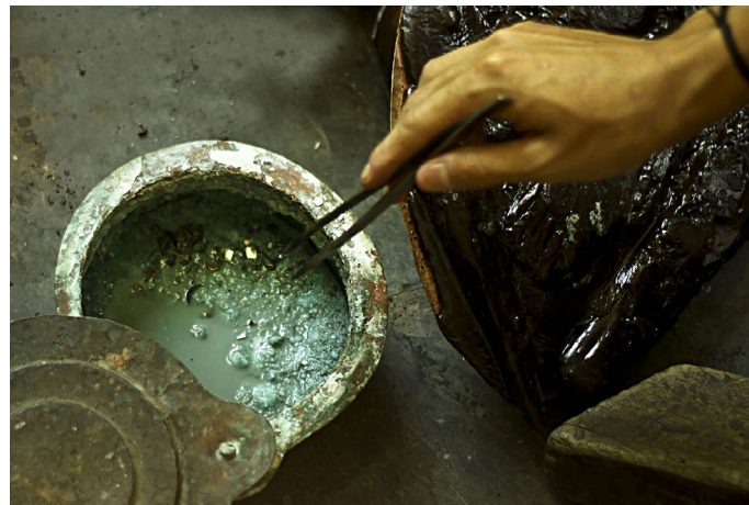
Mixture of zinc, brass and copper in a ratio is placed on the line of two halves.
