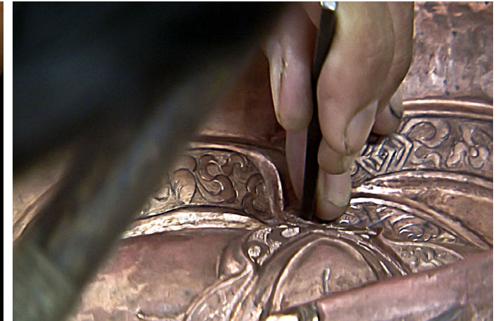
Detailing is embossed using various types of chisels.
