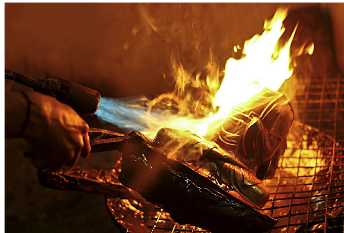
Lacquer is removed by heated and sheet is dipped in diluted acid to remove leftover.
