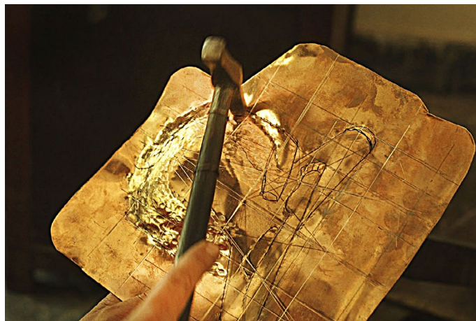
Copper sheet is hammered to get a basic shape of the sculpture according to the design.
