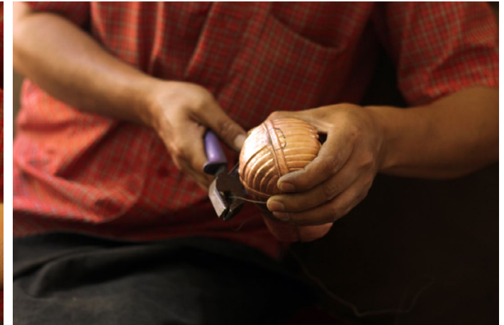
Both halves of the head are tied with a metal wire.
