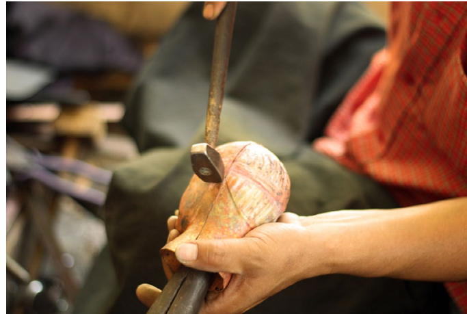
Front and back half of the head of the statue is hammered and shaped to match.
