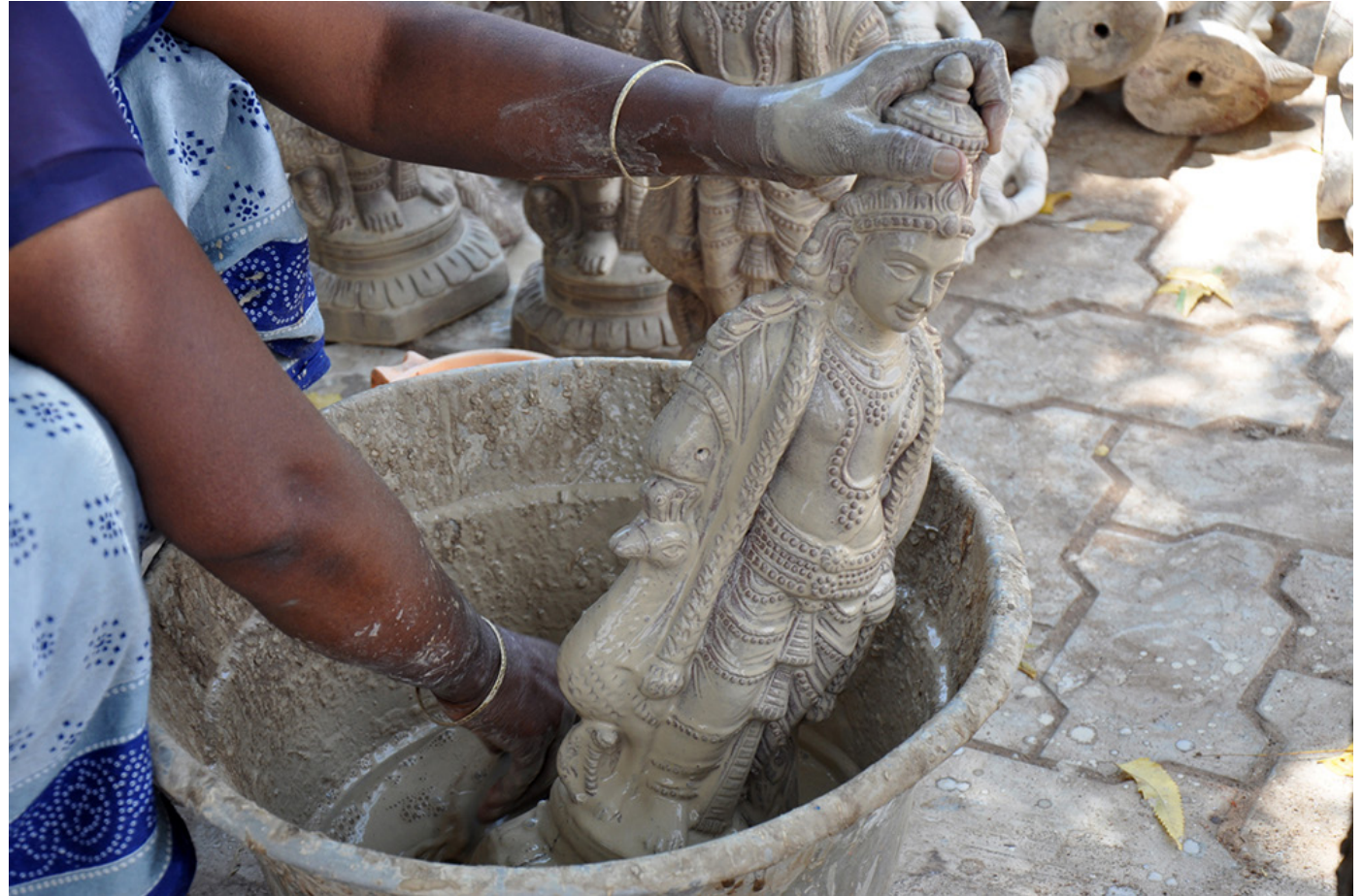
Premier coat is applied on the mold before painting process.
