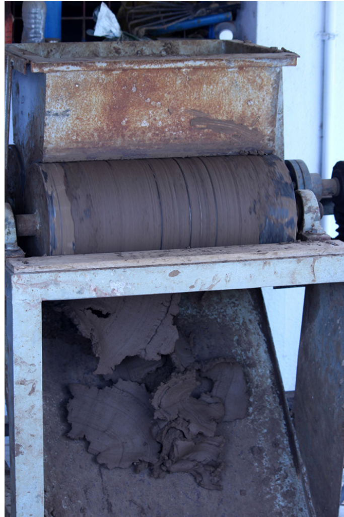
Collected mud from the lake is blended using a blending machine.
