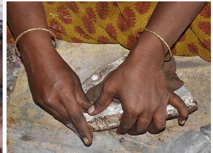
Artisan filing clay both half of the mould.
