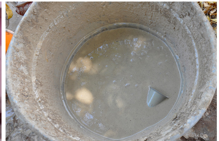
Plaster of Paris used for preparing the mold.
