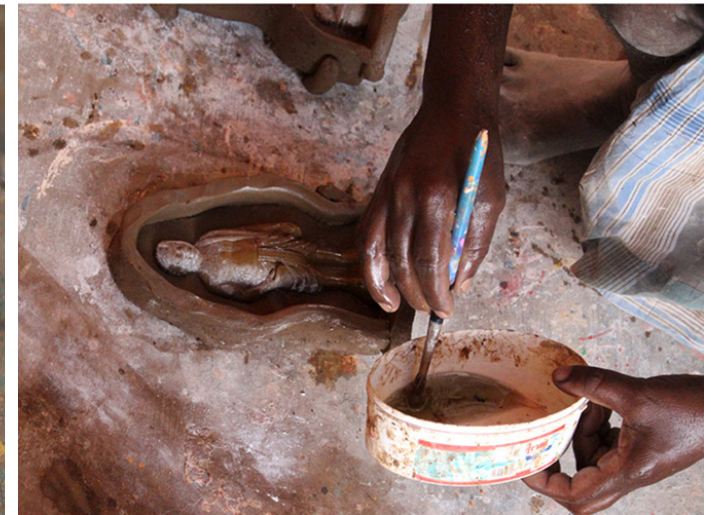
Layer of kerosene is applied on the model to avoid stickiness of mold material.
