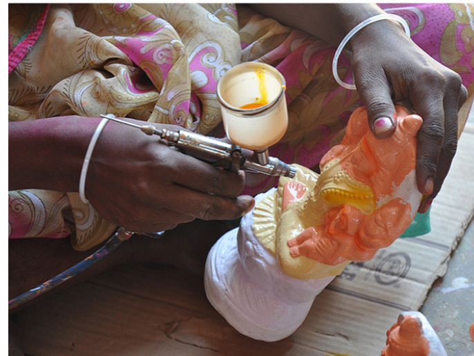
Spray gun is filled with color and then the dolls are colored using spray gun.
