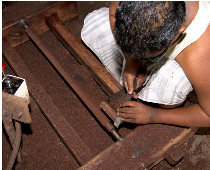
Artisan turning the wooden block on the lathe machine.
