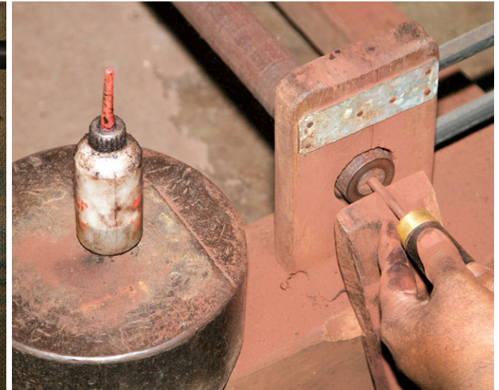
Oil used while turning the wood.
