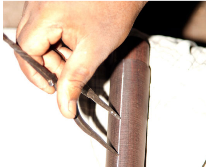
Based on the line holes are marked.
