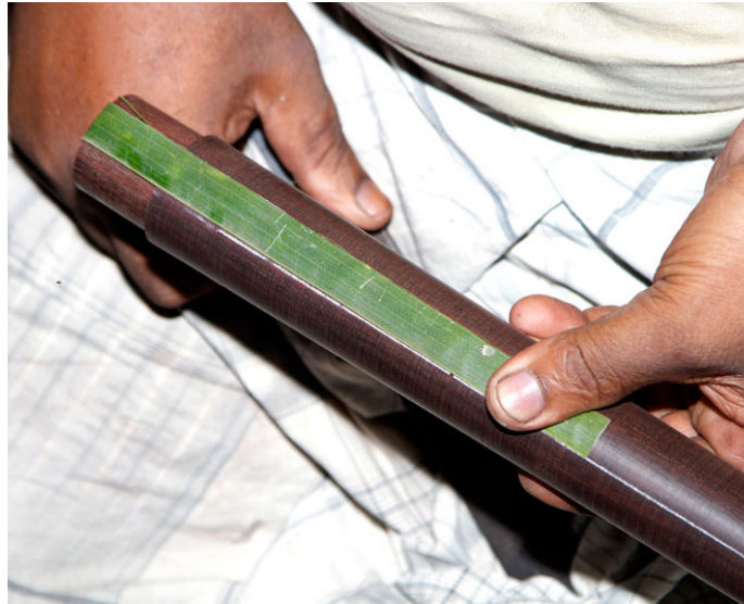
Leaf of a coconut tree is used for measurement while drilling holes.
