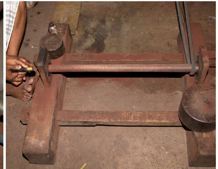
The process of removing the inner pulp of wood.
