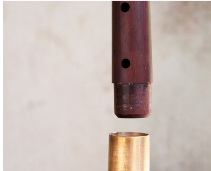
Brass ring is inserted in the middle of instrument..
