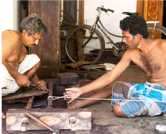
Traditional method of turning with rope.
