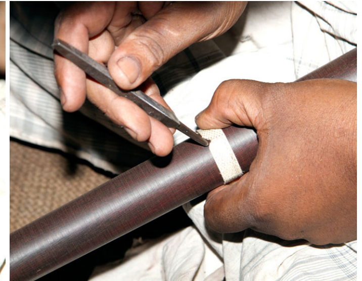
Rough marking is done before drilling.
