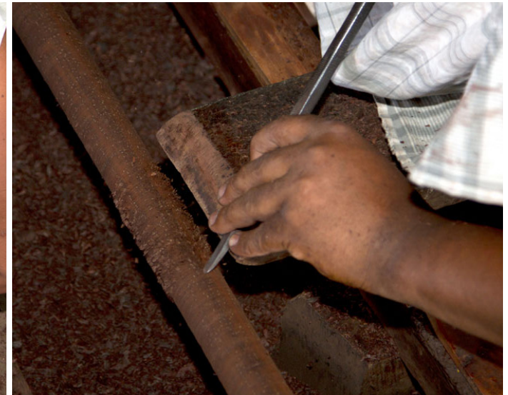
Turning is done to convert the wood piece into a circular wood stick.
