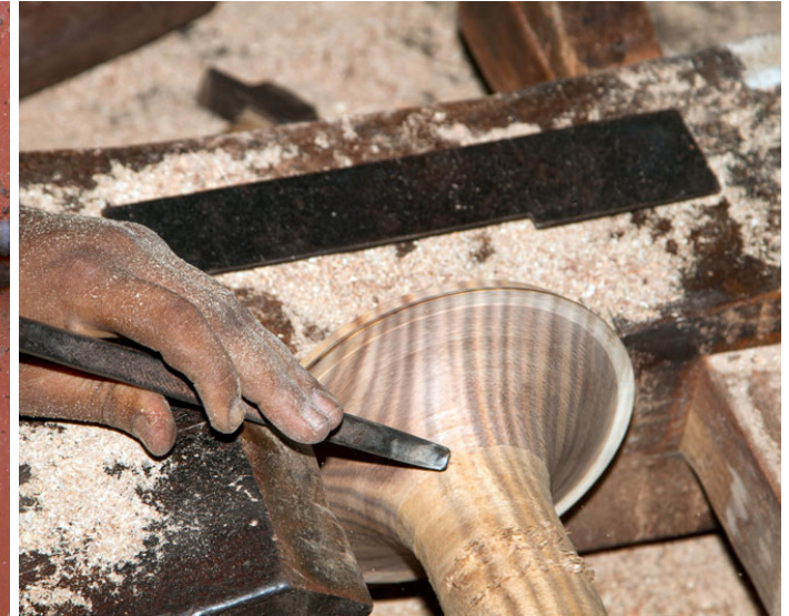
Turning the flaring bell.
