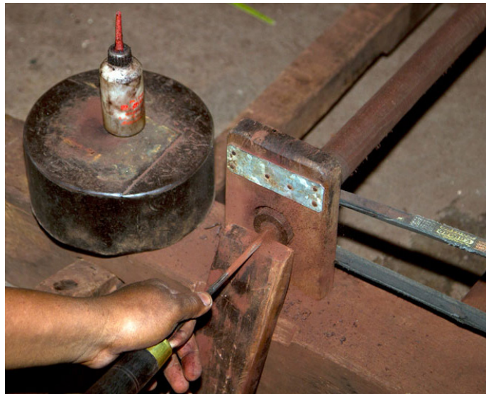
The file is inserted into the wooden stick while it is in motion.
