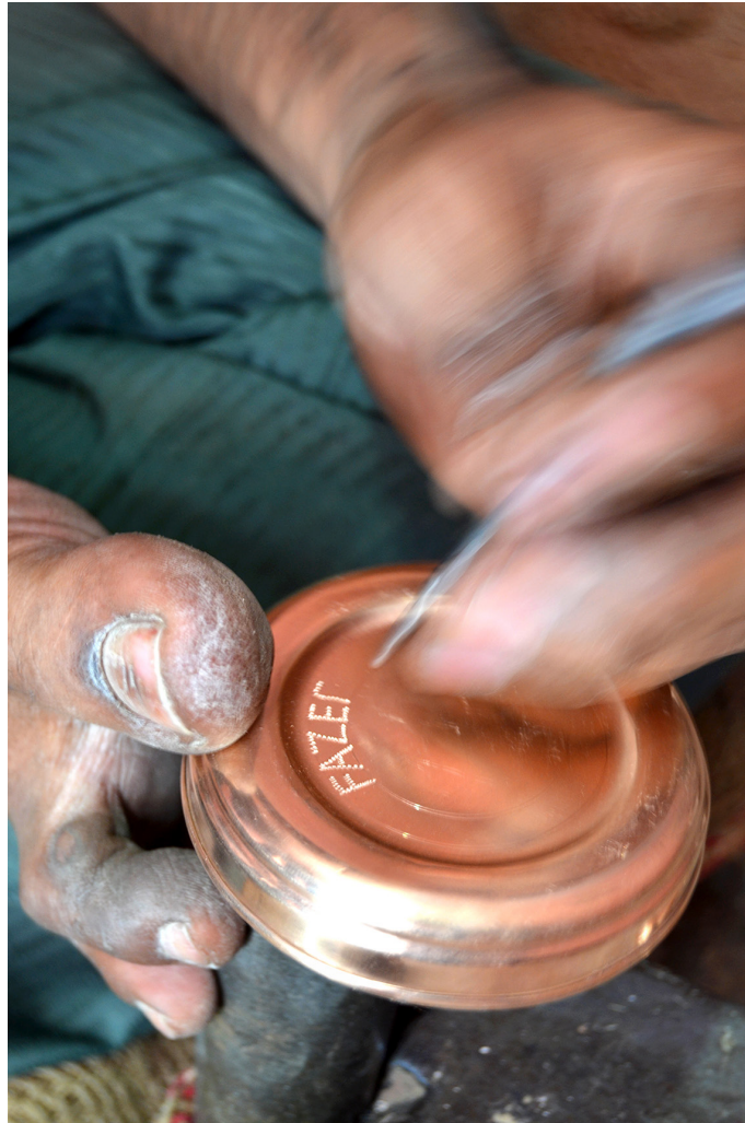
Etching a name on a copper lid.
