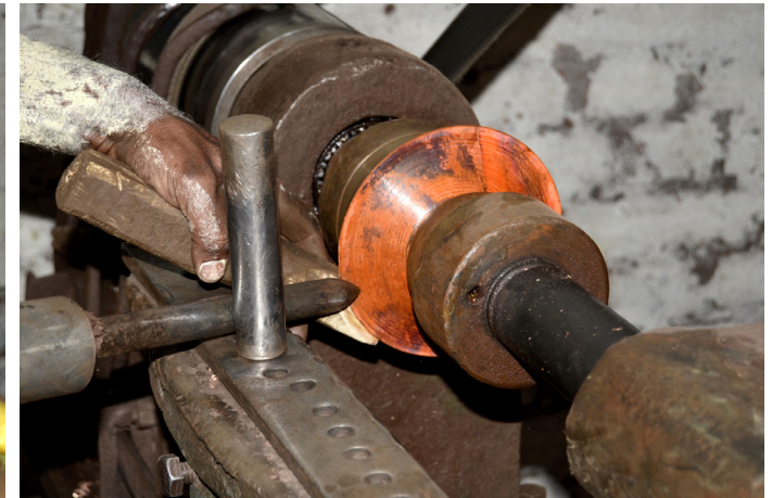
Moulding/ shaping the copper sheets.
