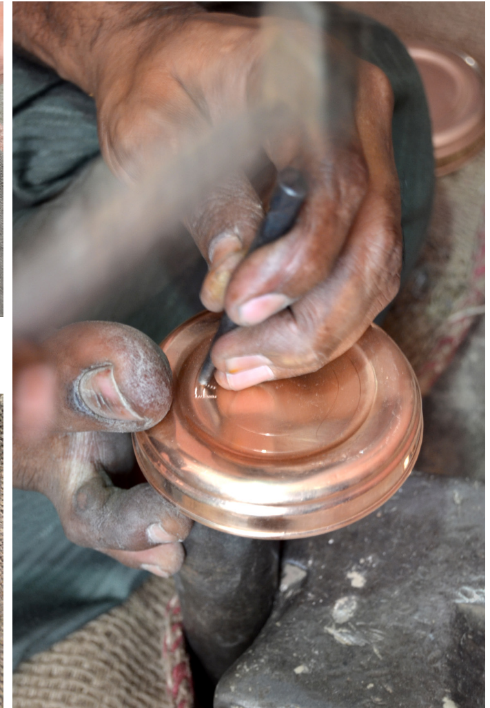
Etching a name on a copper lid.
