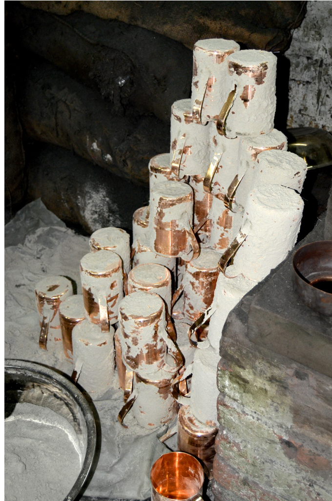
Copperware coated with a chemical powder/dust before buffing.
