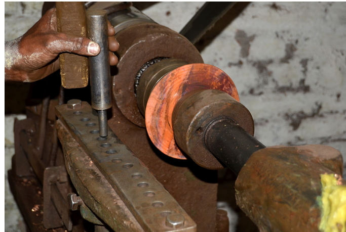
Moulding/ shaping the copper sheets.
