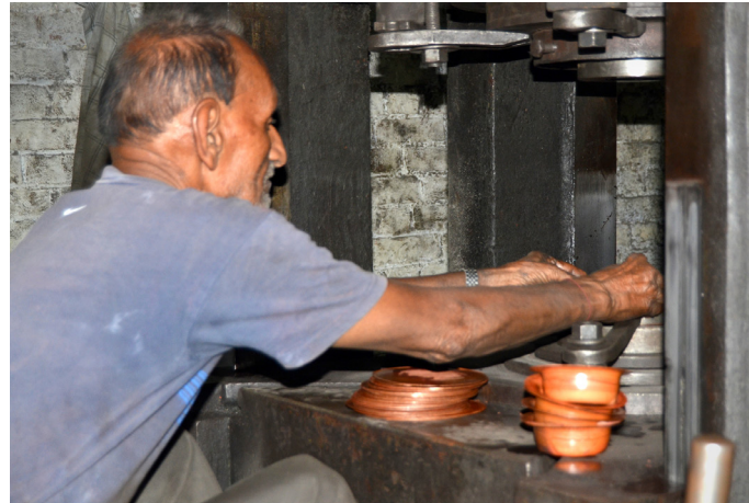
Moulding/ shaping the copper sheets.
