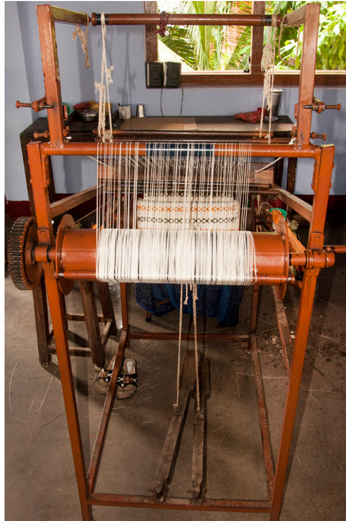
A handloom weaving machine either a “vimala Loom” or “Frame Loom” used in weaving the palm fiber strands together.
