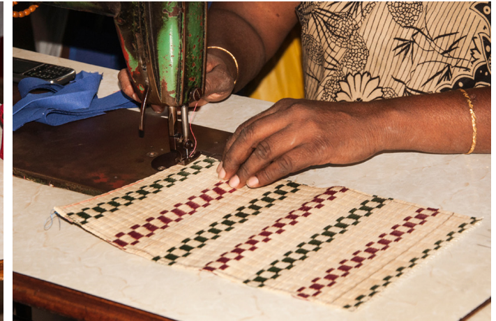
Artisan then stitches along its borders, such that the fiber strands won't fall loose.
