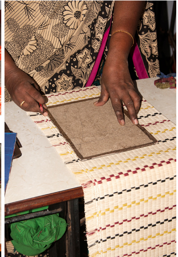
Artisan then marks the mat with a template of required dimensions.
