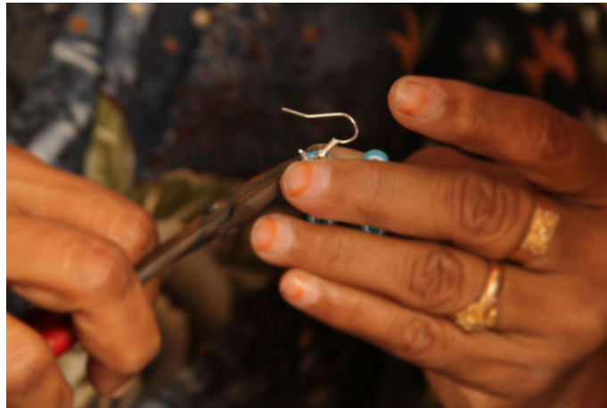
Attaching the ear wire and the ring with the slip joint pliers.
