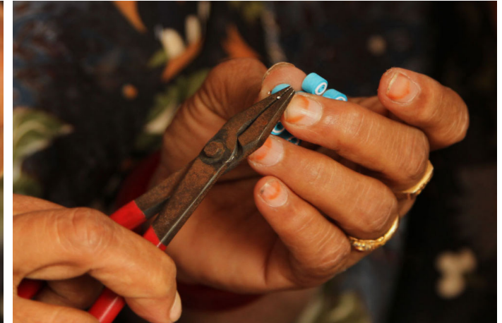
Tightening of ring with the help of slip joint pliers.
