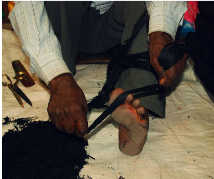
Craftman using his toe to hold the threads.
