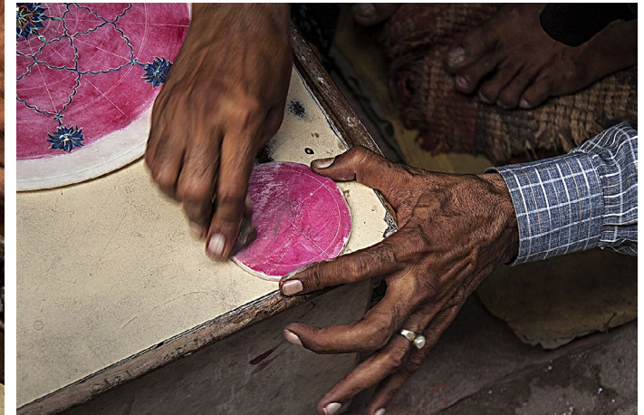
Article is rubbed with a stone to reduce the shade of the color.
