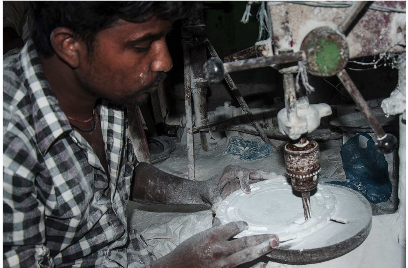
Drilling Machine is used to make holes and design patterns on the marble.
