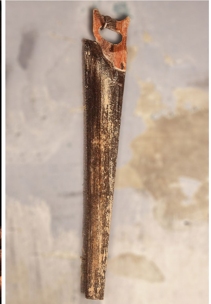
Long length saw is used to cut the marble in required shape and size.
