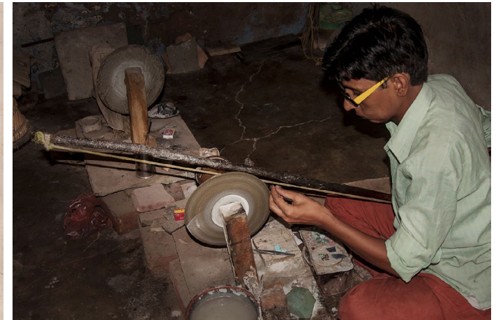
Carving Tool is used to carve the stones in required designs and shapes.
