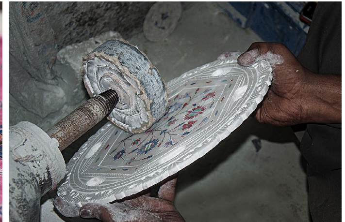
Finished article is buffed to give a smooth finishing and shine.
