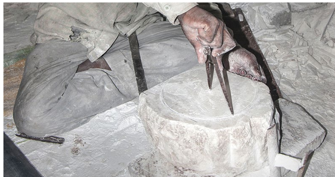
Initially required measurements are drawn on the marble.
