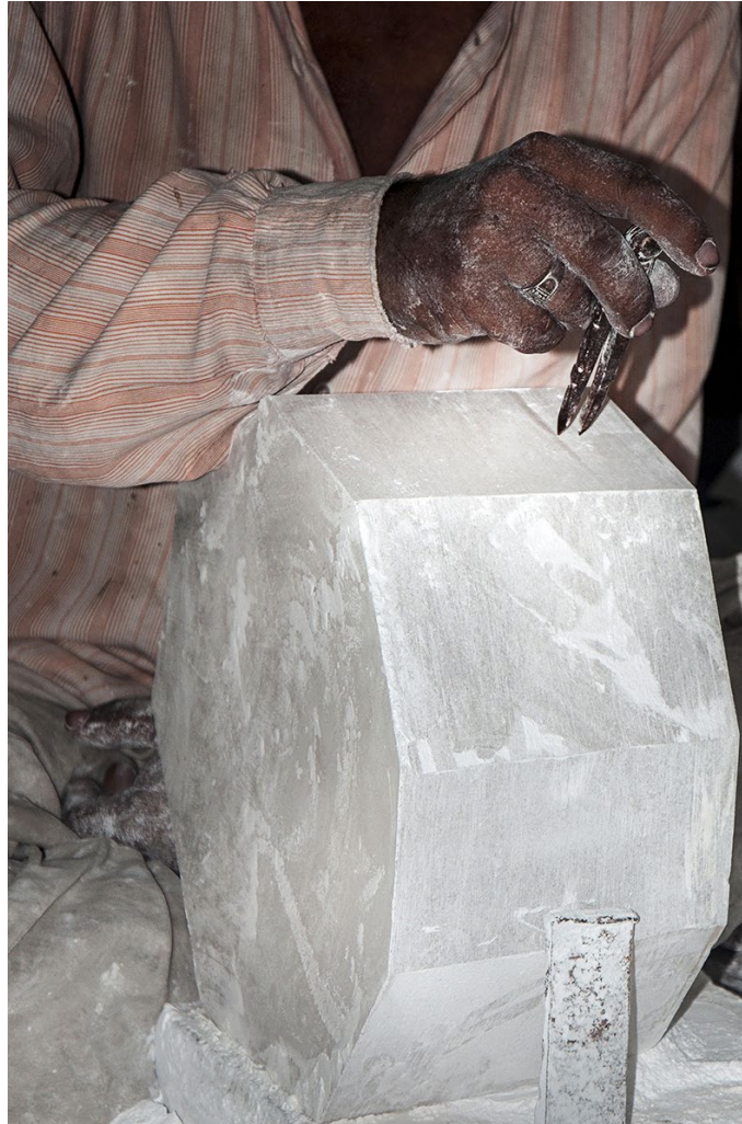
Measurement for the width of the article is drawn and cut accordingly.
