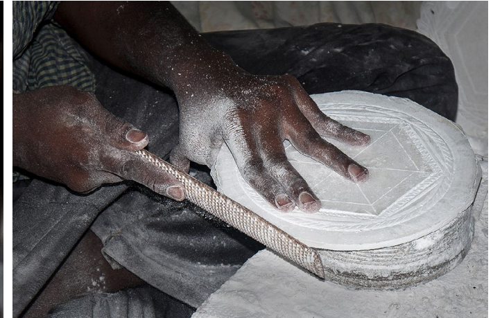
Edges of the article is shaped perfectly by filing.
