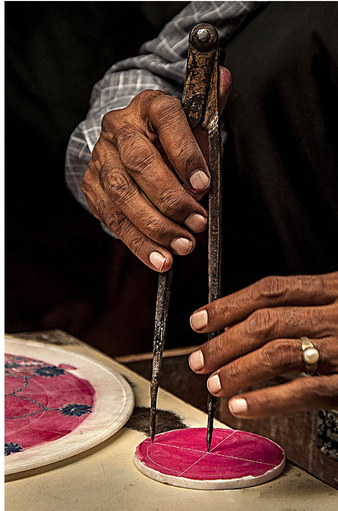
With help of divider the distance and radius of the design is measured and marked.
