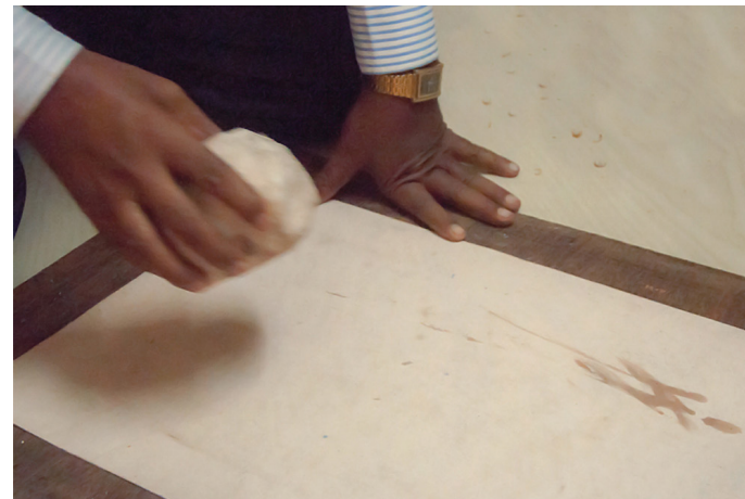
Chikna stone is rubbed to give shining.
