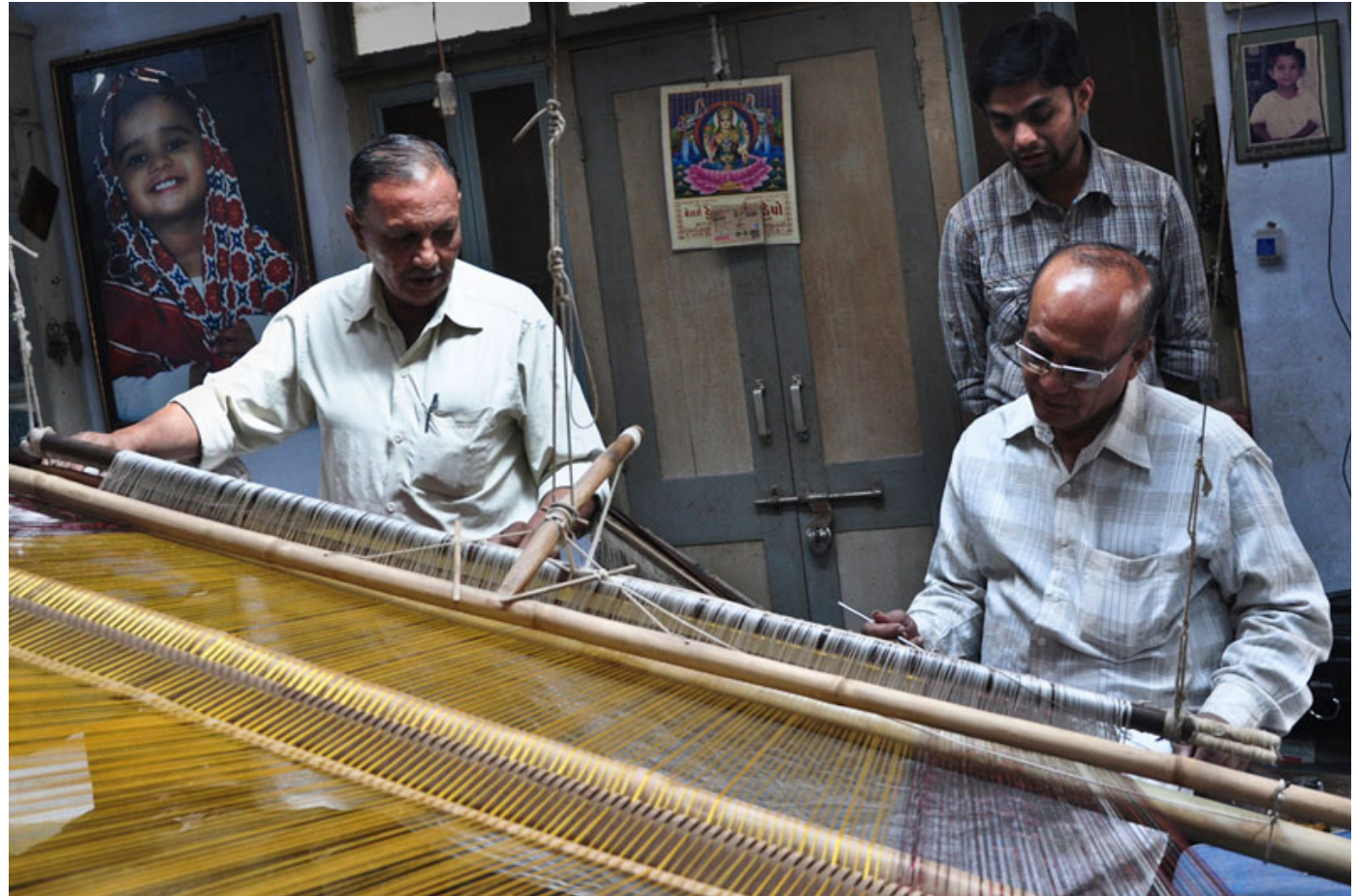
The warp is attached to loom and the weaving is begun.
