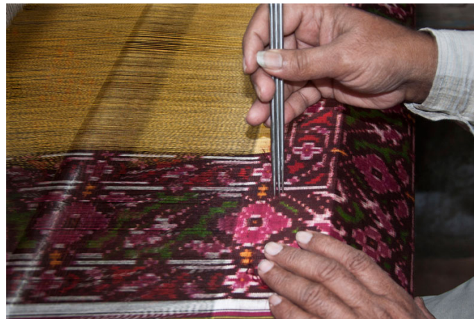
To consume time craftsmen use three needles at ones to cover more threads together.
