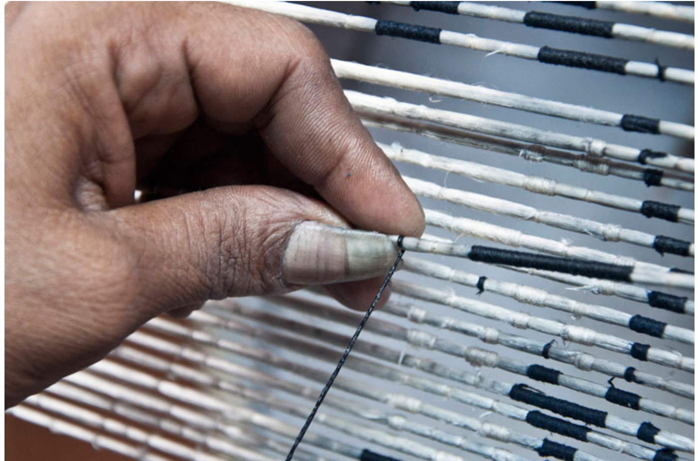
Design patterns are marked on the yarn which is tied with cotton thread soaked in water.
