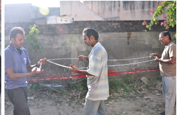
The plain color dyed thread is basically added in the ends to weave as borders.
