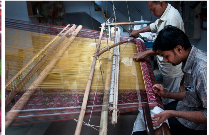
Weaved patterns are arranged properly with the help of a needle.
