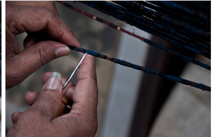
Sharp needle is used to remove the tied threads after dyeing.
