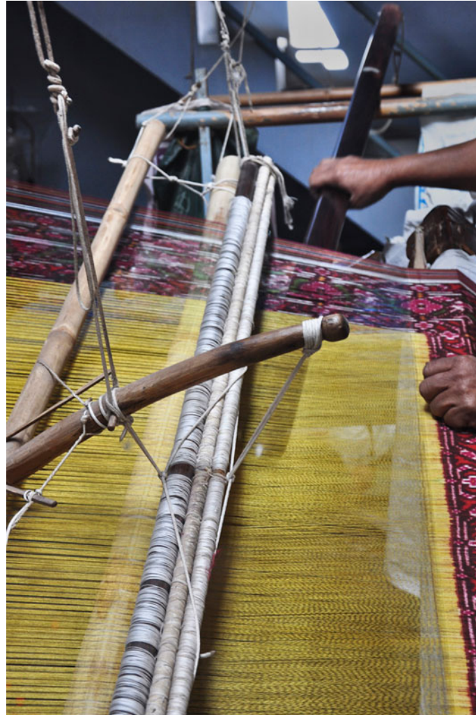
Rosewood rod is used as hand beater to weave the saree.
