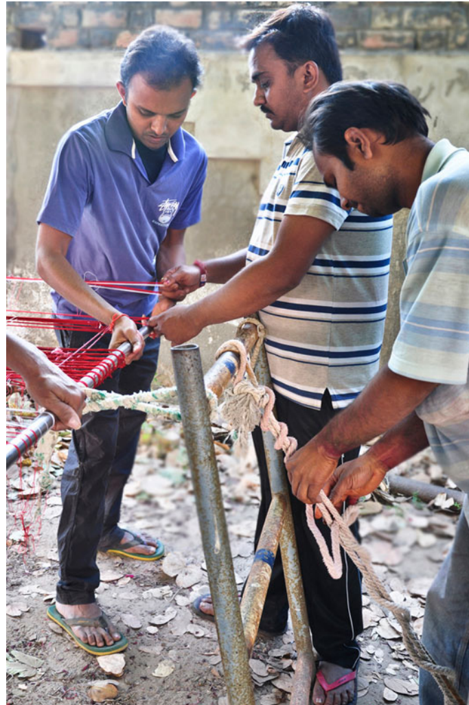
The dyed yarn is arranged to an iron pole for warping process.
