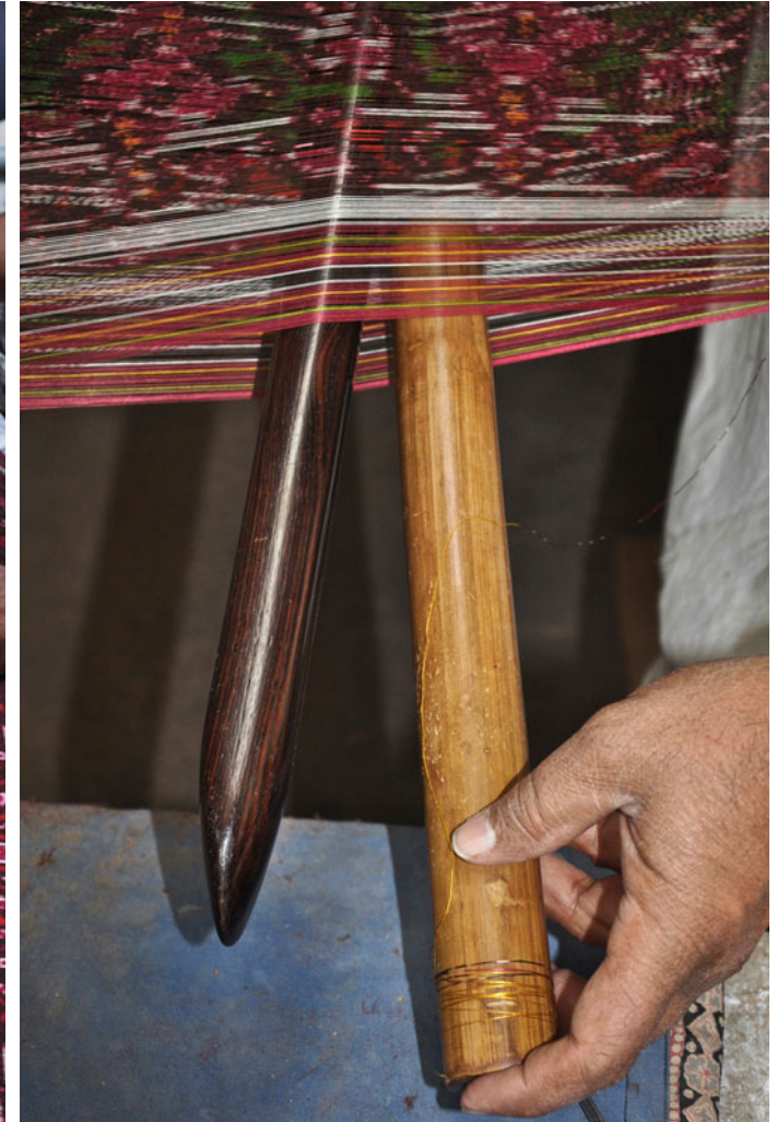
Bamboo shuttle is used to interlock the thread while weaving.
