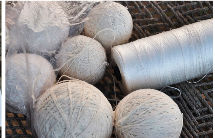
Cotton thread is soaked in water and tied on the warp to form the design in tie and de process.
