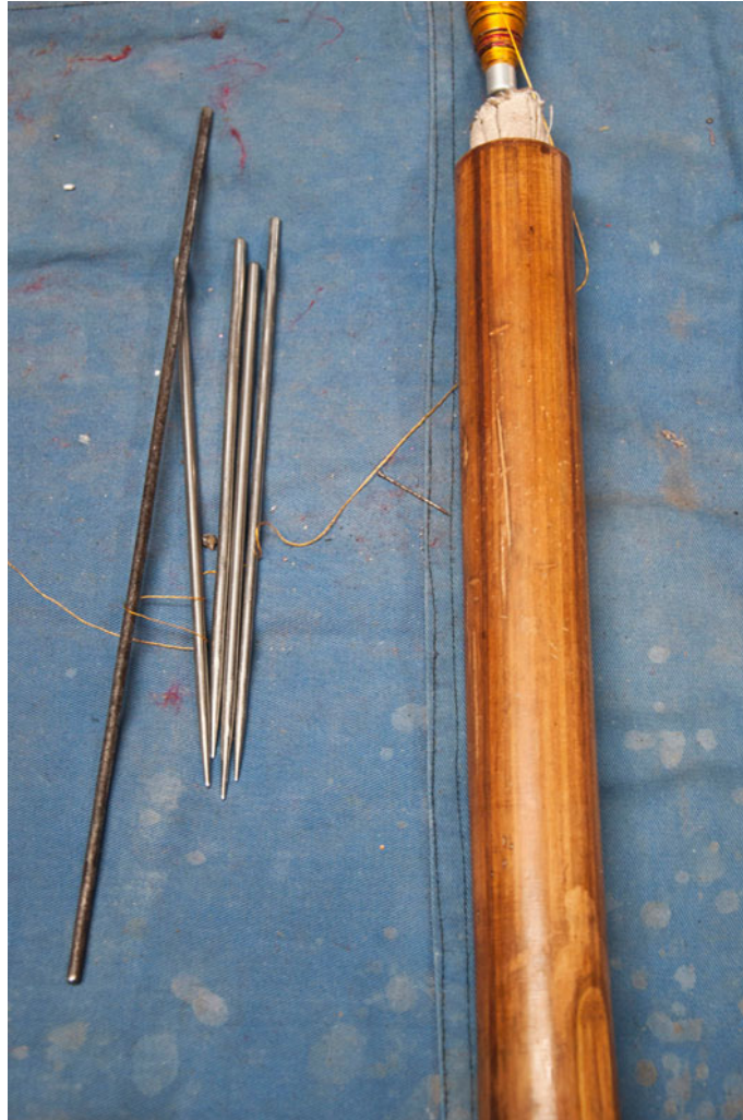
Iron needles are used while weaving to arrange the design patterns in order.
