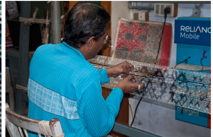
To color the tied area the threads are removed and areas which are colored and dyed again in different color.
