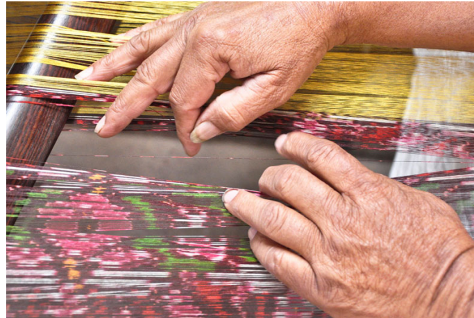
The warp is checked in timely intervals for breakages and corrected.
