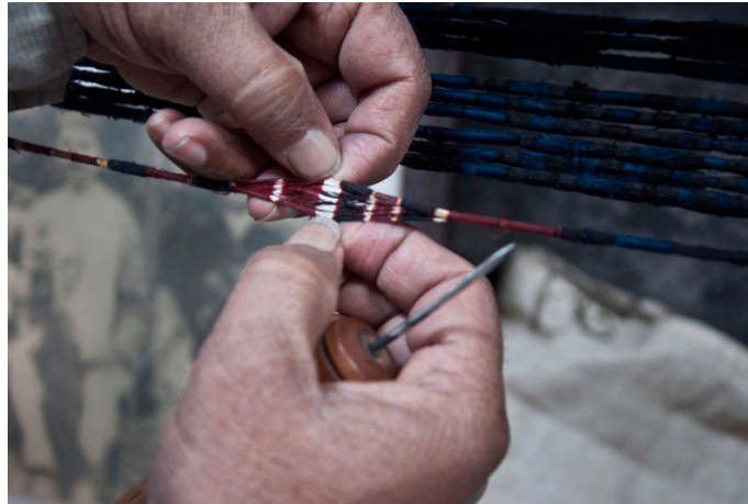
The process is repeated till the required number of colors to be dyed.
