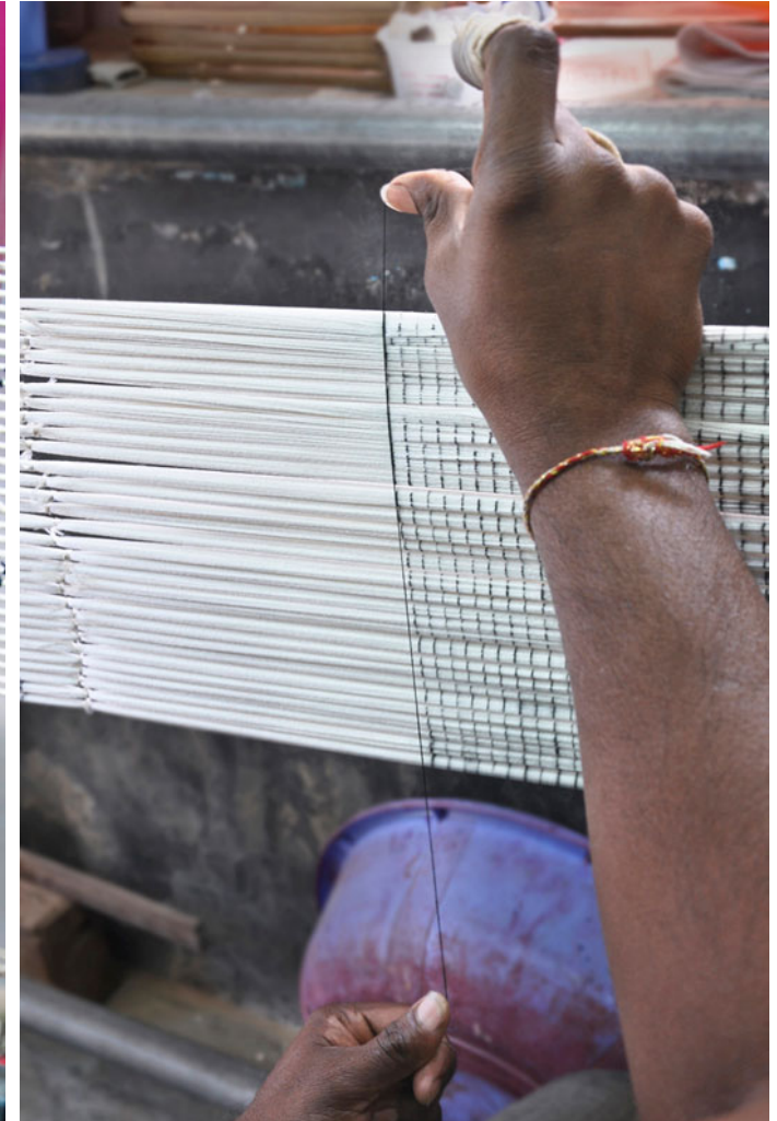
The inked thread is used to mark the designs on the yarn.
