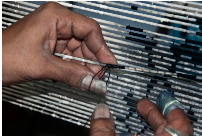
When dyed the exposed and untied area absorb the color.
