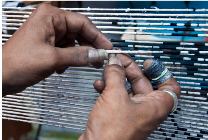
The markings are tied with cotton thread soaked in water.
