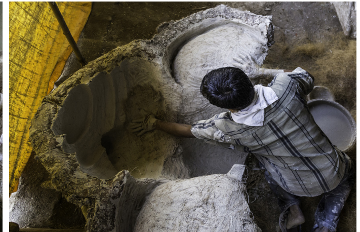
Artisan filling the mould with Plaster of Paris mixed with hay.
