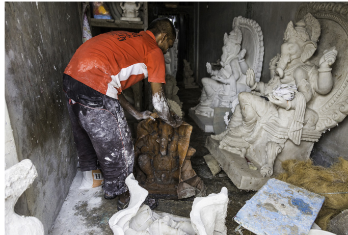
Removing the latex mould.
