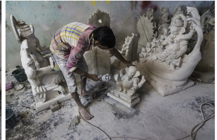
Painting with POP using a spray gun to fill the pores.
