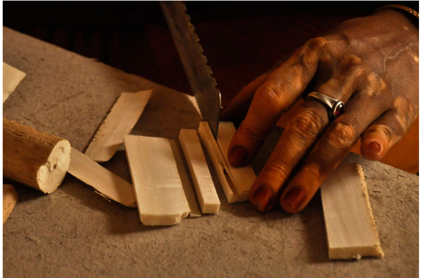
Pith is cut into different size shapes according to the design of the product.
