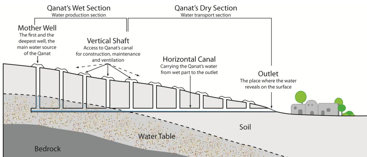
Figure.1 Schematic section of a Qanat (drawn by the author)
