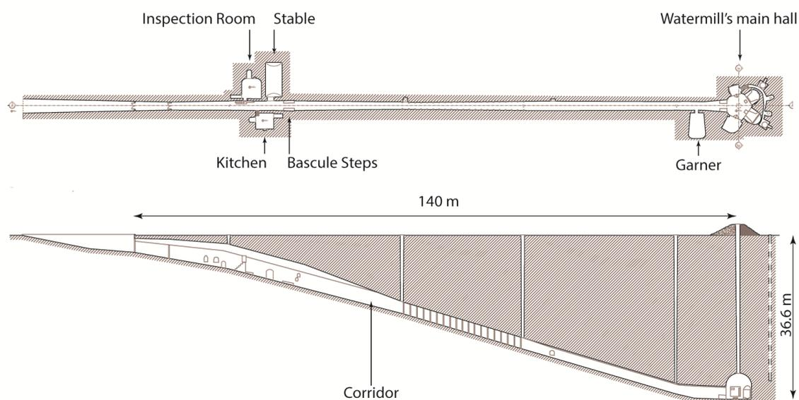
Figure.4 Plan and section view of Mohammadabad double-stone watermill (redrawn by the author)
