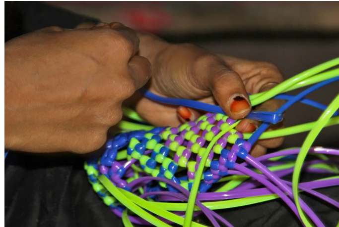
Plastic wire is looped and another wire is inserted into the loop and pulled out forming the knot.
