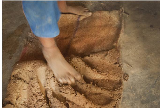
Clay is mixed thoroughly to ensure uniform consistency.
