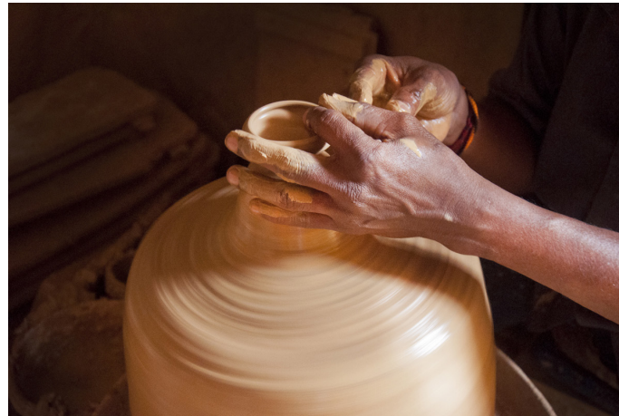
Walls are pulled upwards from the base for depth.
