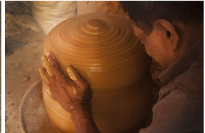
A big lump of clay is then centered on the Electric Potter's Wheel.
