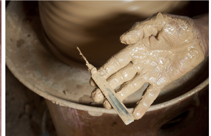
Wooden tool with a sharp iron needle used in cutting and shaping the clay while rotating.
