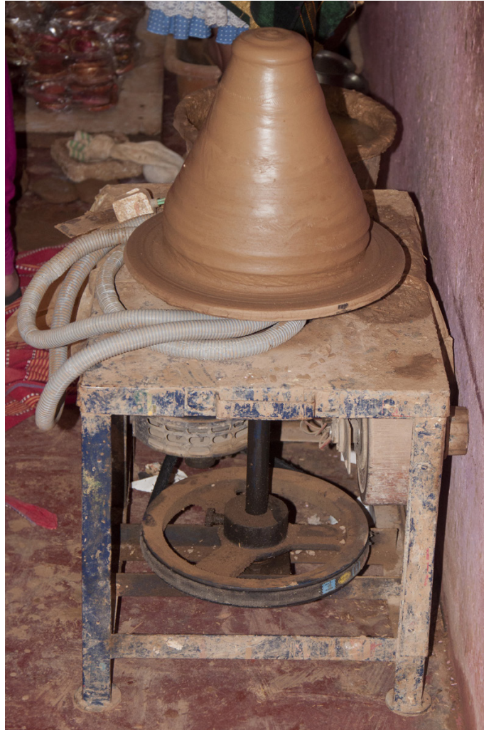
Electric Potter's Wheel used to shape the pots and lamps.
