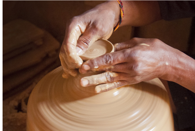
A flat base is made first, to further give the required shape.
