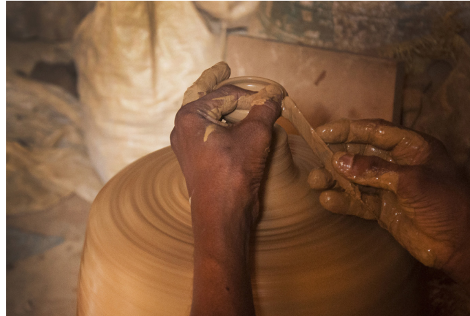
A sharp wooden tool is used to create the accurate shape.
