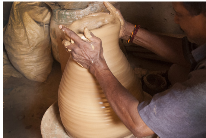
While turning process clay is lifted up to make a pointed shape from which the craftsmen can start shaping.
