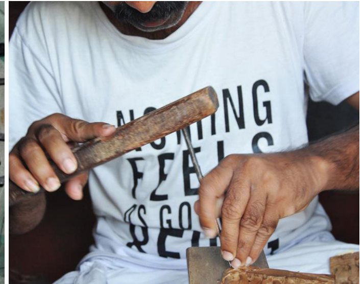
Wooden mallet and chisel is used in carving process.
