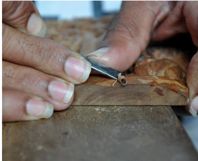
The excess wood is removed as per marked design.
