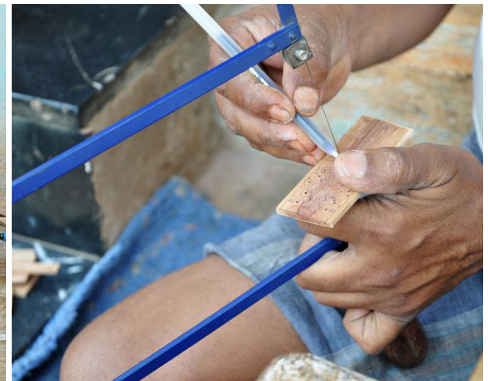
A coping saw is used to cut intricate external shapes.
