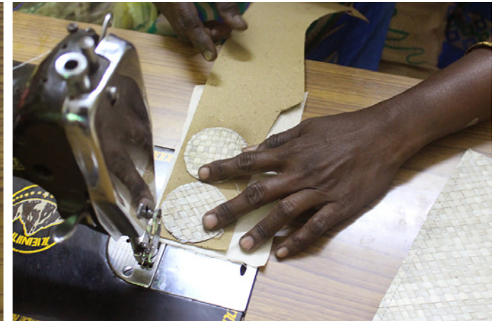
Spheres are stitched with cloth and cardboard to give strength.
