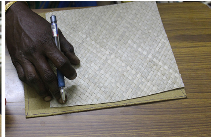
Cardboard is been marked and cut keeping mat as the reference.
