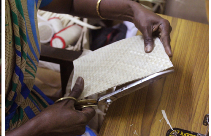
Pine mat is cut as per the cardboard measurement.
