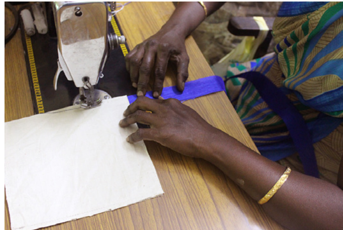
A blue color cloth is stitched to give outline of the pouch.
