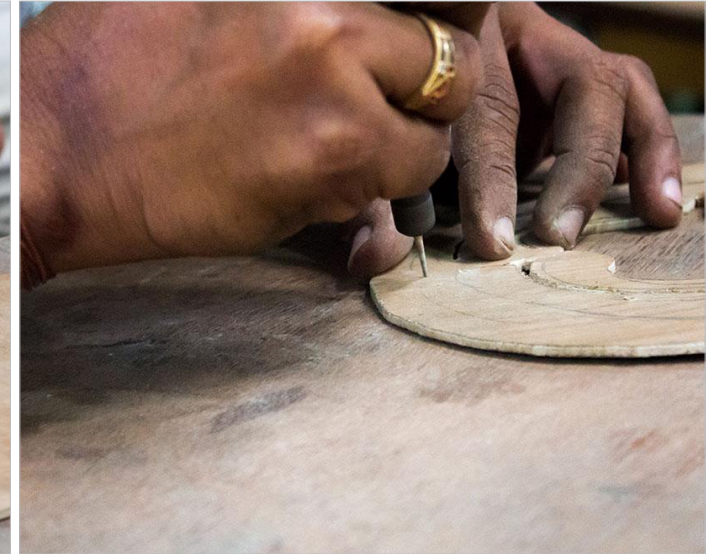
Using Dremel tool highlighted hair in the head portion of the plywood sheet is drilled.
