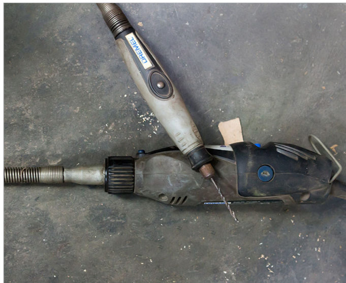
Dremel Tool - Used for cutting, grinding, sanding, buffing and shaping materials.
