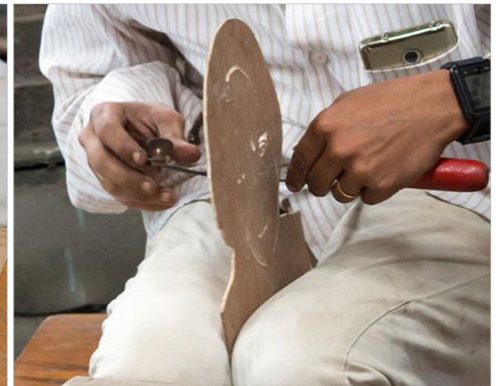
To cut down below the Eye Bag of the celebrity, plywood sheet is turned upside down and using the coping saw it is cut.
