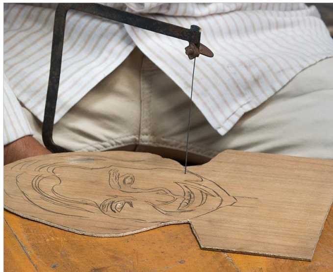
With the help of coping saw excessive face portion is cut down.
