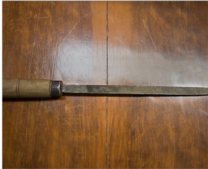
Fine File - Used to remove fine amounts of material from workpiece.
