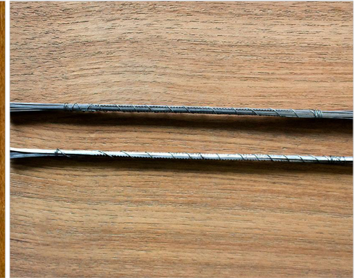
Blade strips - Used to make fine cuts in between ply-woods.
