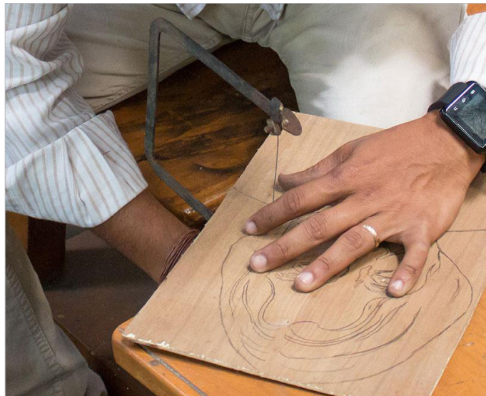
Using a coping saw, apart from the sketch impression excess of plywood sheet is removed.
