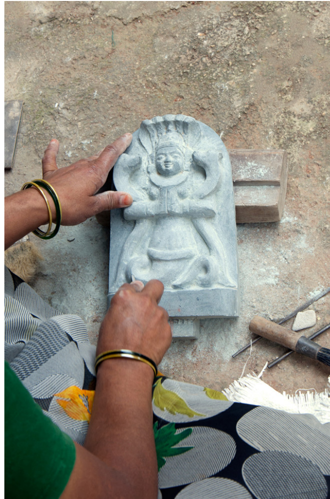
Artisan is minutely filing the precise shape to smoothen the surface.
