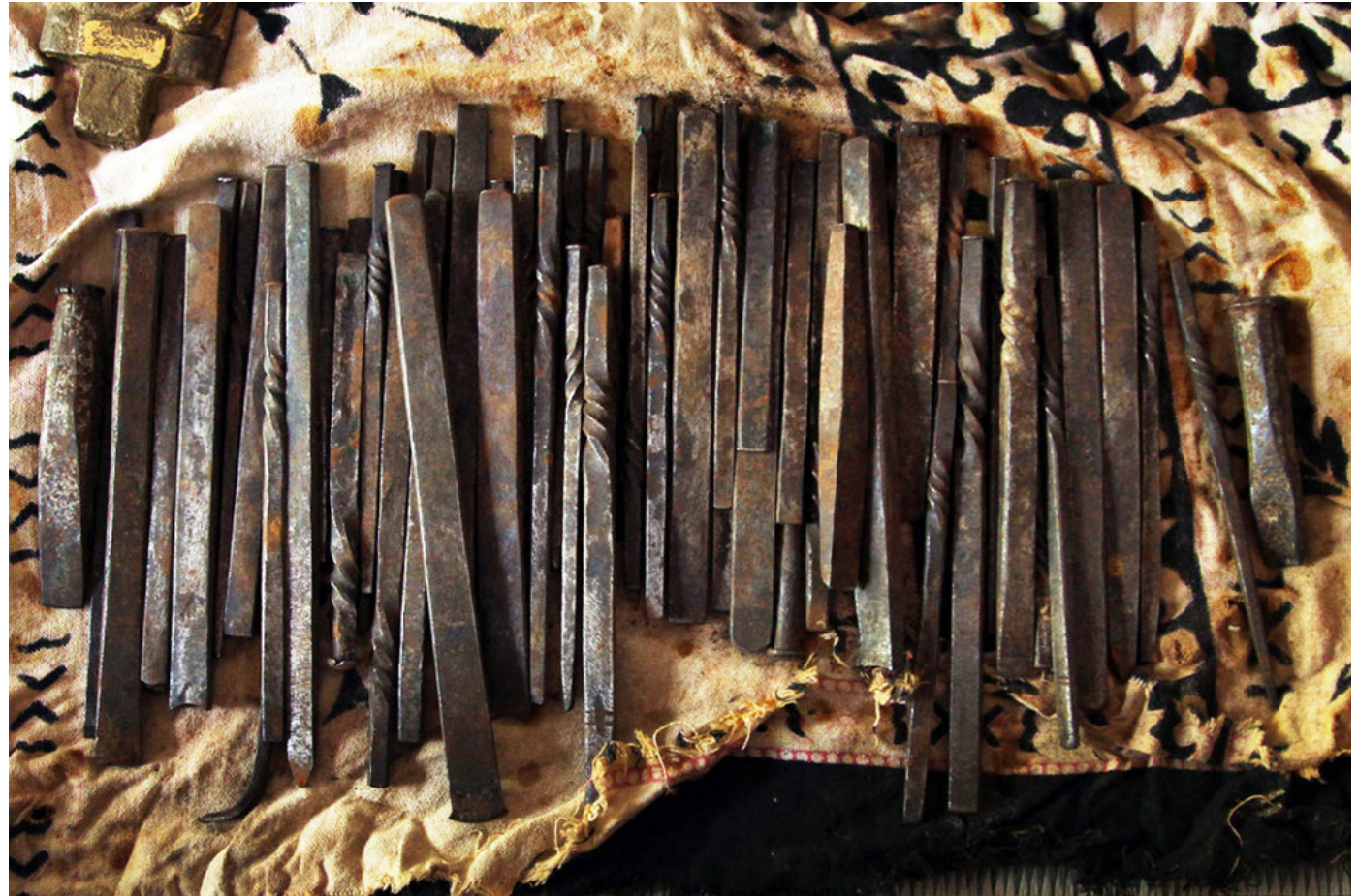
Chisels of various sizes and shapes which is used in carving the stones.
