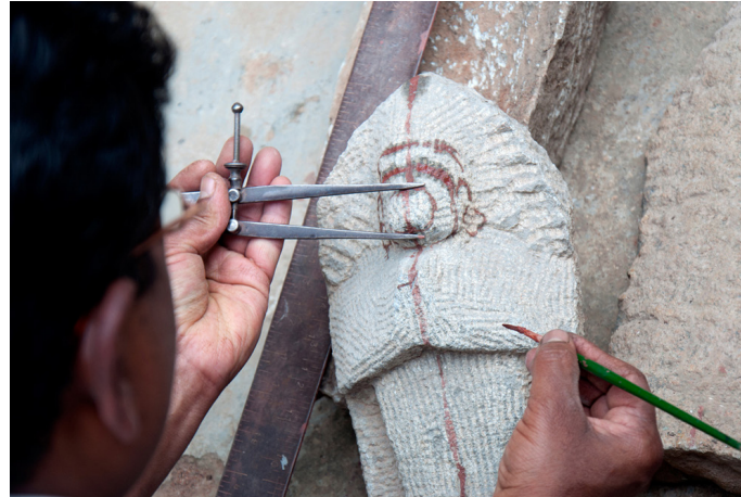
Divider caliper is used to measure the distance of the sculpture and mark them for carving.
