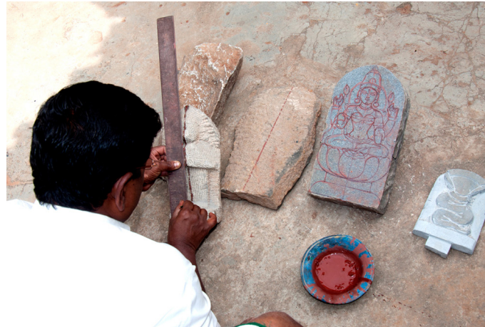
The process of dividing the raw stone into equal proportions to carve out the god and goddess.
