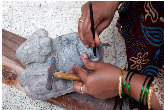
The markings are outlined on the stone with the help of a flat chisel.
