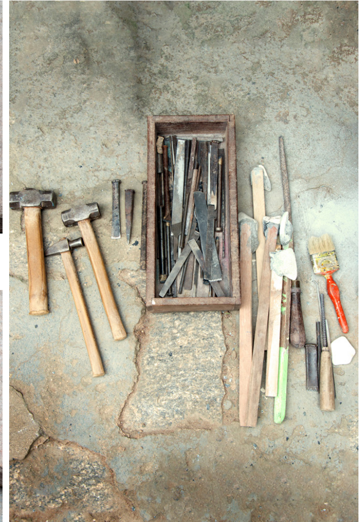
Hammers of various sizes along with chisels and brushes are used in carving.
