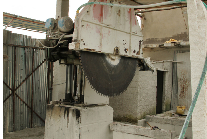
The huge cutting machine is used in cutting of the stones.
