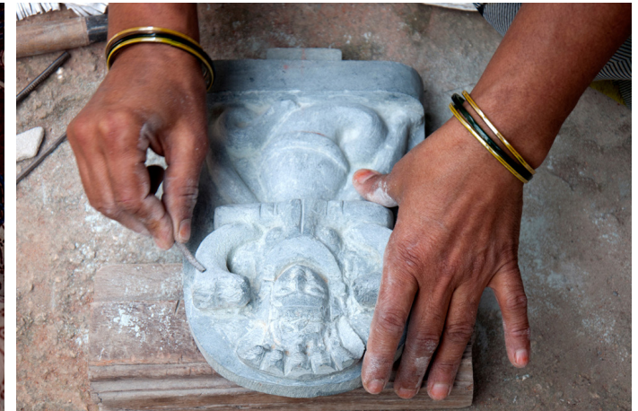
The final filing of the object to shape it into a smooth surface.
