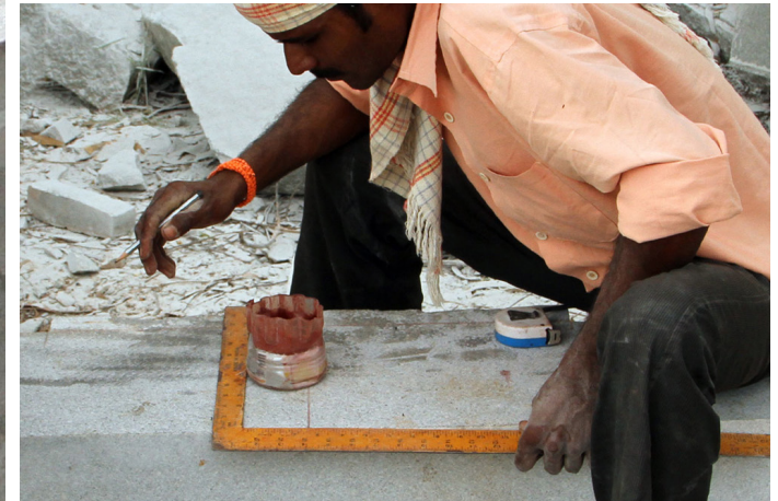
Artisan with the help of L shaped scale draws the straight lines.
