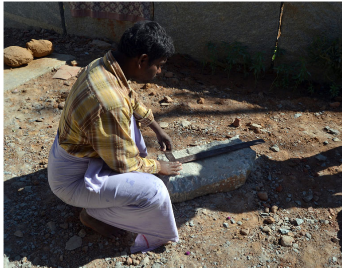
Large scale to mark the stone horizontally.
