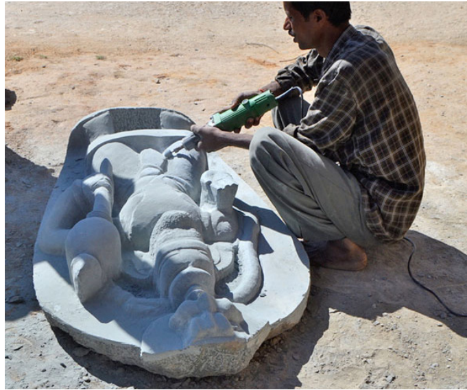
Die grinder to finish the area where the hand usually do not rich like curves and corners, in this machine the front stone can be replaced with the different kinds of stone.
