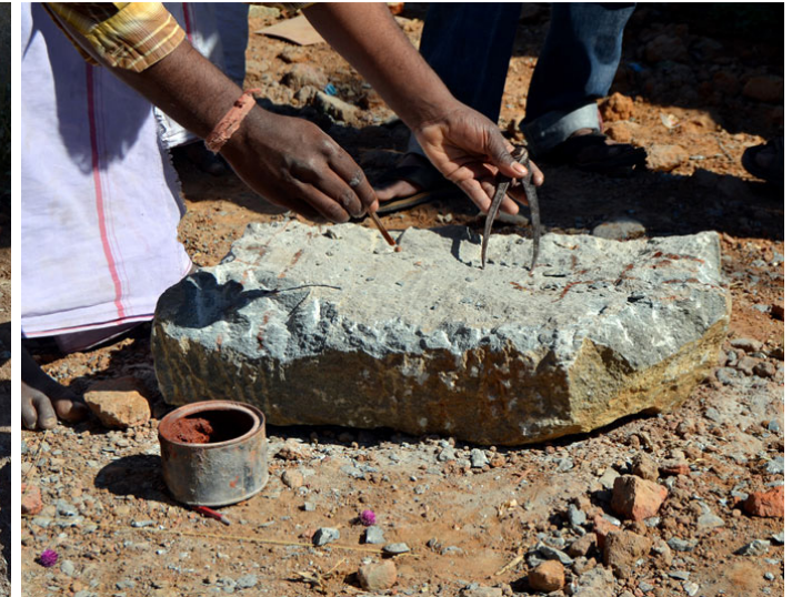
Radial compass to measure the diameter and to get the proportion of the sculpture.
