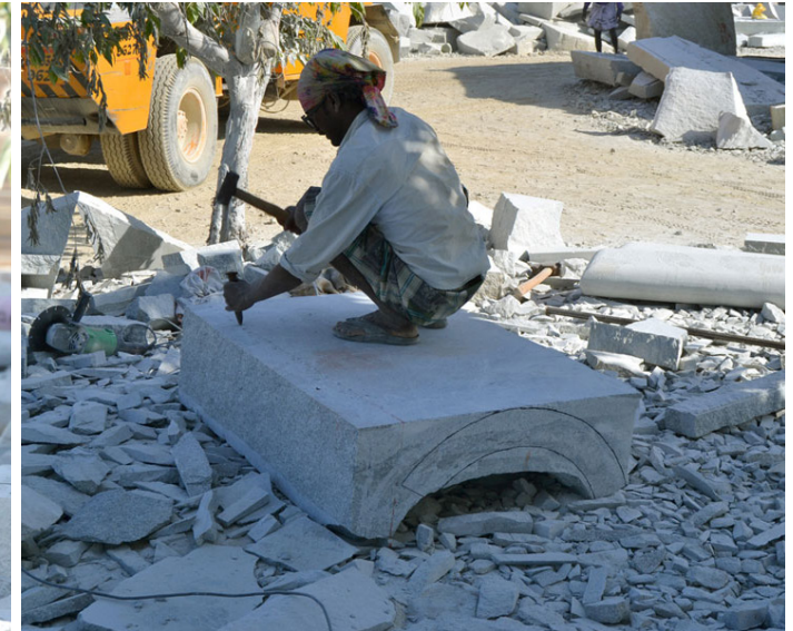
Round chisel of different size with a pointed tip to cut the stone.
