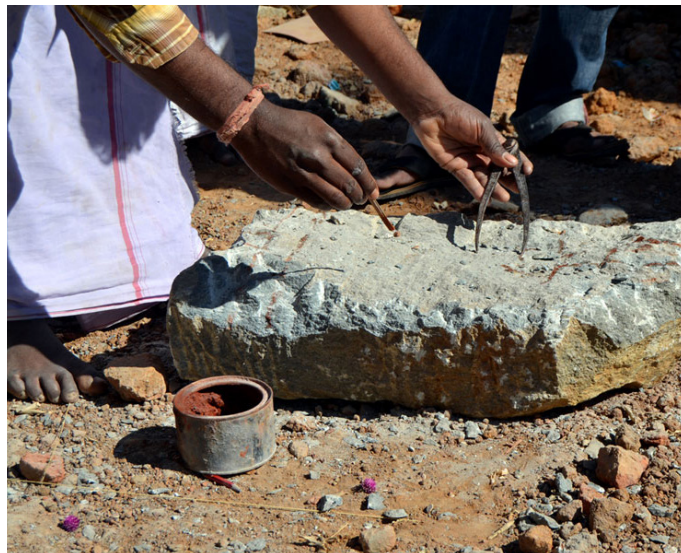
Radial compass to measure the diameter and to get the proportion of the sculpture.
