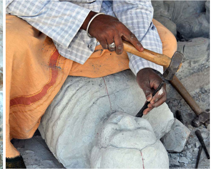
Flat chisel of different size with a pointed tip to cut the stone.
