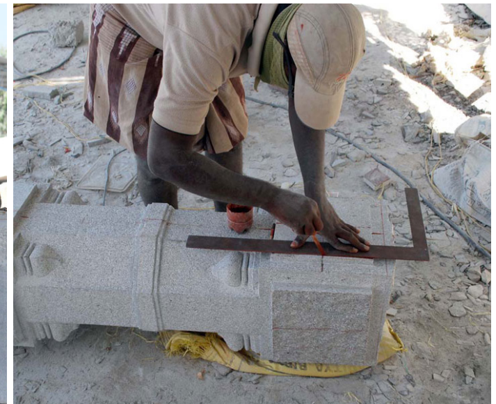
The master craftsman does the marking on the rough stone.
