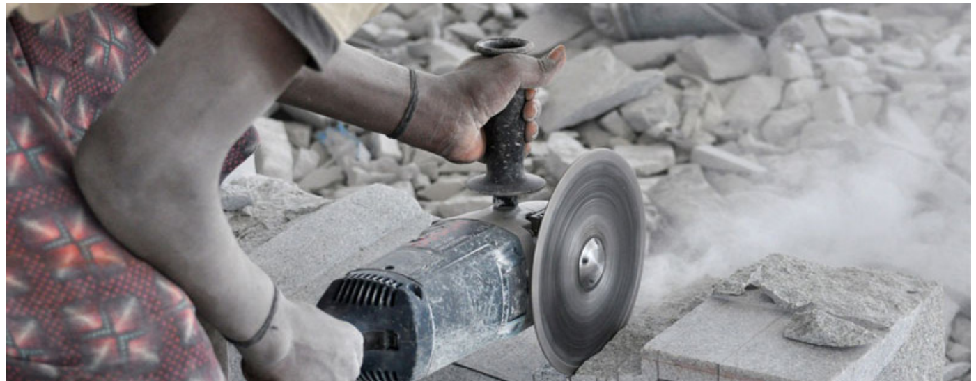
Small channel cutter to cut smaller surface.
