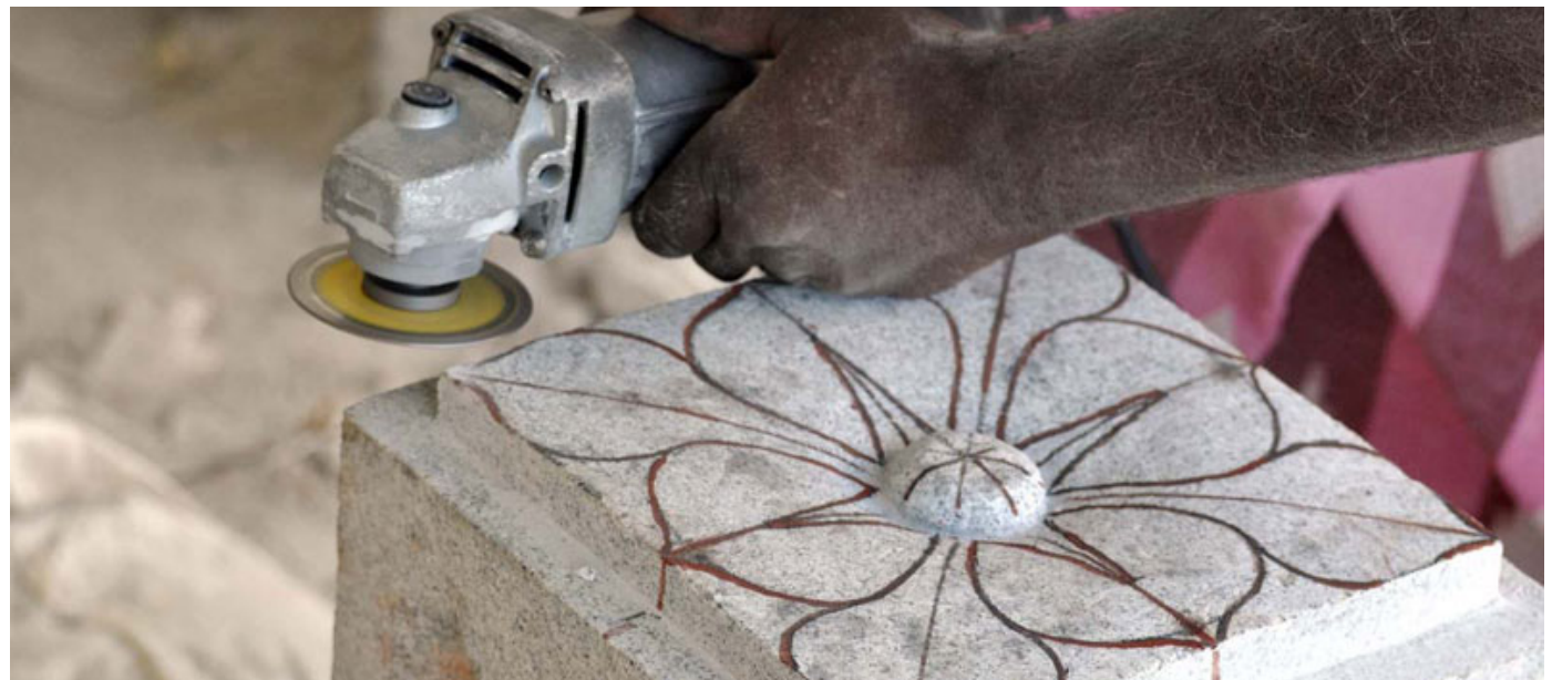
Stone filler, use to make the surface plane.
