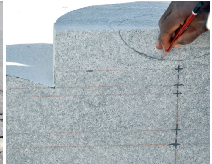
The master craftsman does the marking on the rough stone.
