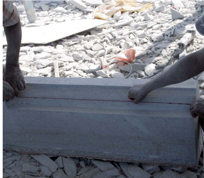
The master craftsman does the marking on the rough stone.
