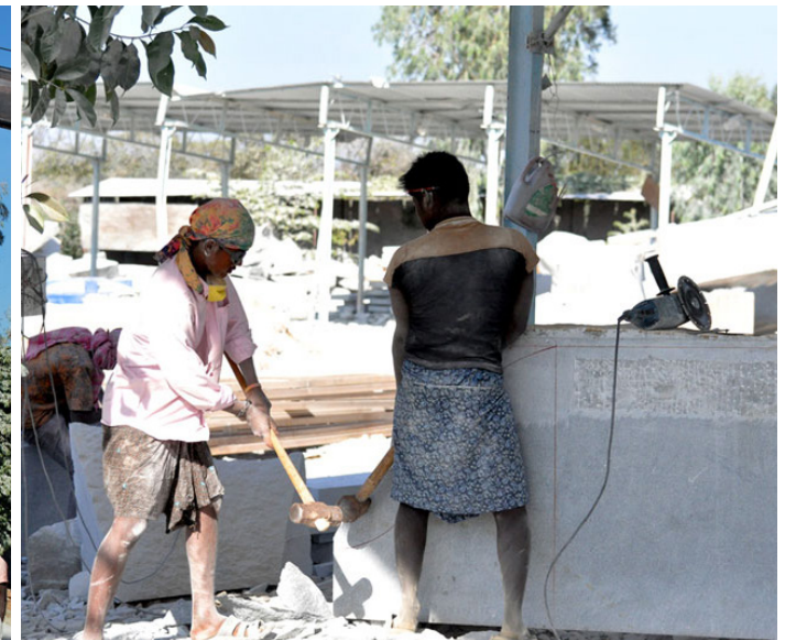
Hammer of different weight and size to cut the stone.
