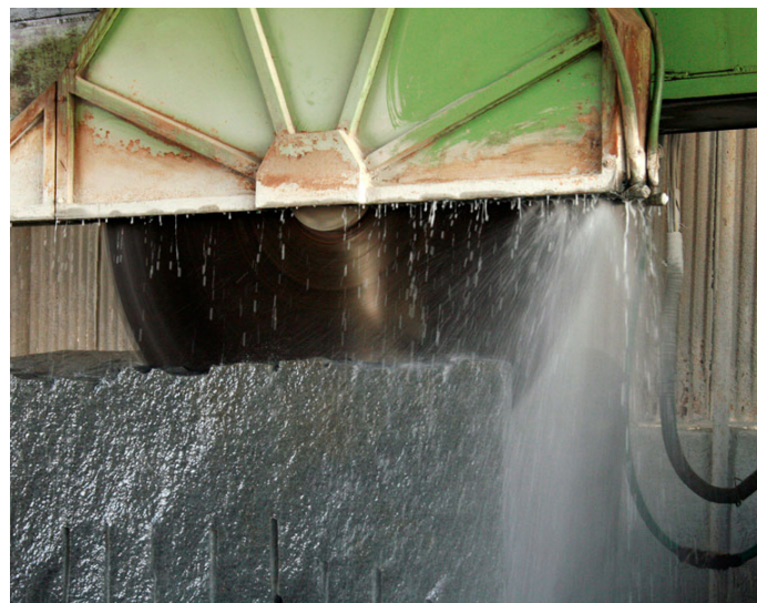
Bigger channel cutter to cut the bigger surface.
