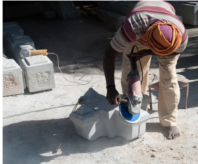
Stone filler, use to make the surface plane.
