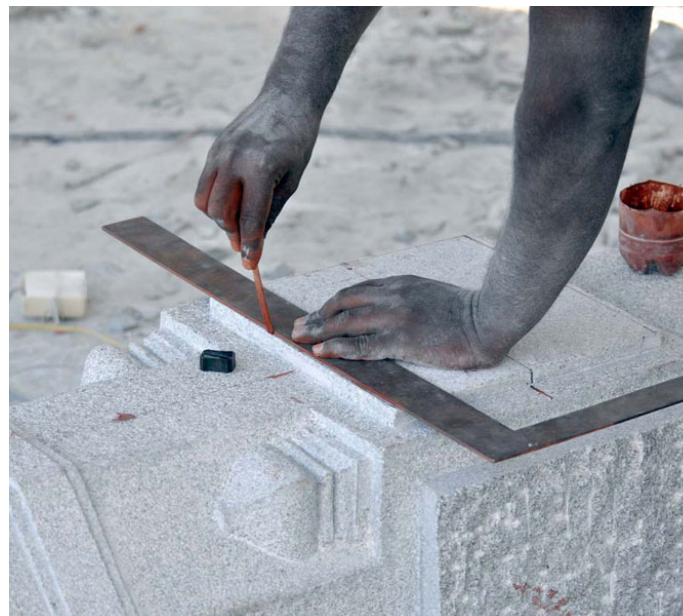
The master craftsman does the marking on the rough stone.
