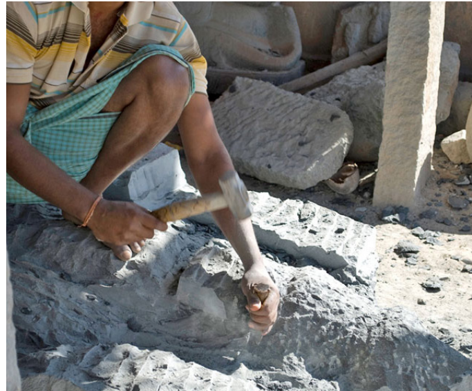
Round chisel of different size with a pointed tip to cut the stone.
