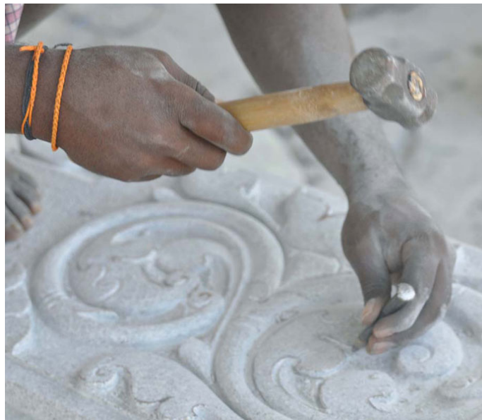
Round chisel of different size with a pointed tip to cut the stone.
