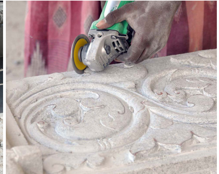
Stone filler, use to make the surface plane.
