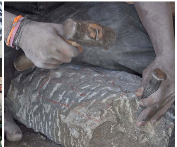
Round chisel of different size with a pointed tip to cut the stone.
