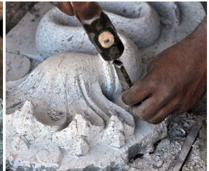
Flat chisel of different size with a pointed tip to cut the stone.
