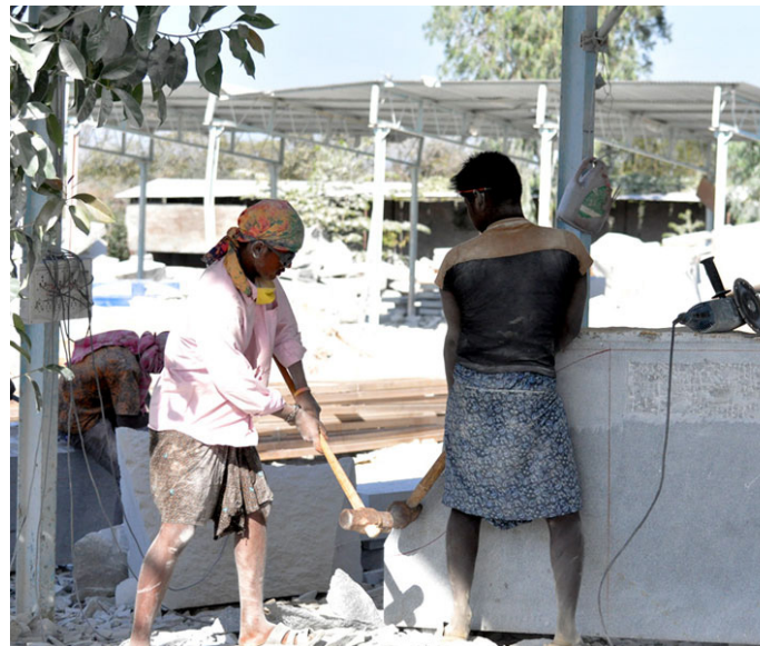
Hammer of different weight and size to cut the stone.
