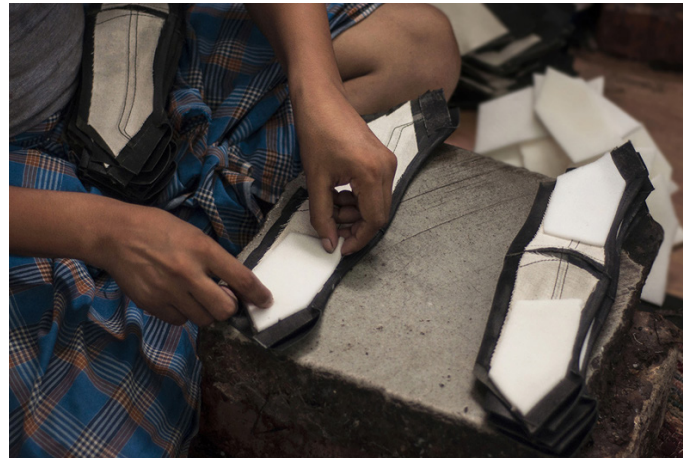
Sponges are measured and placed in the proper positions.
