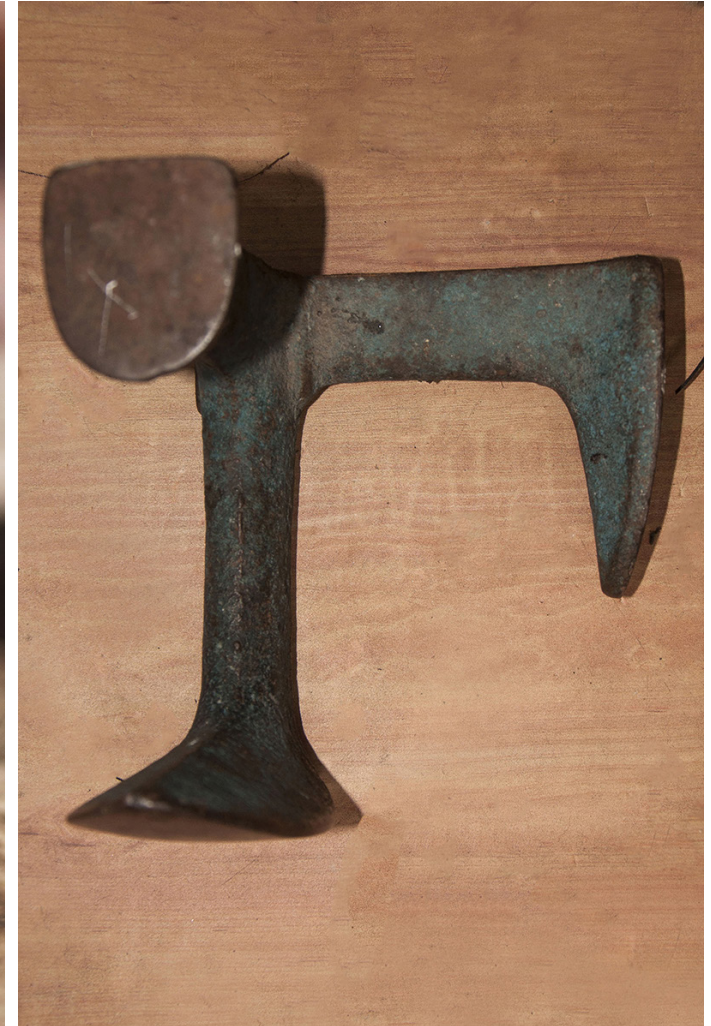
Antique Iron Shoe Cobbler stand used for hammering and repairing.
