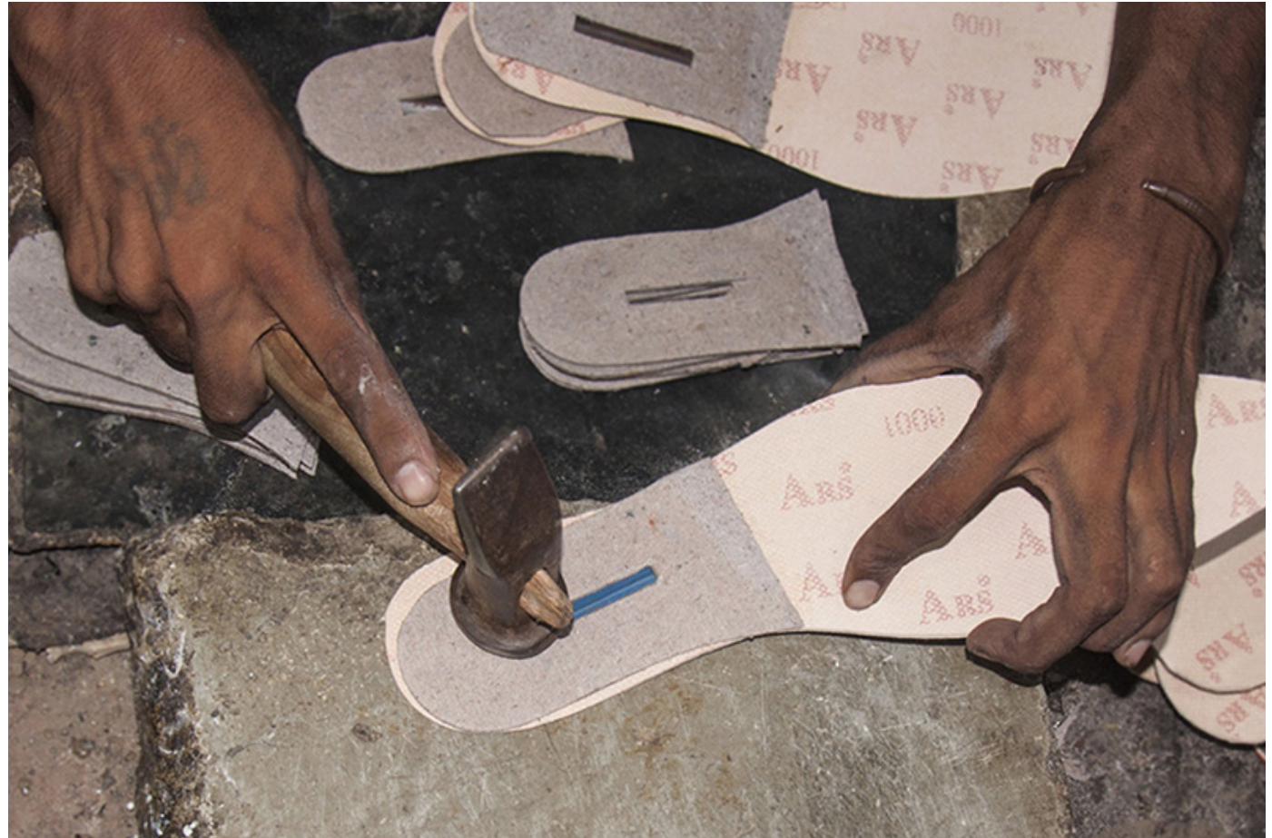
With the help of tack hammer shanks are set into places.
