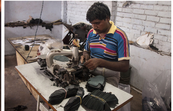
Craftsman cutting out the different parts of the leather shoes.
