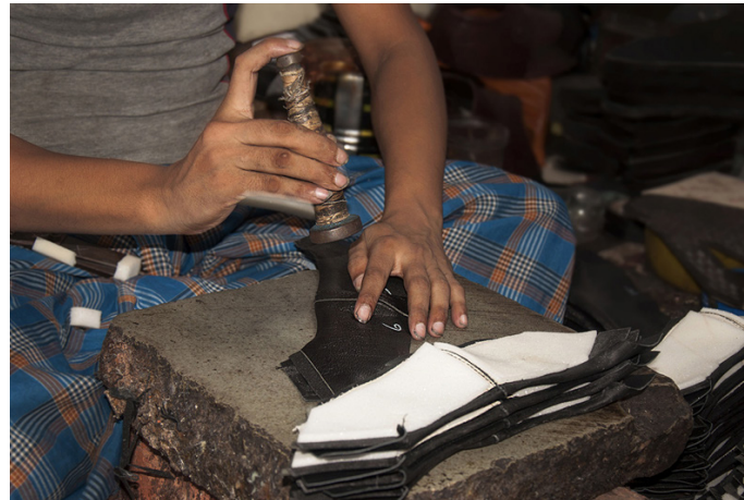
Raw hide mallets are used as hammers for stamping.
