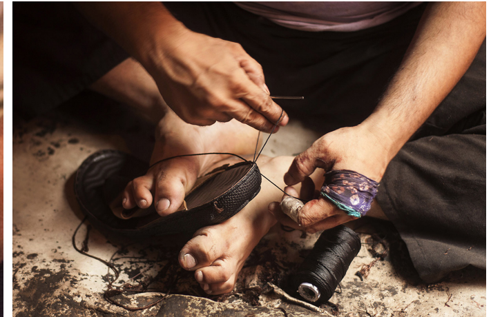
Stitching Awl is used to sew the parts of the shoe.
