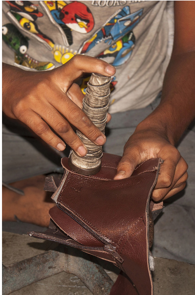
The sewed leather are stamped to flatten the stitches.
