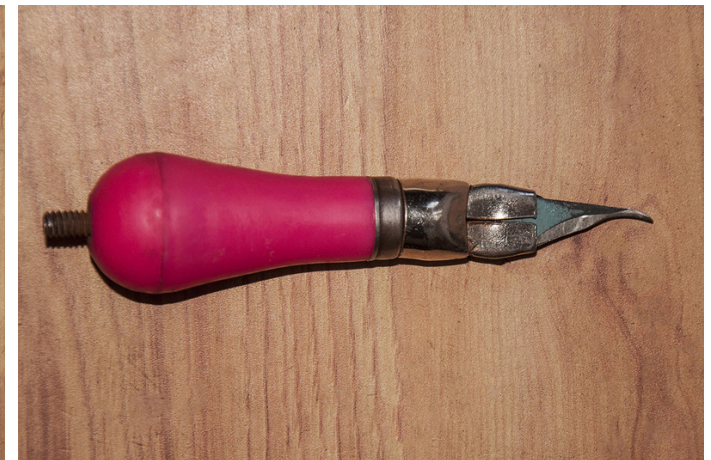
Stitching awl used for the purpose of sewing shoes.
