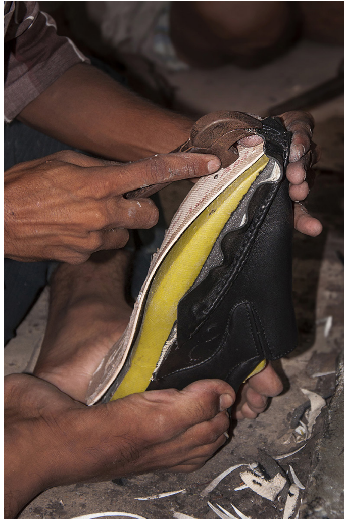
The leather parts are bend using shoemaking pincers.
