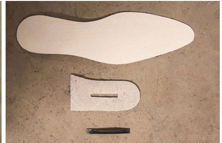
Inner sole and heel part of the shoe.
