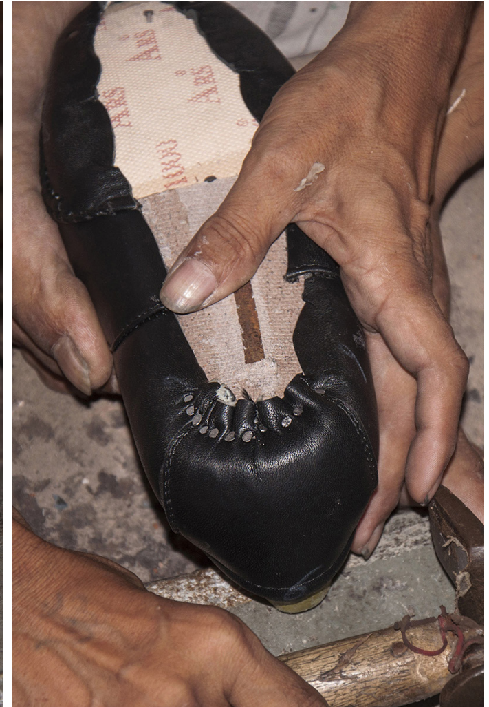
Metal nails attached to the insole and leather.
