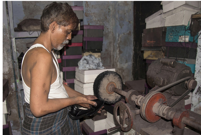
Buffing machine is used to remove excess polish from the shoes.
