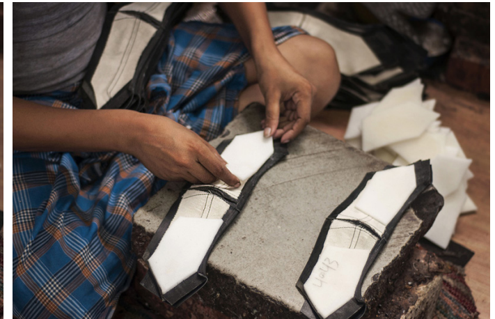
The sponge part is attached to the leather.
