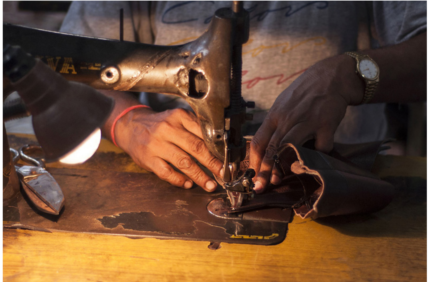
Sewing machines are used for sewing the leather.
