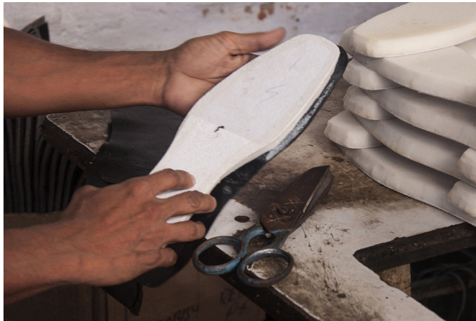
The cut sponges are attached to the insoles.
