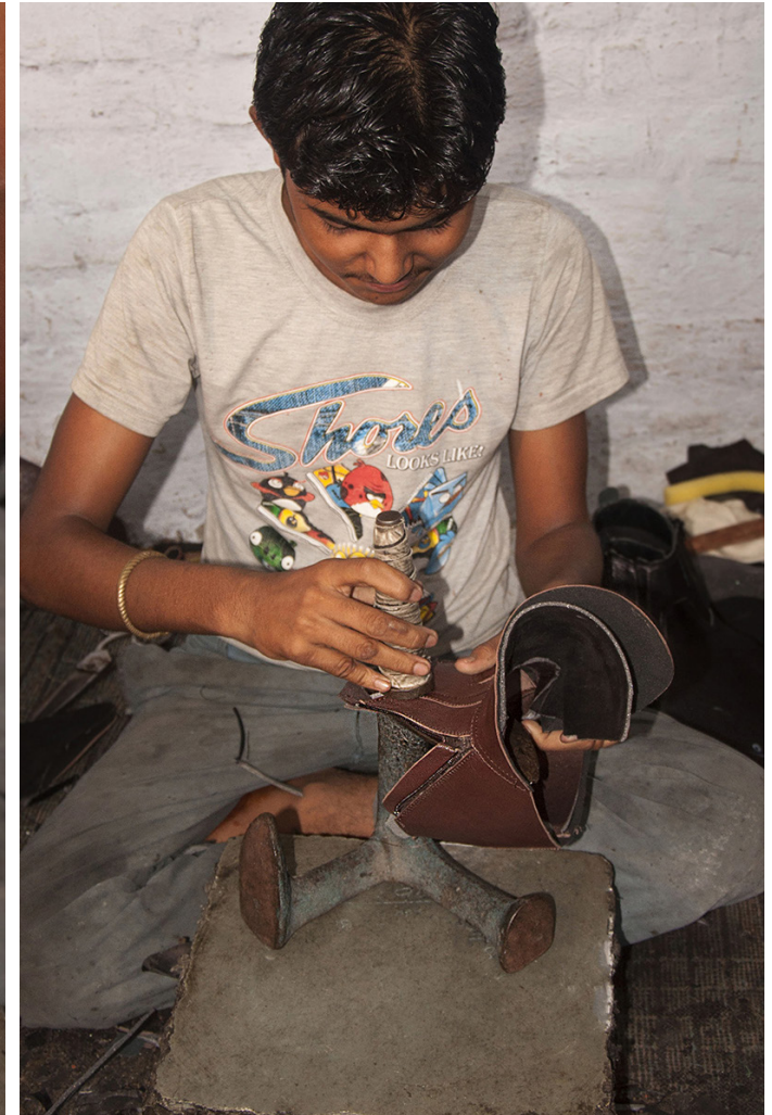
The upper leather part are placed on iron cobbler stand and stamped.
