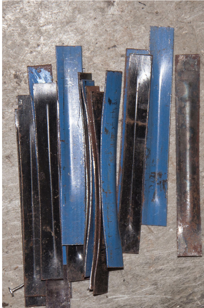
Metal strips (shanks) are attached to the insole to provide arch support.
