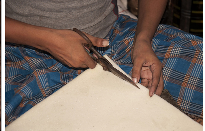
Thick sponges are cut into desired shapes.
