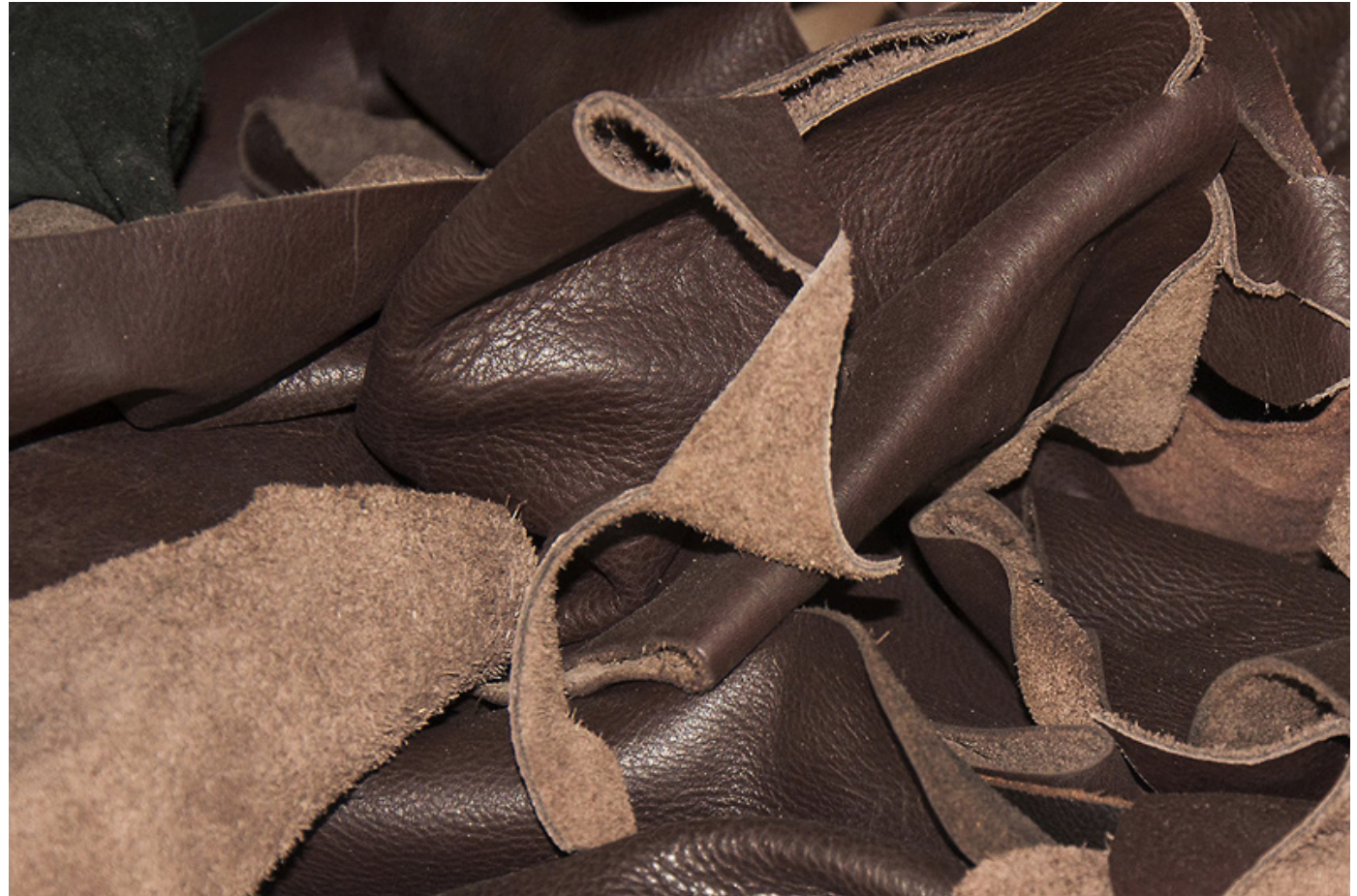
Cut out pieces of tanned soling leather is used for making shoes.
