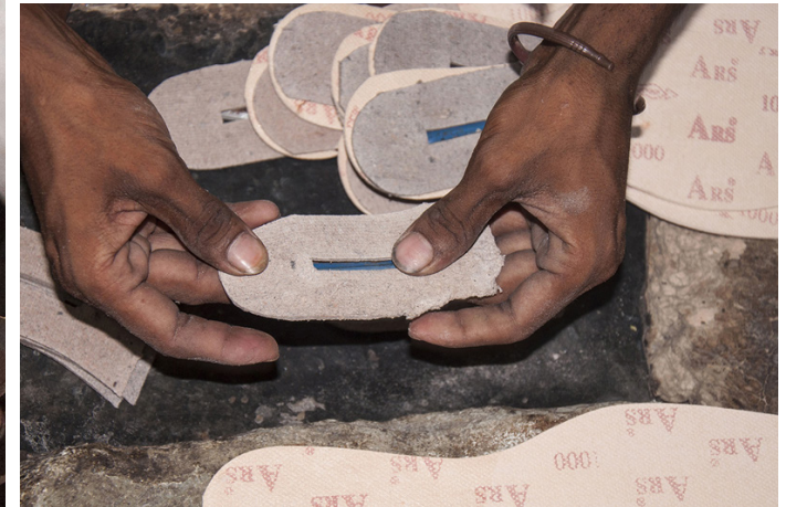
Metal strips (shanks) are glued with the insoles.
