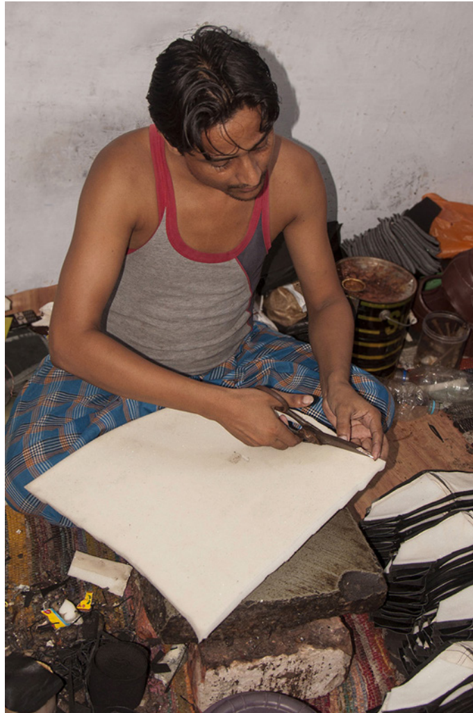
Leather sheets are cut into required shapes.
