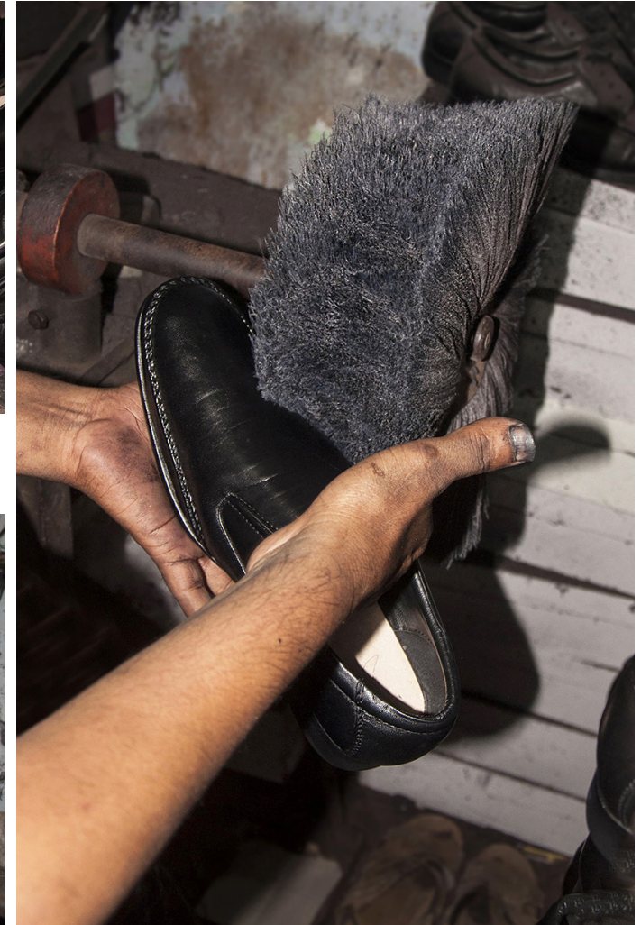
Buffing machines are often used for smoothing up the remaining polish into the leather.
