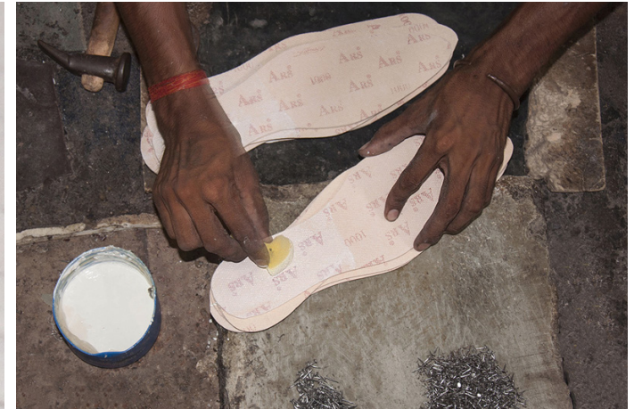
Glue is applied to the insoles.
