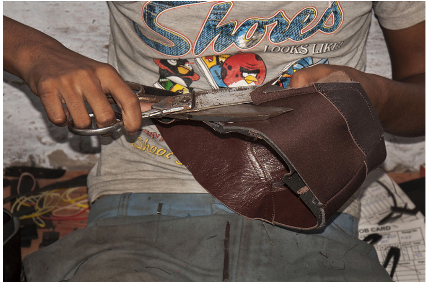
The unwanted leathers are scrapped out using scissors.
