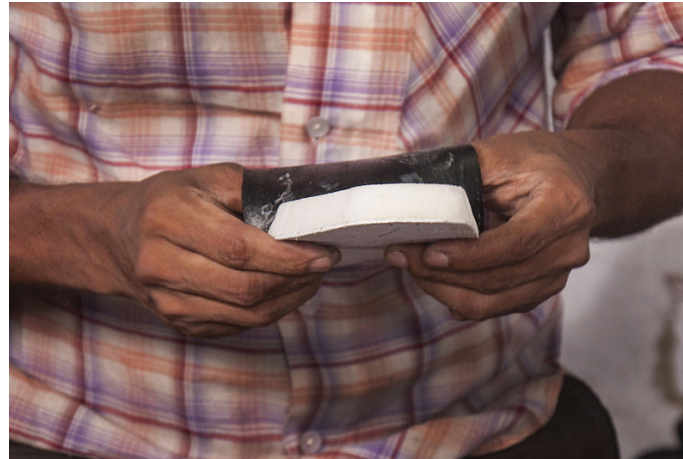
The insoles pressed hard to stick firmly with the sponge.
