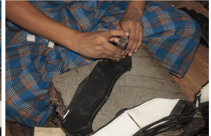
Mallets are used to make folds in leather.
