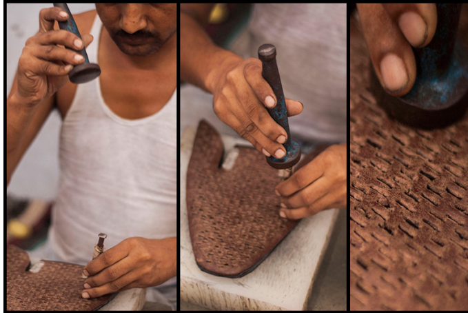
Skilled artisan involved in designing the vamp with Raw hide mallets.
