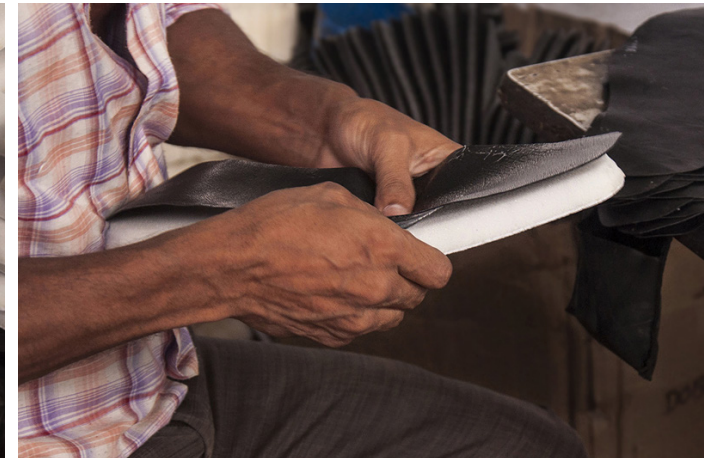
Artisan ensures that all sides of the sponges are firmly glued.
