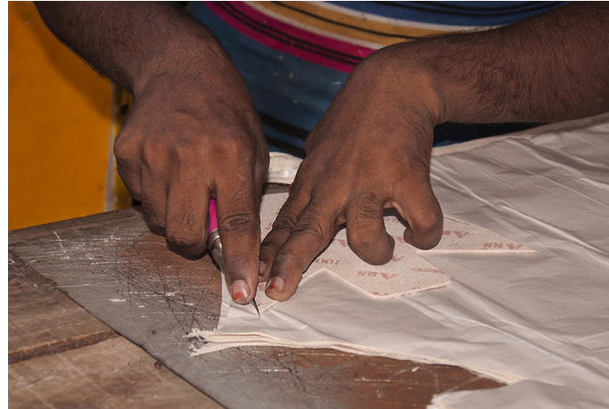
Craftsmen uses Stencils to cut out the leather.
