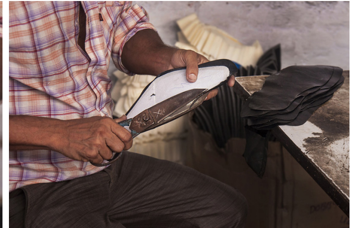
Unwanted leather parts are removed.
