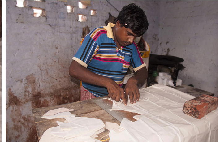
Different parts of the shoes like vamp, soles and heels are cut.
