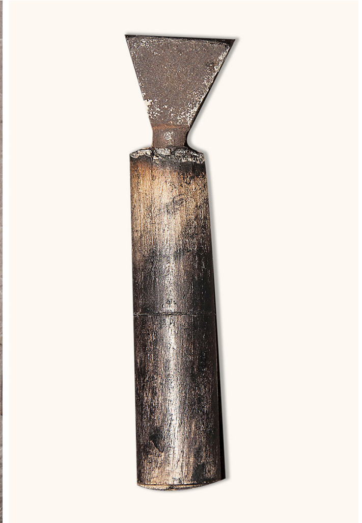
A shoe maker's Chisel.
