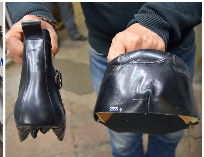
Difference between a machine-pressed and unpressed upper
