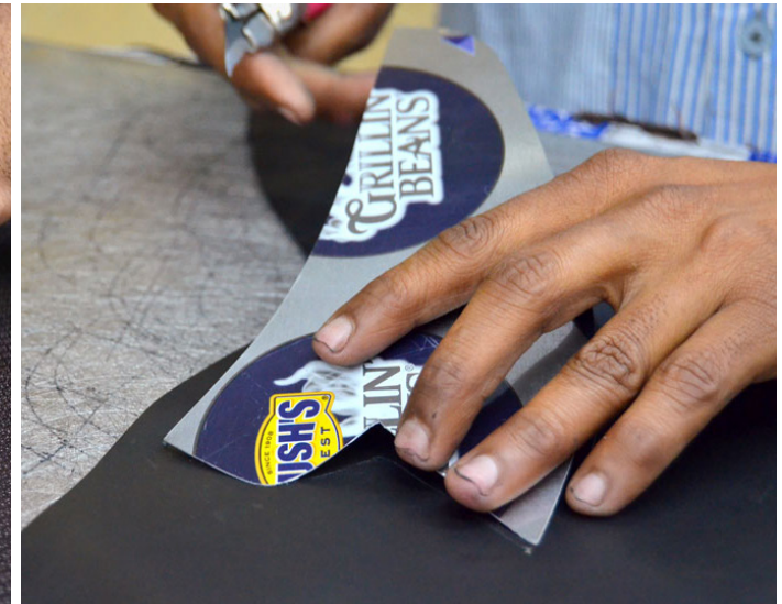
Tin stencil being used to cut the shapes in leather
