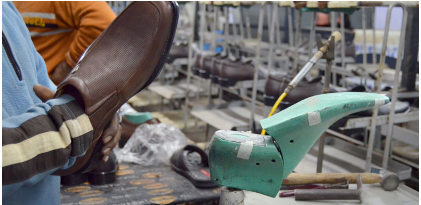
Last being removed from the finished shoe to be used in making other pieces
