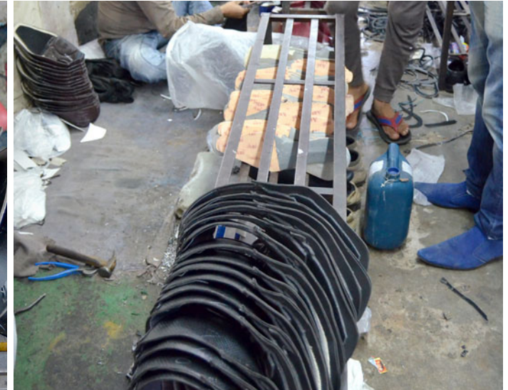
Uppers, numbered and stacked to be lasted
