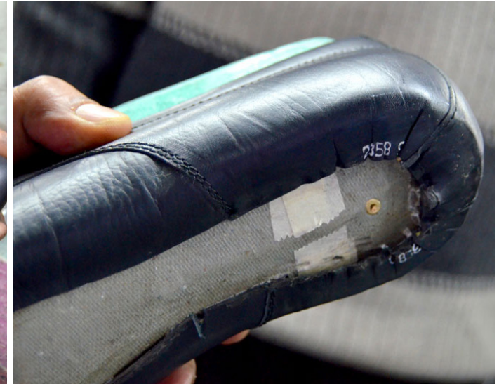
Parts of the upper glued to the surface of the insole visible at the bottom
