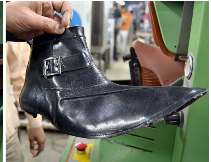
The machine that presses the upper
