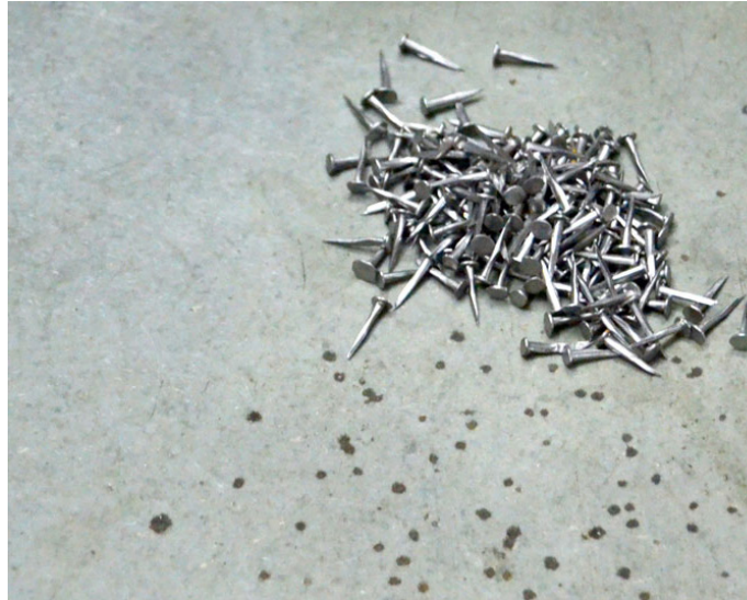
Nails (are used to fit the upper on the last for only the sample shoe, the rest of them are glued)
