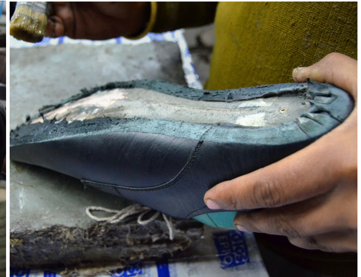
Parts being rubbed off to make the leather rough (called skiving)
