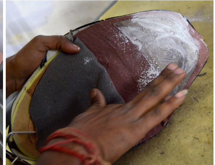
The patch being attached to the upper
