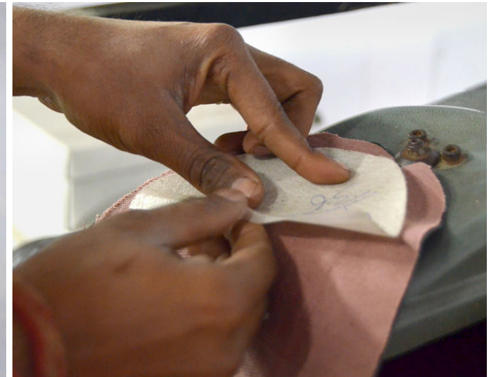
The patch being attached to the upper
