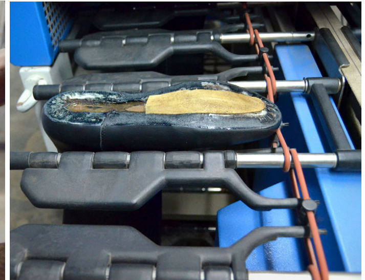
Machine that dries off the adhesive just right enough to stick well
