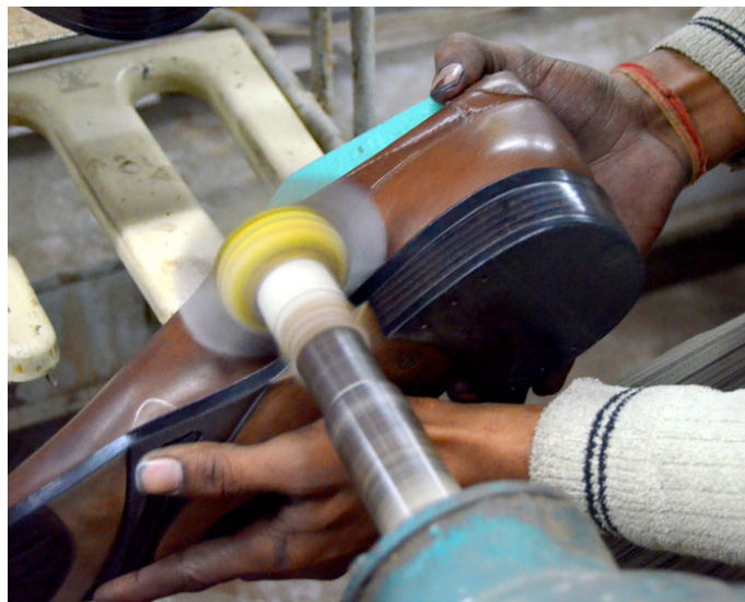
The heel and the edge of the sole being cleaned
