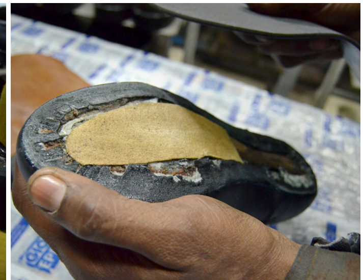
Sole being glued to the lasted upper
