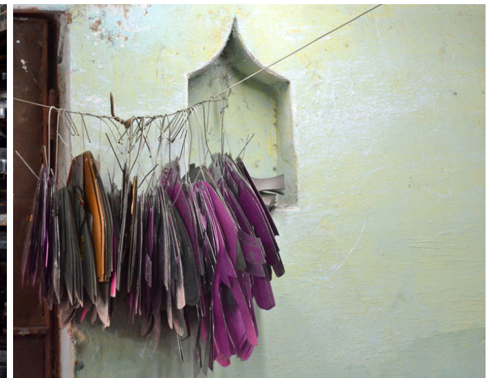
Tin stencils for cutting the shapes in leather
