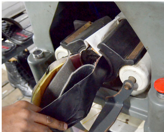
Upper being pressed in the machine for giving it better shape
