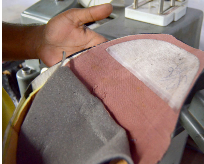
The patch being attached to the upper
