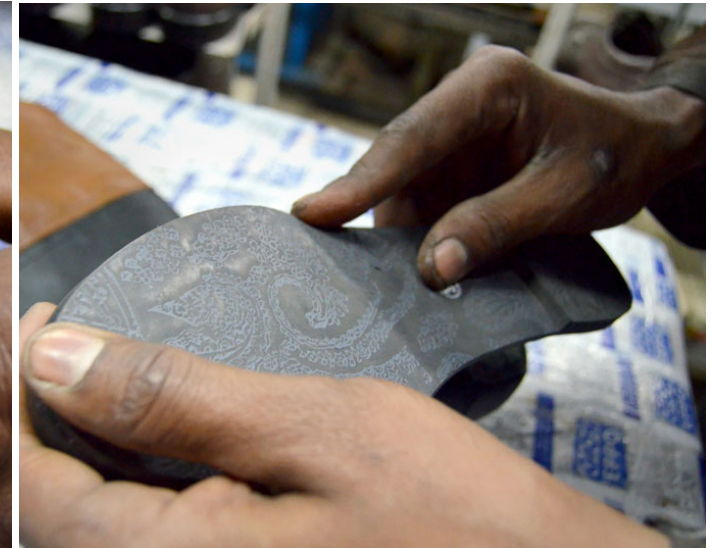
Sole being glued to the lasted upper
