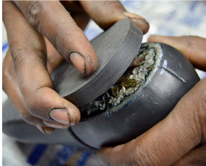
Sole being glued to the lasted upper
