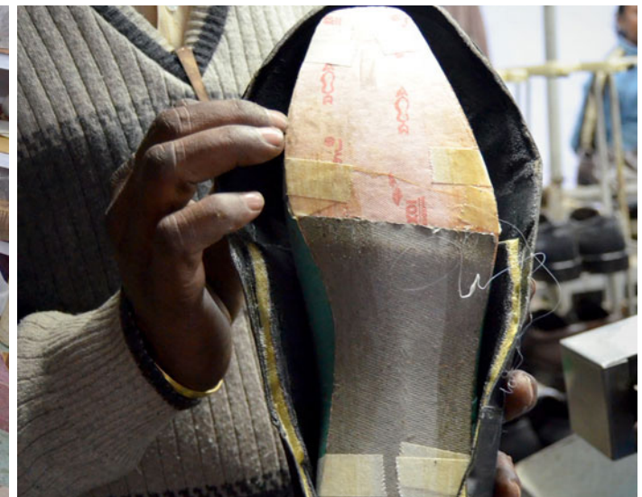
Insole attached to the bottom of the last
