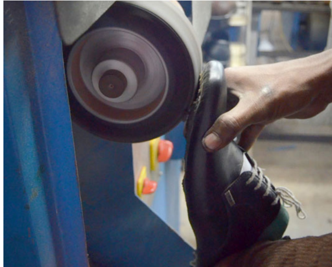
The base of the lasted upper being rubbed off
