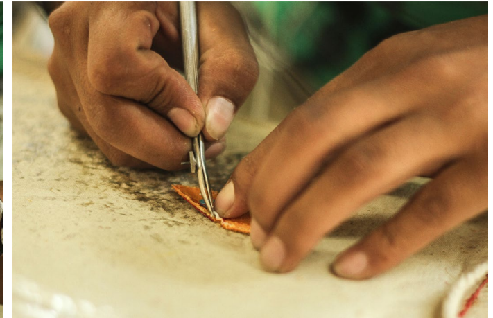
Cut edge is folded backward with a divider and pasted with using adhesive.
