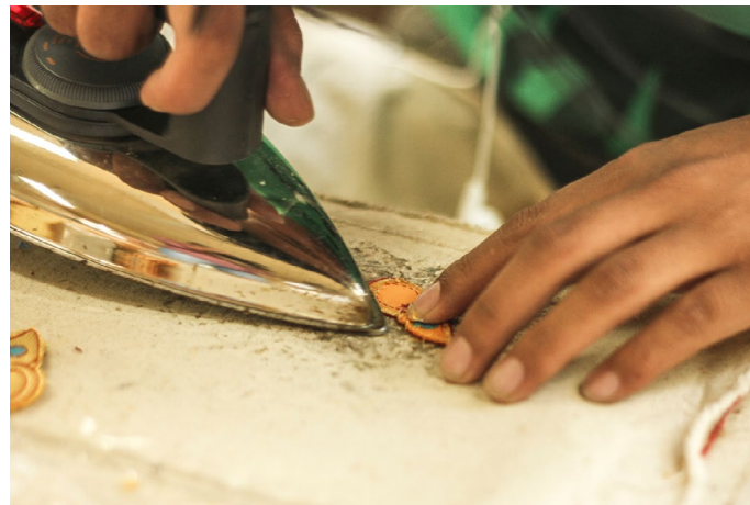
Glued edges are ironed to get a fine finishing.
