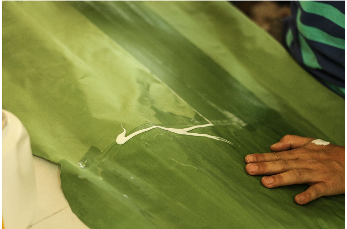
Synthetic adhesive is applied (spread) on the fabric to make it stiff.
