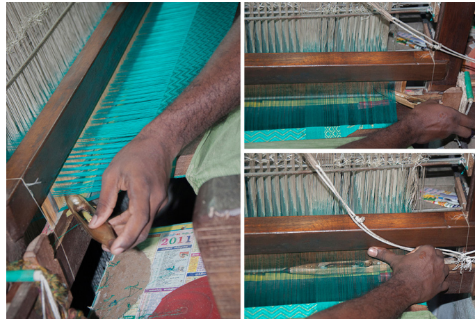
Moving Flying shuttle to and fro.
