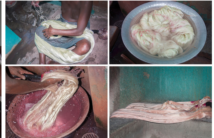
Soaking yarn and washing with plain water to dye the yarn.
