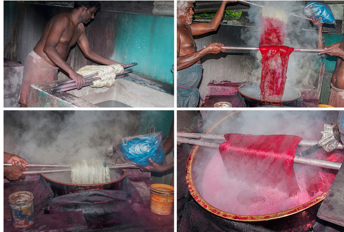
Placing washed yarn with the help of metal rods.
