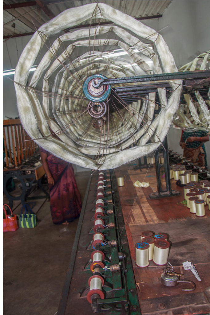
Reeling threads from the Winding Creels to the spindles.
