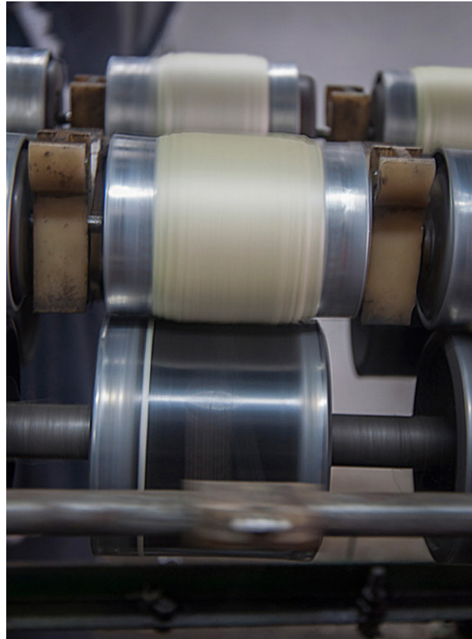
Winding machine – twisting two threads into single thread.
