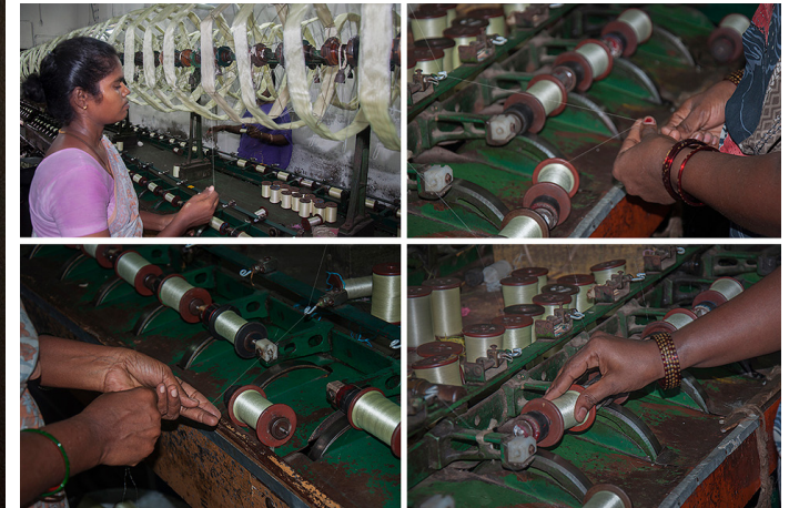
Joining thread from the machine to the spindle by twisting.
