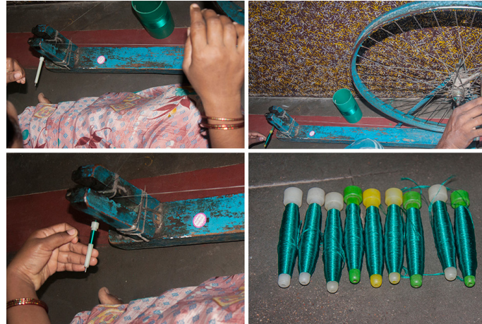
Winding threads to the pirns according to the colour combination of the saree.
