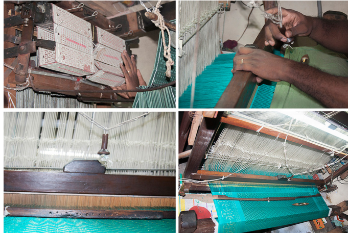
Weaver starts weaving by arranging the Jacquard machine punch cards according to the designs.
