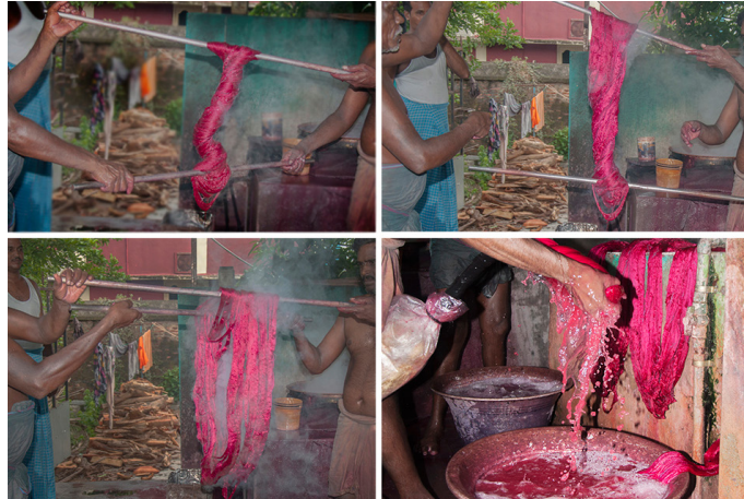
Dyed silk yarn is removed from the container and washing with normal water.
