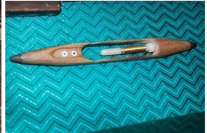
Flying Shuttle - that carries the thread across the loom left yarn while weaving.
