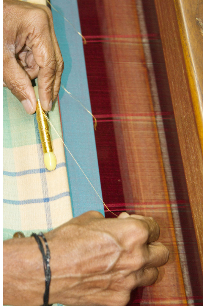
Zari threads are inserted for the buta design in the process of silk saree weaving.
