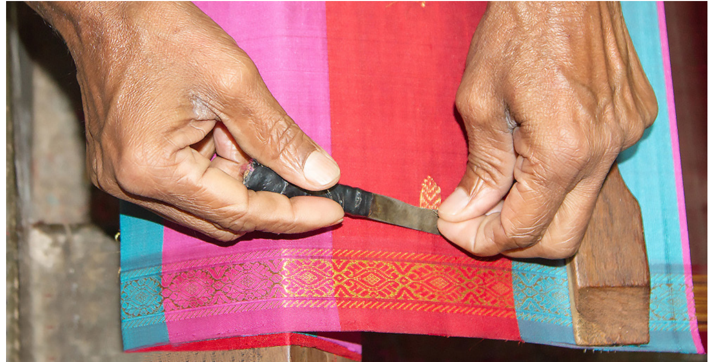
The extras of zari threads are removed through the help of knife.
