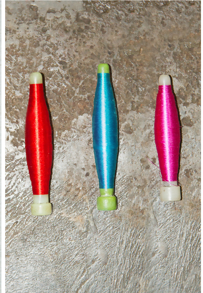
Different colored silk yarn are spun onto the pirns.
