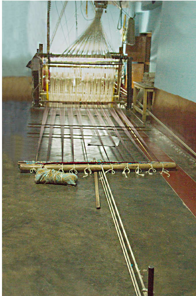
The loom, used in Melukote for silk saree weaving.
