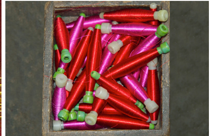
Pirns spun with colored silk threads, used for weaving.
