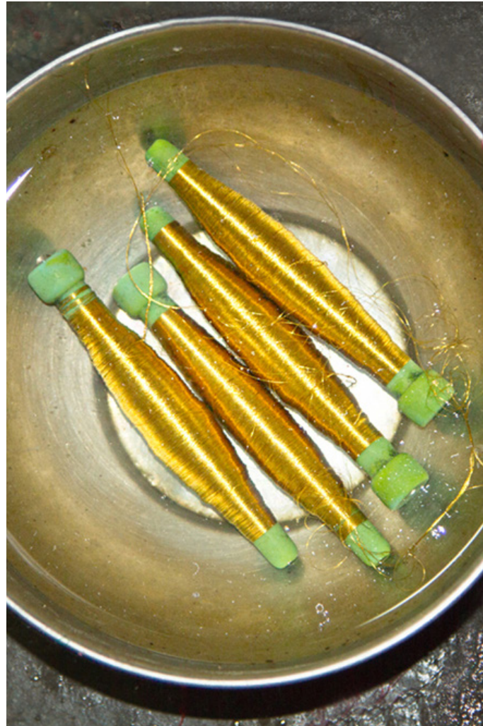
The Zari which is spun to the pin is soaked in water before putting it to the fly shuttle.
