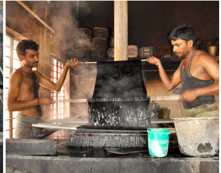
Two artisans work together to rotate/roll the yarns systematically so that the color spreads evenly.
