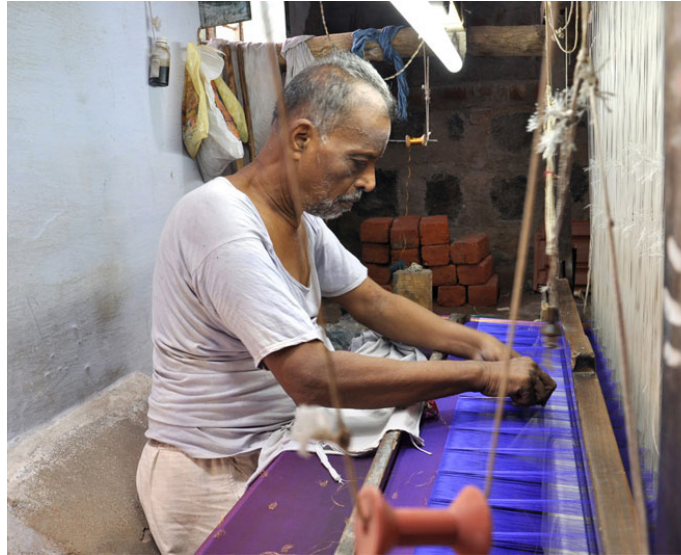
Silk sarees are woven on a raised pit loom.
