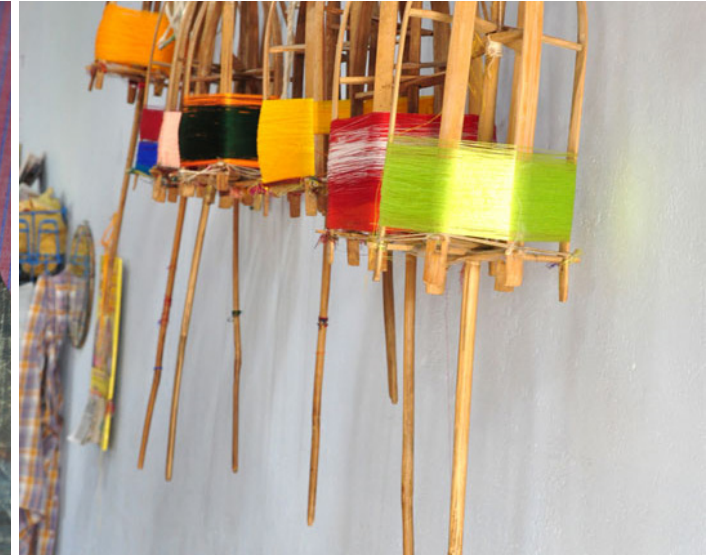
Thiravattam: used for winding yarns .
