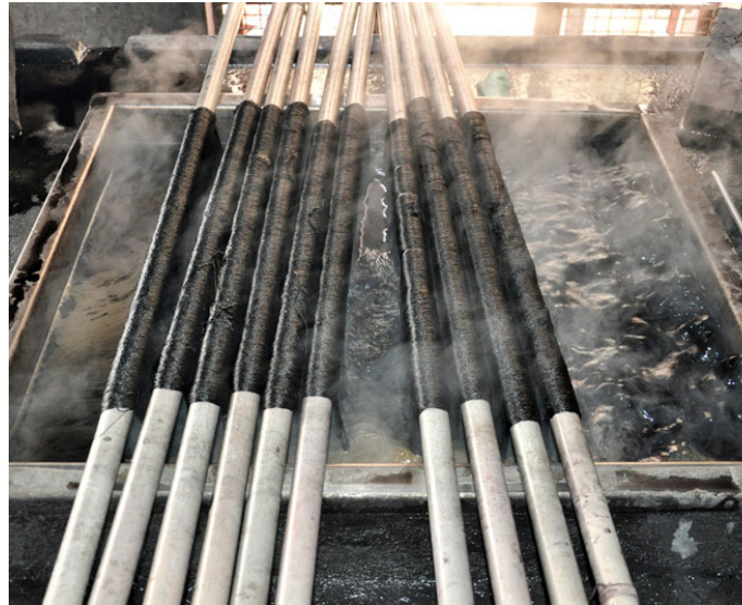
The bundle of yarn are hanged/ hung from the metal rod and dipped in a tank with boiling water and color.
