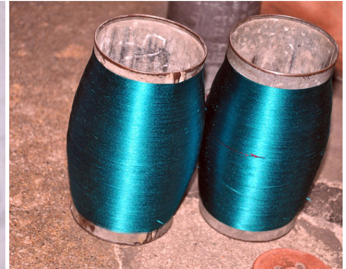
Yarn are winded/ coiled on the bobbin.
