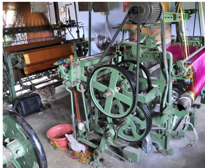
Sometimes jacquards is also used to carry out production or to make complex designs.
