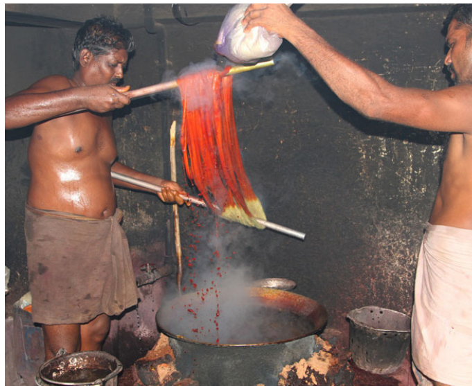
The yarn is hanged between two iron rods to rotate continuously while coloring.
