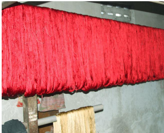
Colored yarn dried at room temperature.
