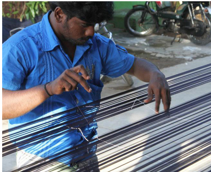
Warp is stretched over bamboo stick to inspect breaks in the silk threads.
