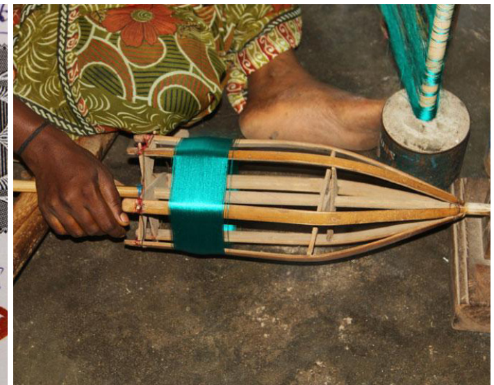
Parivattam - Bamboo spool used to wind the yarn to form silk bundles.
