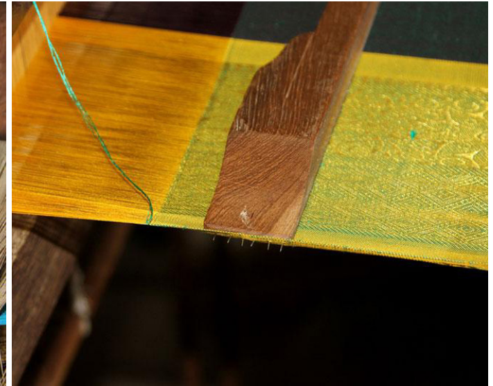
A wooden stick fixed to the woven part of sari for better support.
