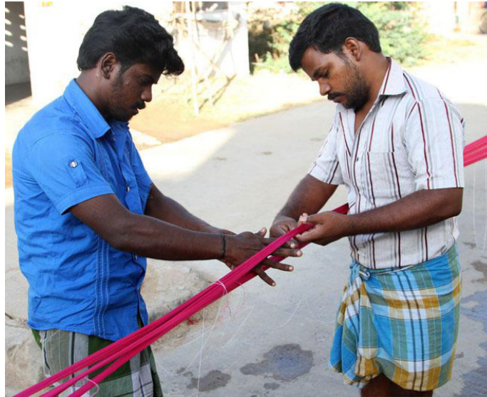
Artisan making space to insert bamboo stick.
