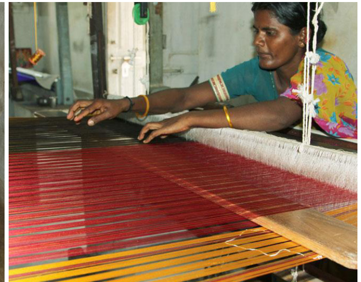
Weaver inspecting warp to ensure smooth weaving.
