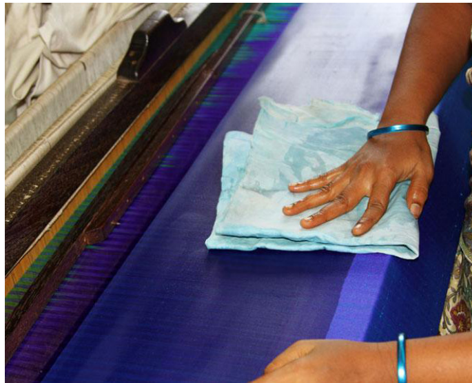
Excess gum is removed.
