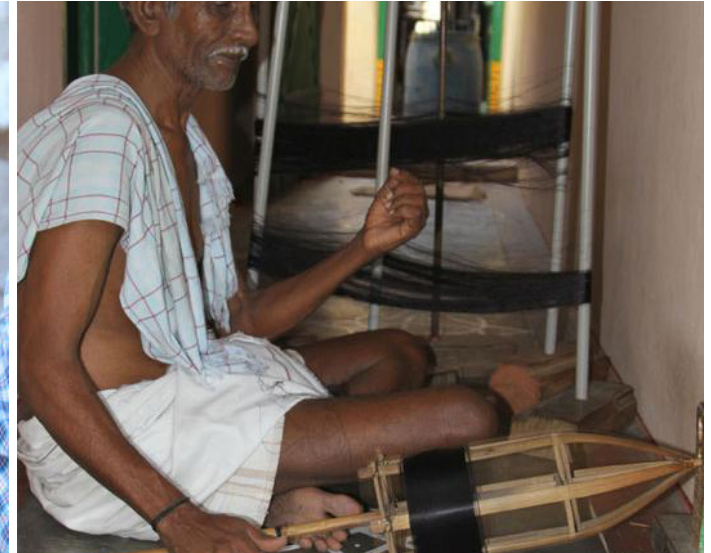
Silk bundle is reeled onto traditional bamboo spool.
