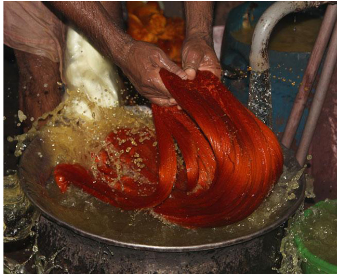
The dyed color is washed in normal water.
