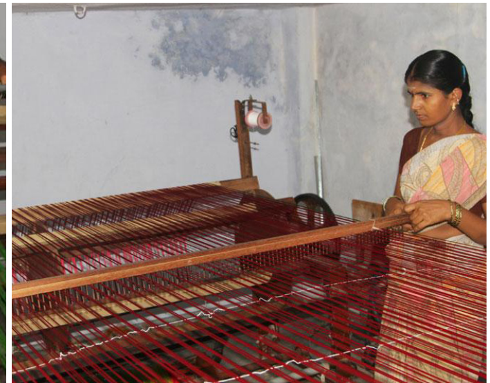
Reed is inserted into warp threads to make them even.
