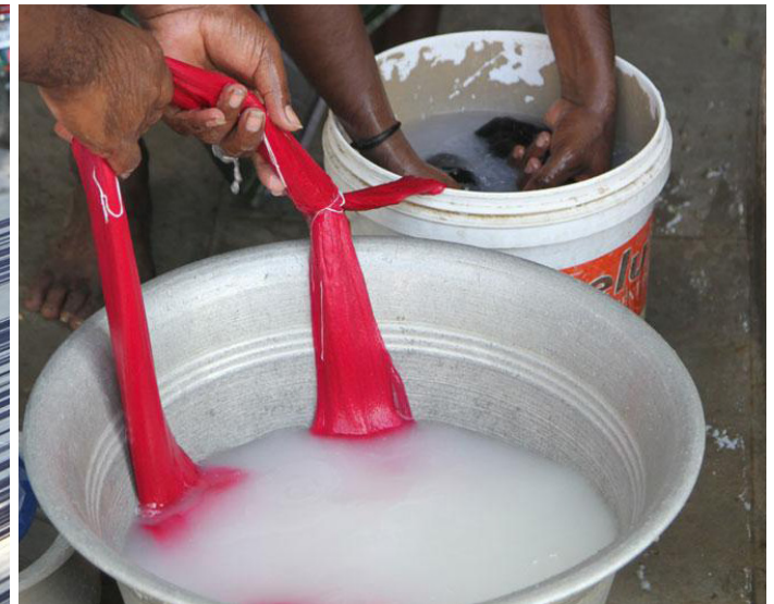
After warping, the silk is dipped in rice starch.
