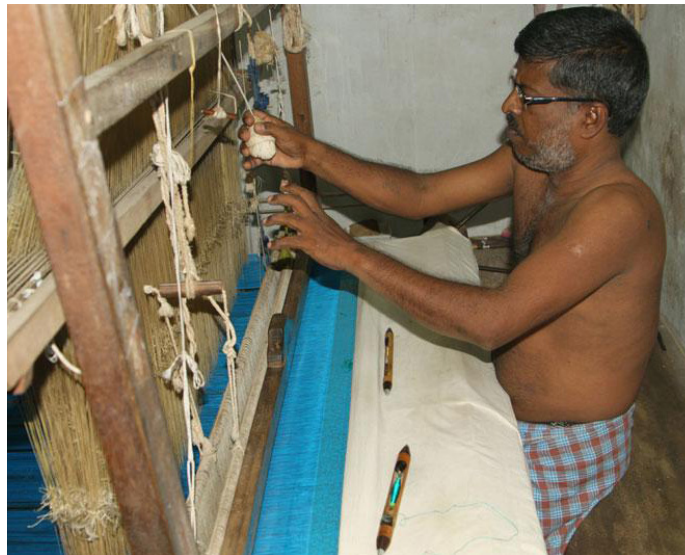
Pulley helps to lift the warp threads.
