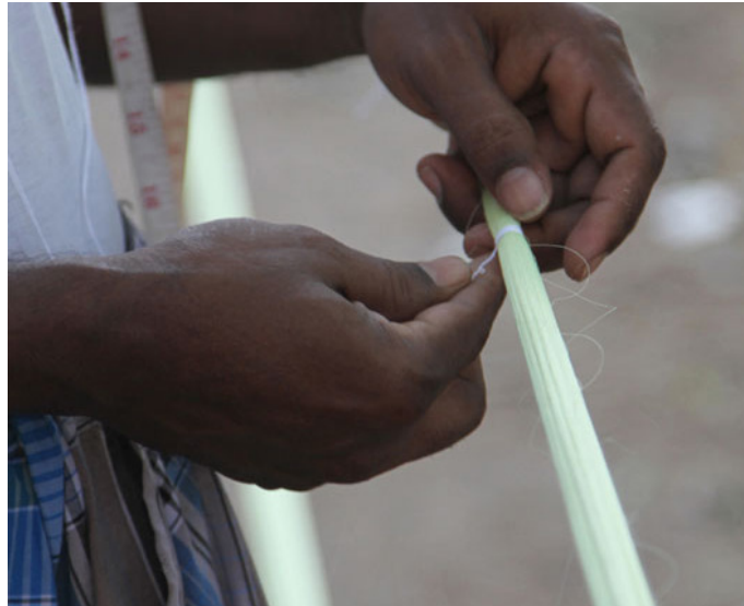
The warp is measured with tape and knotted with cotton thread.
