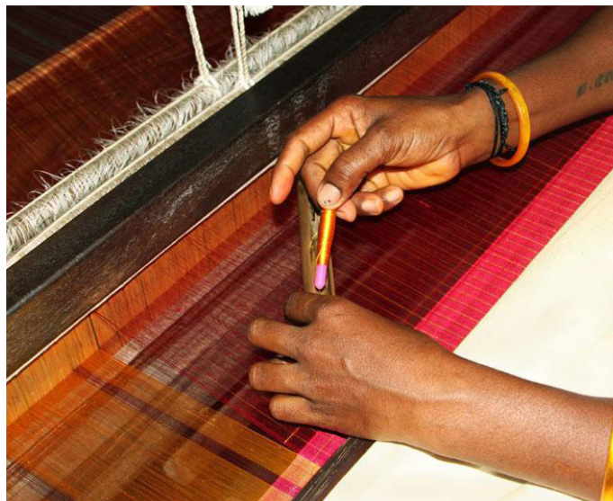
Spindle is being inserted into fly-shuttle.
