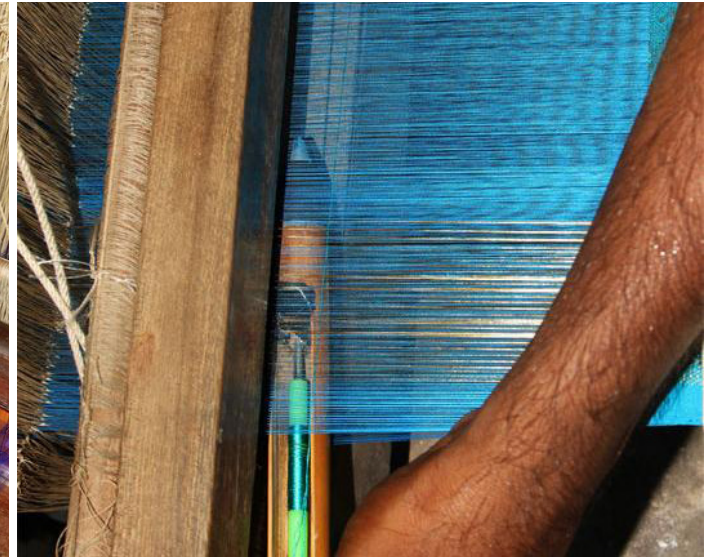
The shuttle is collected from other end.
