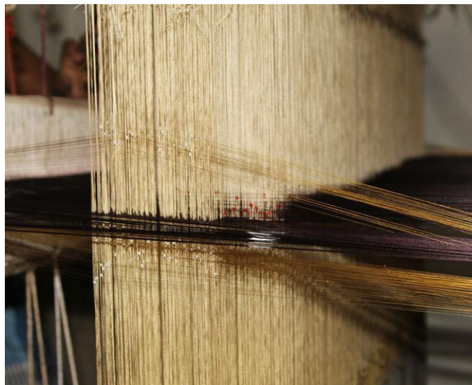
Zari-golden thread loaded in warp for borders.
