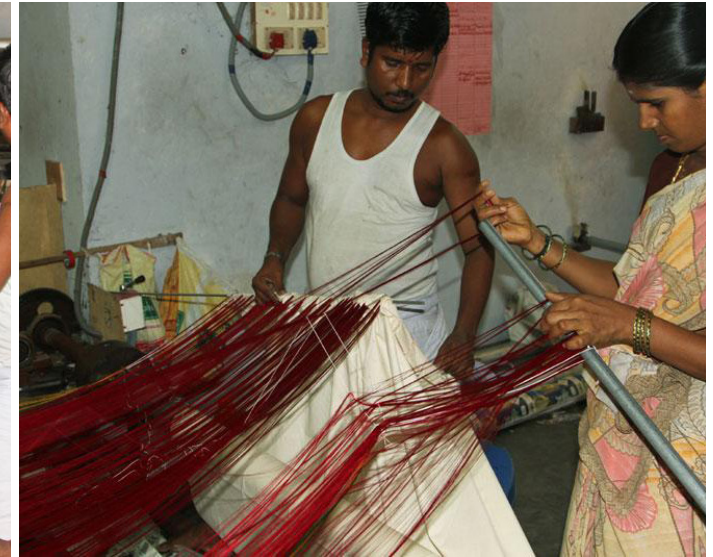
The ends are connected to iron rod to make warp beam.
