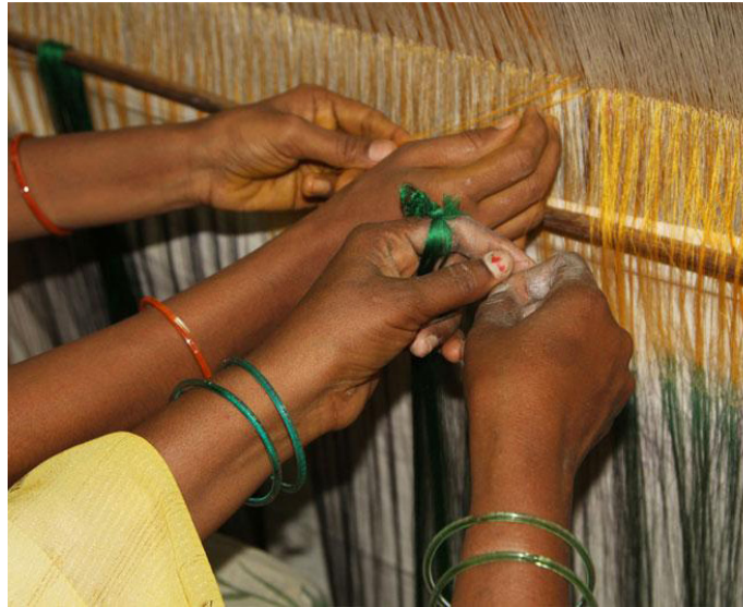
Each thread from warp beam is being attached to the loom silk threads.
