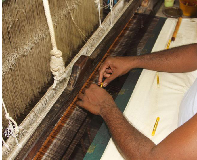
External Zari thread is inserted to create motif designs.
