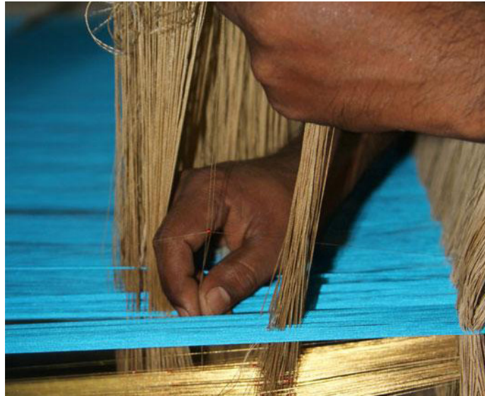
Small beads are inserted to connect warp threads and jacquard threads.
