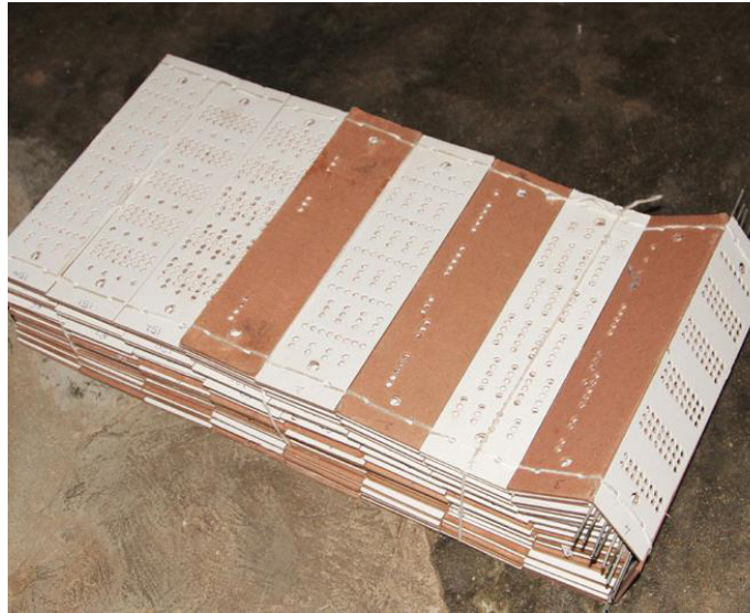
Punch cards are loaded into Jacquard for getting design in the sari.
