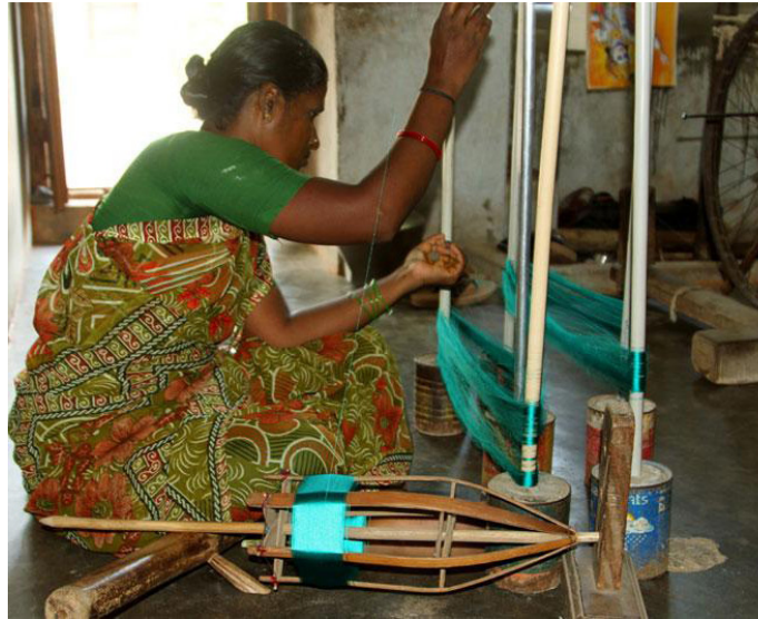
Entangles and breaks are cleared in spinning process.
