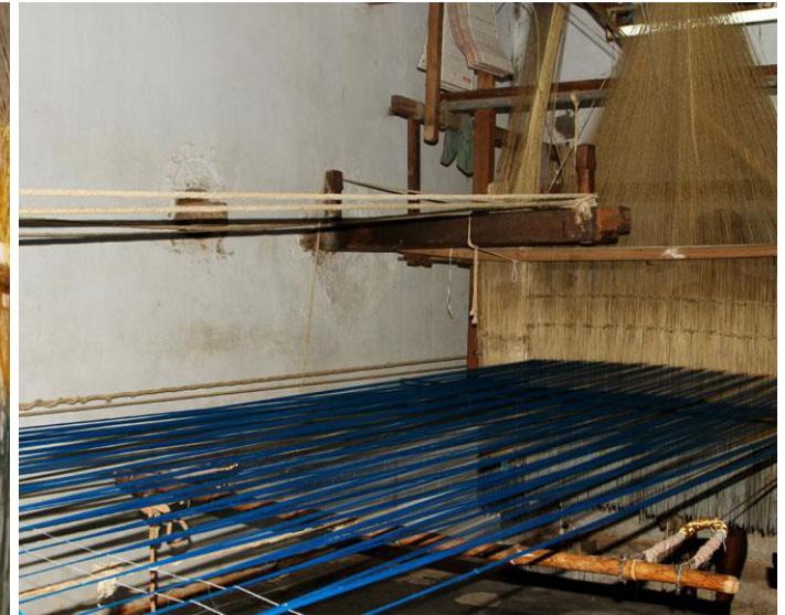
In Kanchipuram, Count of warp threads ranges from 5000 to 6000.
