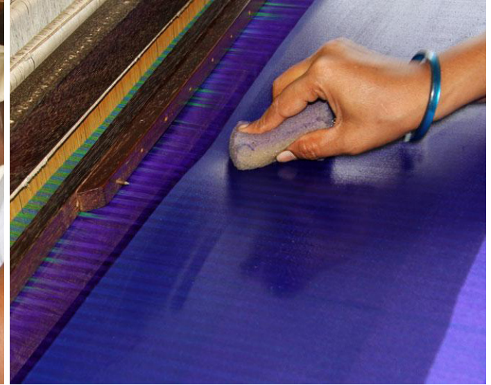
Gum is applied on the sari for stiffness.
