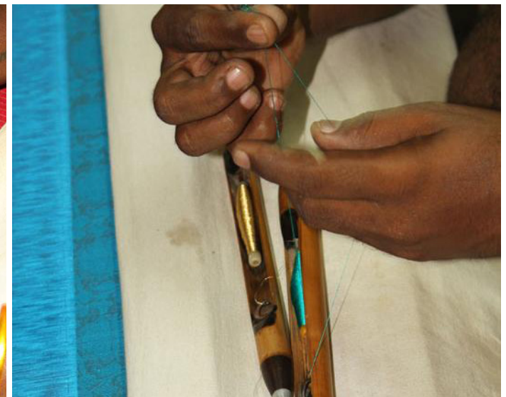
The thread of fly-shuttle is connected to warp threads.
