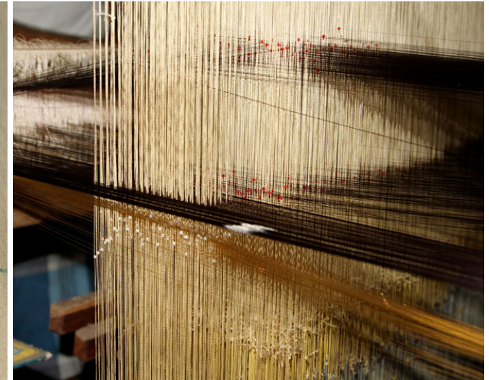
Synthetic threads to connect jacquard and warp threads.
