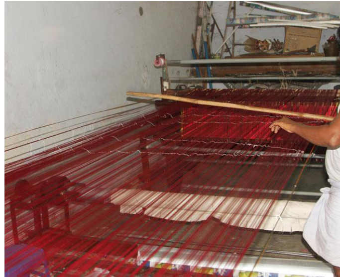
Artisan checking the tautness between the stretched warp.
