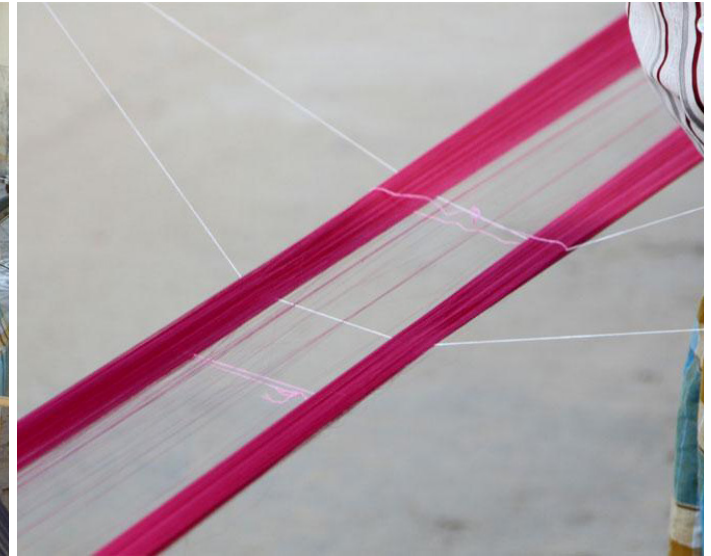
Cotton thread is inserted into warp threads as it helps to find the damaged silk threads.
