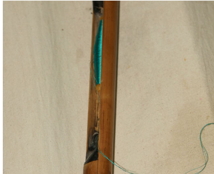
Spindle –Kulal is inserted into Fly-shuttle- Neelalocally.
