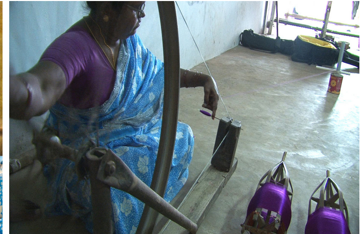
The yarn is wound into pirns from parivattam with the help of Charkha.
