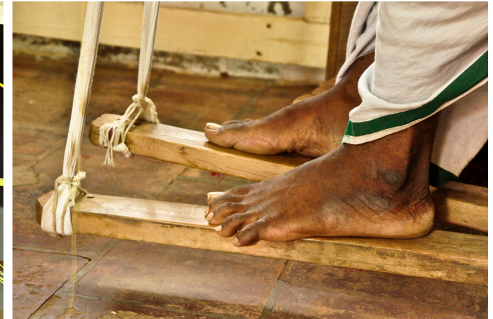
Foot pedals are used to control the insertion of the pattern of designs.
