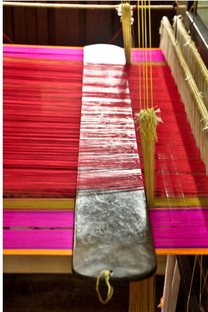
Another plank is inserted horizontally between the warp threads to prevent from tangling.
