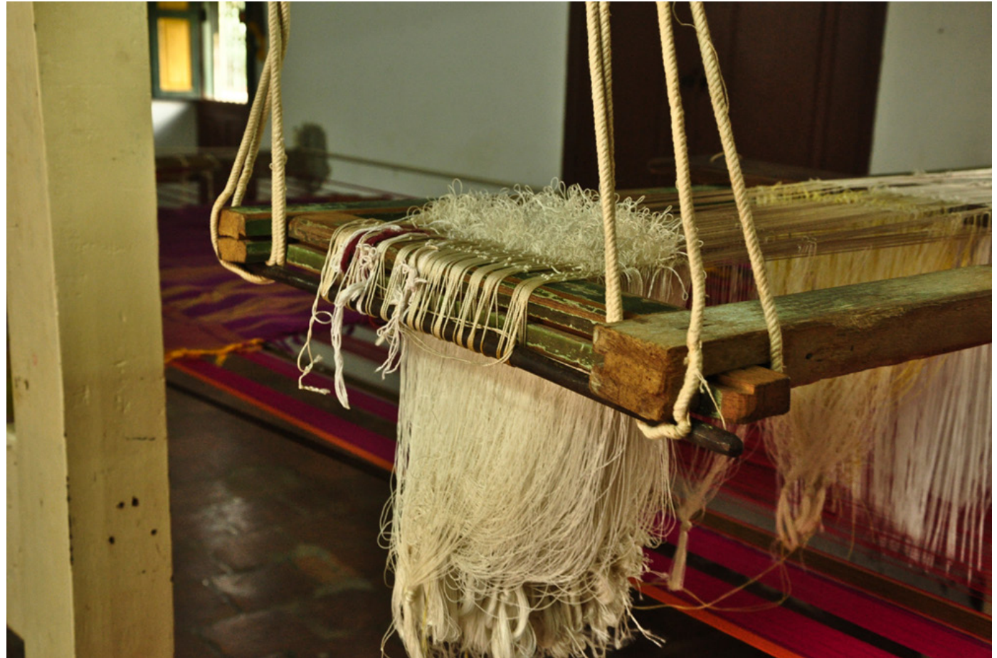
Adai attachments are used for the insertion of the design pattern.
