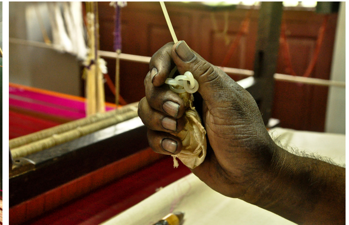
The hand holder is pulled to keep changing the punch cards in the Jacquard to form the designs.
