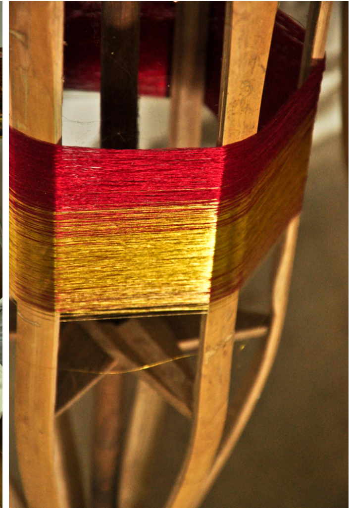
Two or more colors of silk threads are wound on the parti to weave multicolor saree.
