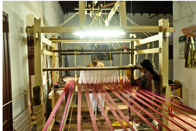
Looms with adai are used to weave the silk saree.
