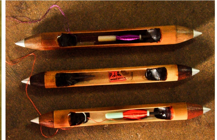
Fly shuttle is used for the weft insertion while weaving.
