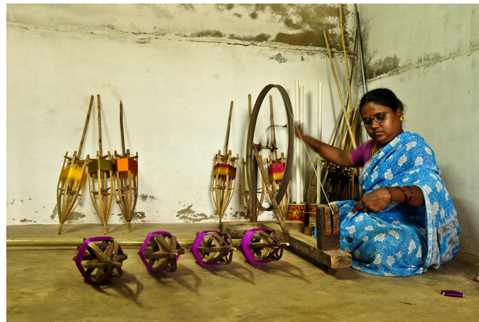
These spindles are used in fly shuttle while weaving.
