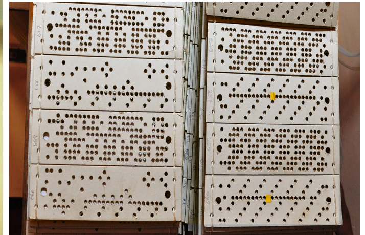
Punch cards are used to insert the pattern of design.
