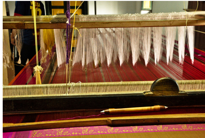
Fly-shuttle is used to interlock the weave. (Adai attachments are fixed to the loom for design insertions)
