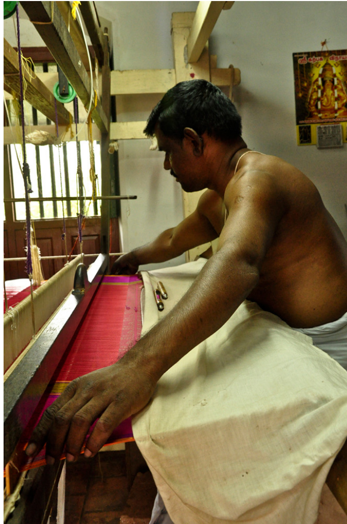
The weaver arranges the thread and loom for weaving.
