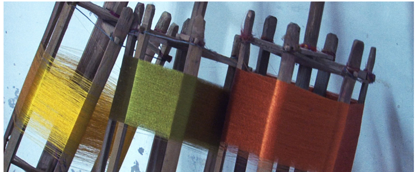
Swift (parivattam) is used to spin the silk yarn.
