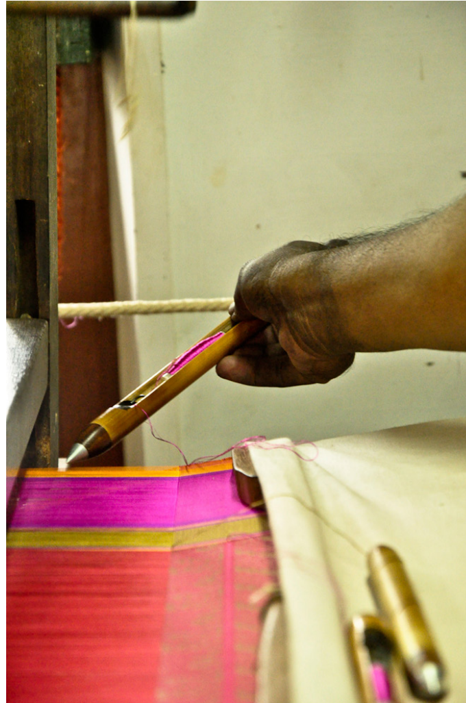
Shuttle with weft color thread is used while weaving, which interlocks the weave.
