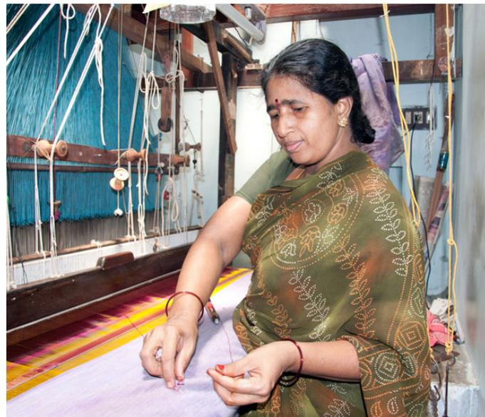
Joining the silk thread from fly shuttle to the loom thread.
