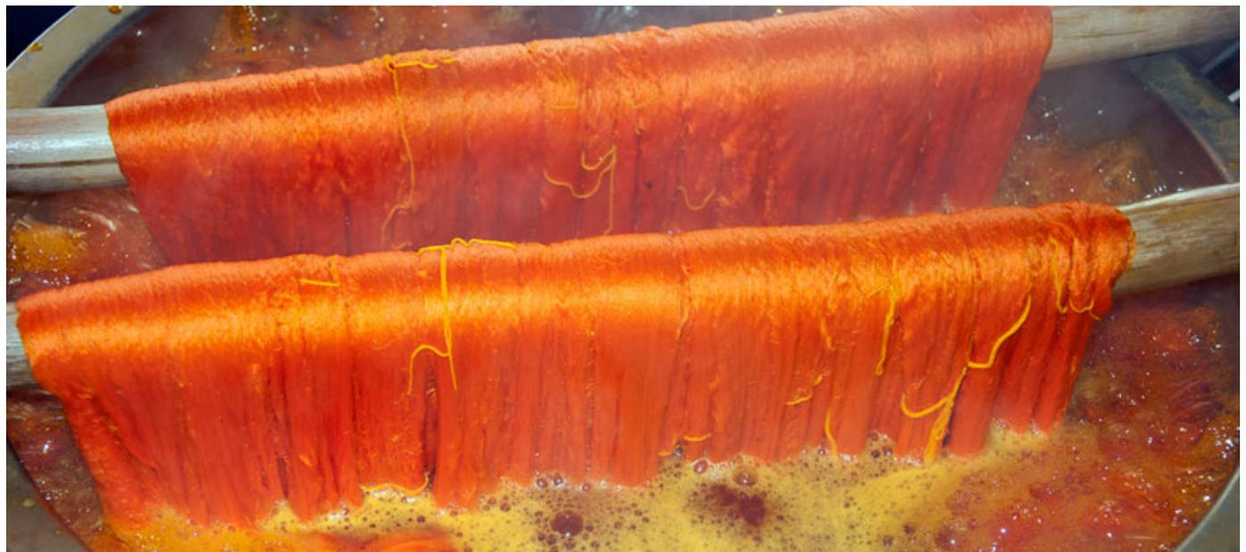
The silk yarn kept for boiling continuously for 30 min.
