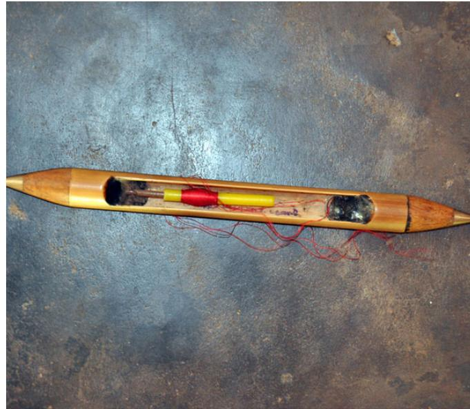
Fly shuttle made of bamboo.
