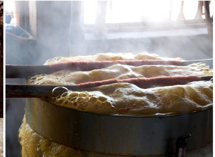
The yarn is immersed in dye solution.
