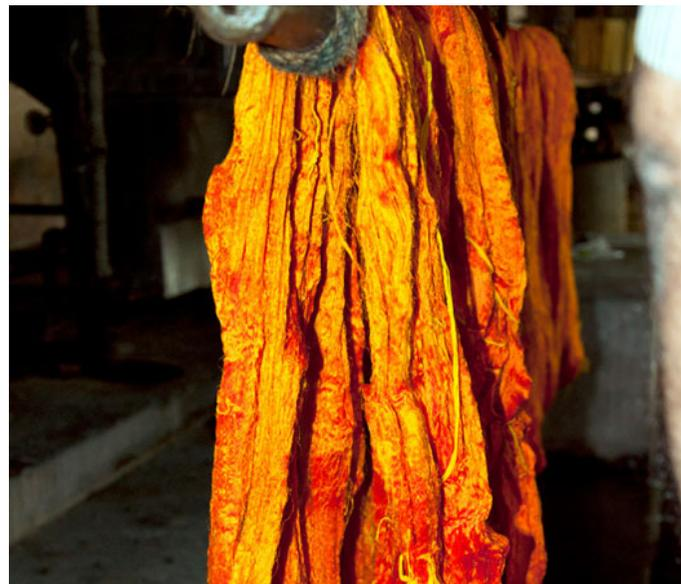
The yarn is hung on a bamboo stick and allowed to dry under shade.
