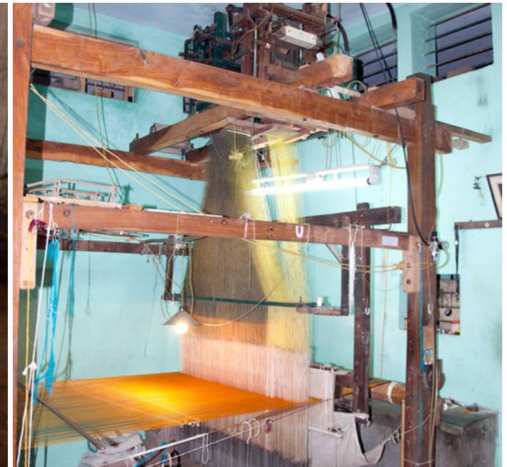
Arrangement of loom with jacquard machines at the top.
